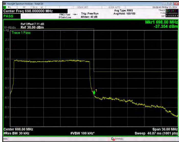
Band71 QPSK BW=20MHz Channel=133222 RB Size=1 Position=#0
