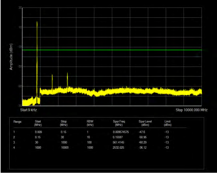
Band5 QPSK BW=3MHz Channel=20415 RB Size=15 Position=#0
