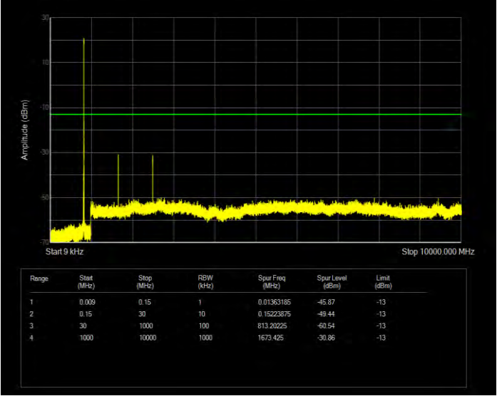
Band5 16QAM BW=1.4MHz Channel=20643 RB Size=6 Position=#0
