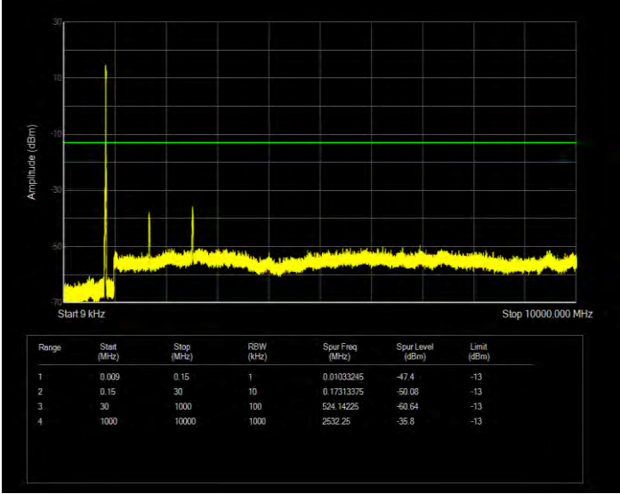
Band5 16QAM BW=3MHz Channel=20415 RB Size=15 Position=#0
