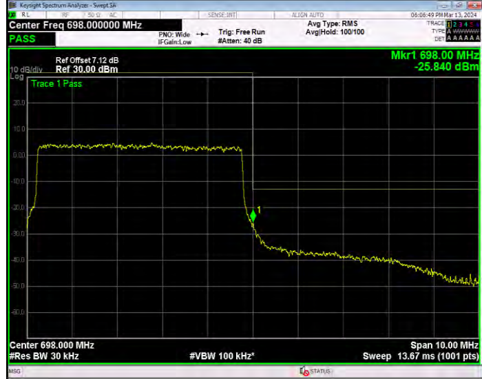
Band71 QPSK BW=5MHz Channel=133447 RB Size=25 Position=#0
