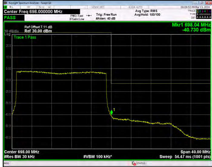
Band71 QPSK BW=5MHz Channel=133147 RB Size=1 Position=#0
