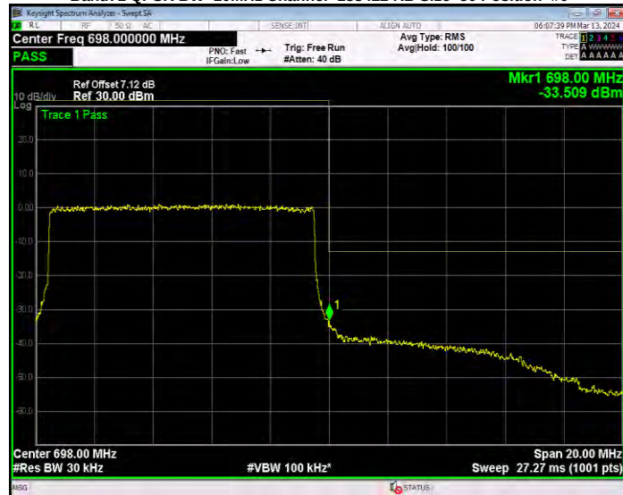
Band71 QPSK BW=15MHz Channel=133197 RB Size=1 Position=#0
