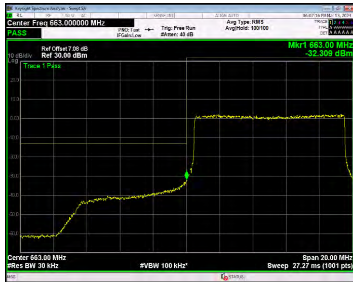
Band71 QPSK BW=10MHz Channel=133422 RB Size=1 Position=#0
