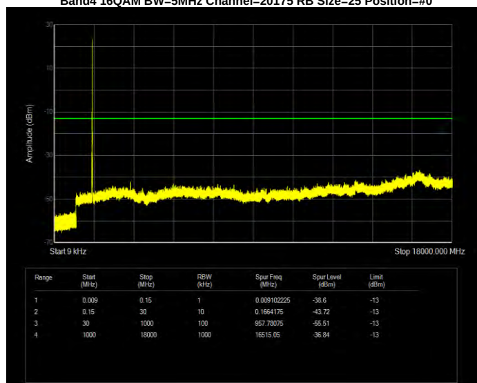
Band4 16QAM BW=5MHz Channel=20375 RB Size=25 Position=#0
