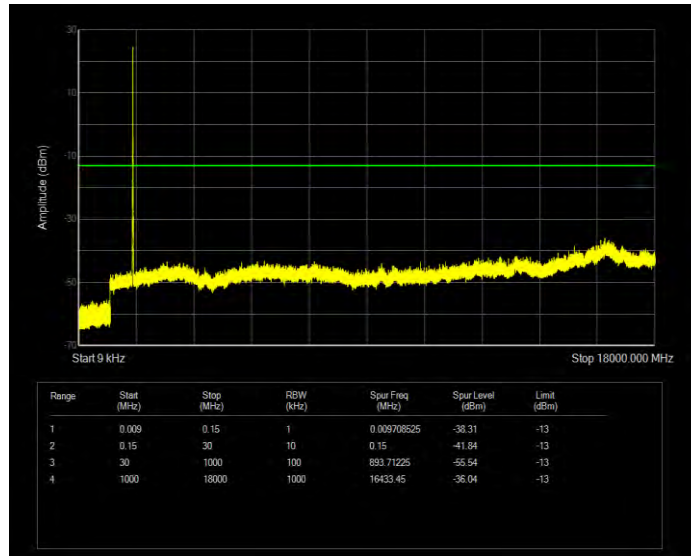
Band4 QPSK BW=5MHz Channel=20175 RB Size=25 Position=#0
