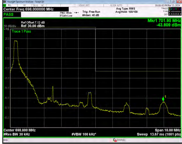
Band71 QPSK BW=5MHz Channel=133447 RB Size=25 Position=#0
