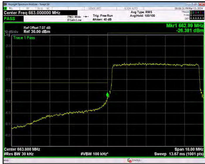
Band71 QPSK BW=5MHz Channel=133447 RB Size=1 Position=#0
