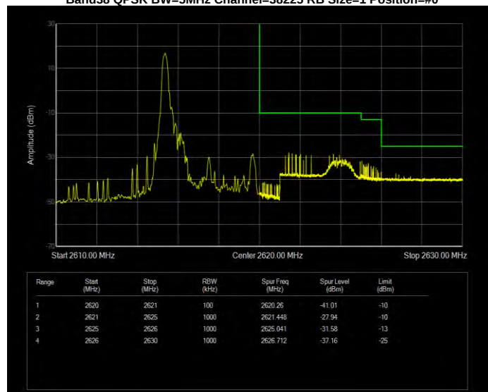
Band38 QPSK BW=5MHz Channel=38225 RB Size=25 Position=#0
