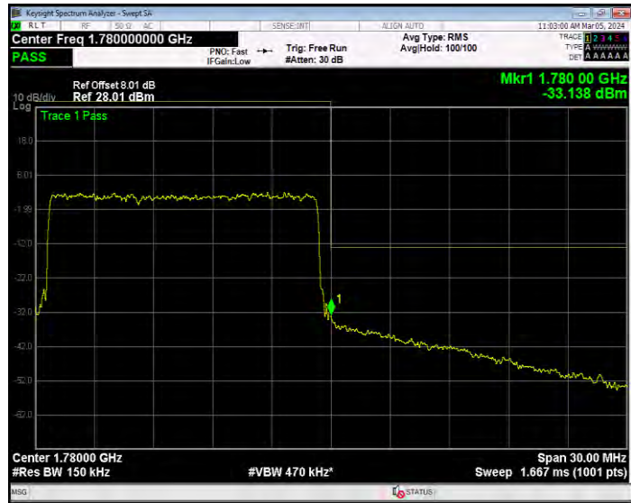
Band66 QPSK BW=20MHz Channel=132072 RB Size=1 Position=#0
