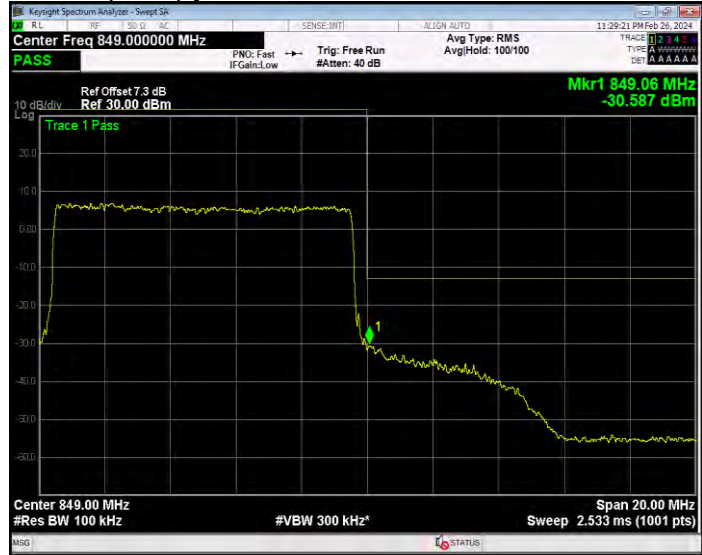
Band26(824-849) QPSK BW=15MHz Channel=26865 RB Size=75 Position=#0
