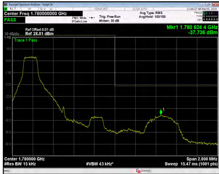
Band66 QPSK BW=1.4MHz Channel=132665 RB Size=6 Position=#0
