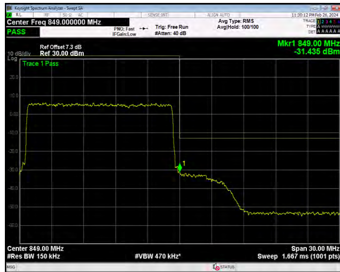
Band26(824-849) QPSK BW=3MHz Channel=26805 RB Size=15 Position=#0
