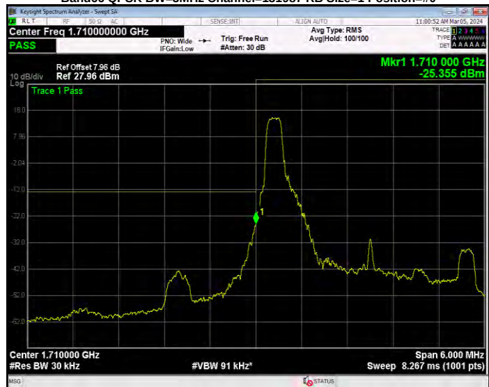
Band66 QPSK BW=3MHz Channel=131987 RB Size=15 Position=#0
