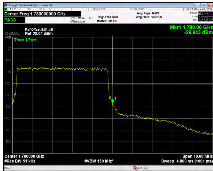
Band66 QPSK BW=1.4MHz Channel=131979 RB Size=1 Position=#0
