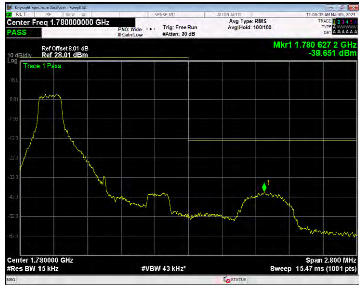
Band66 16QAM BW=1.4MHz Channel=132665 RB Size=6 Position=#0
