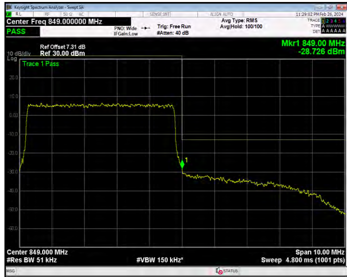
Band26(824-849) QPSK BW=1.4MHz Channel=26797 RB Size=6 Position=#0
