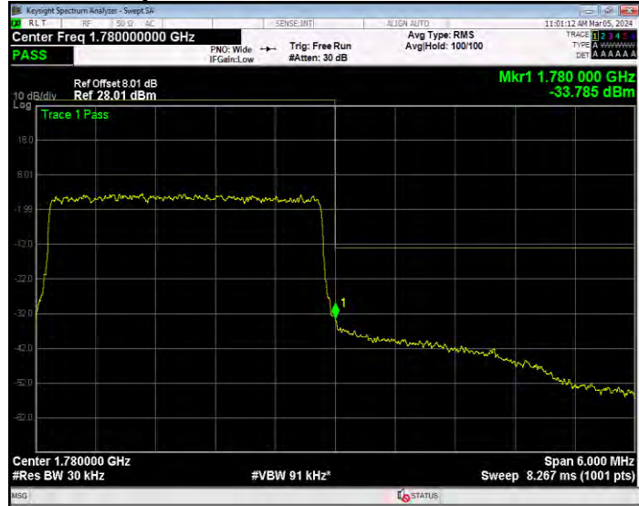
Band66 QPSK BW=5MHz Channel=131997 RB Size=1 Position=#0
