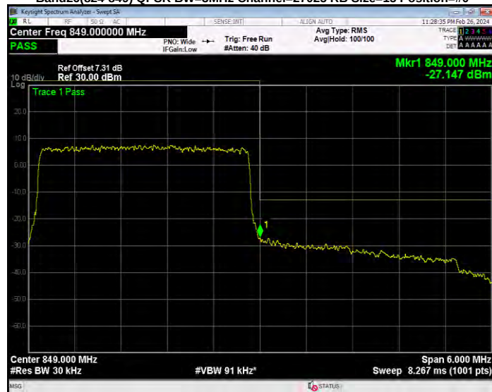
Band26(824-849) QPSK BW=5MHz Channel=26815 RB Size=25 Position=#0
