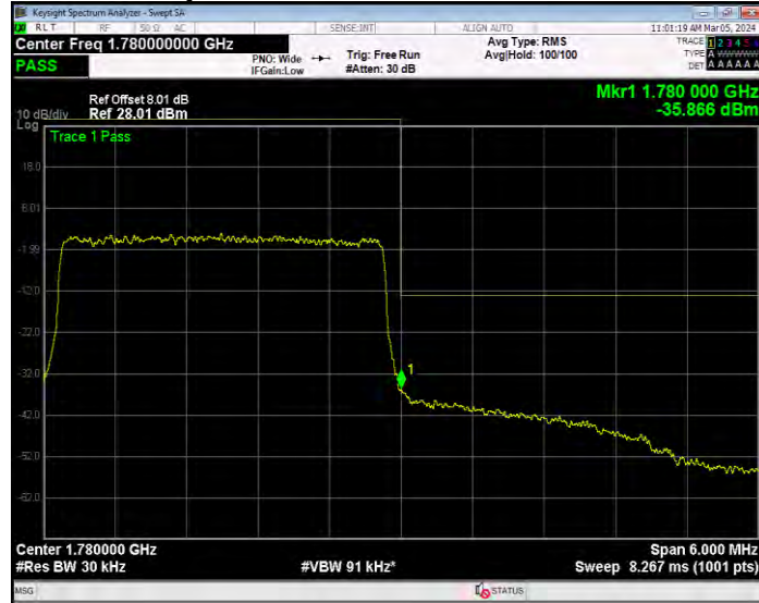
Band66 16QAM BW=5MHz Channel=131997 RB Size=1 Position=#0
