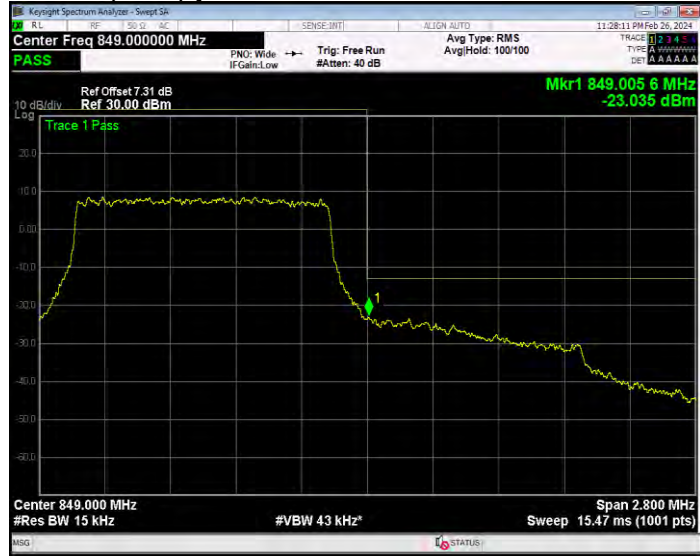
Band26(824-849) QPSK BW=10MHz Channel=26840 RB Size=50 Position=#0
