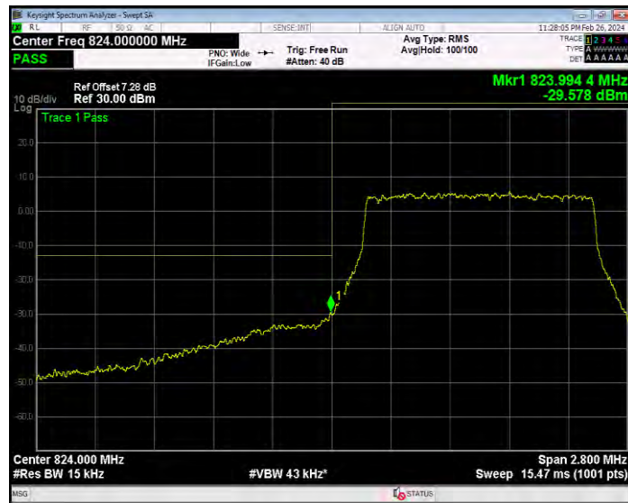
Band26(824-849) 16QAM BW=1.4MHz Channel=27033 RB Size=6 Position=#0
