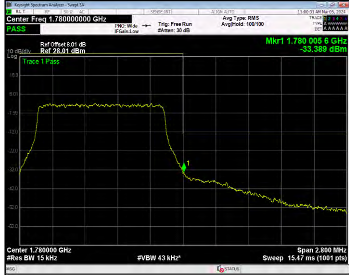
Band66 QPSK BW=10MHz Channel=132022 RB Size=1 Position=#0
