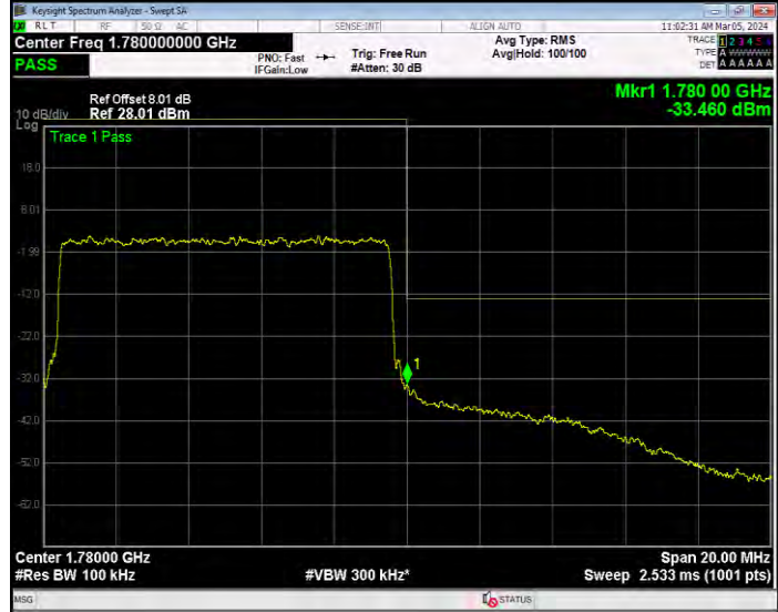
Band66 16QAM BW=15MHz Channel=132047 RB Size=1 Position=#0
