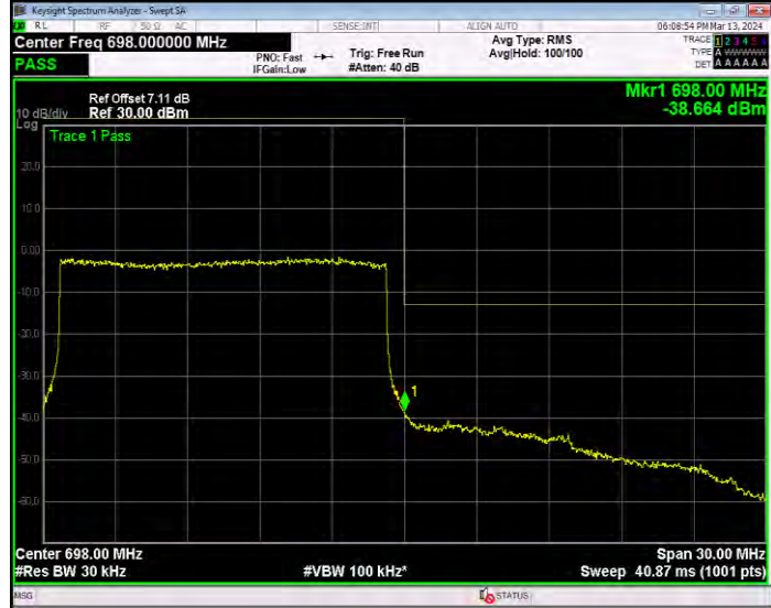
Band71 16QAM BW=20MHz Channel=133222 RB Size=1 Position=#0
