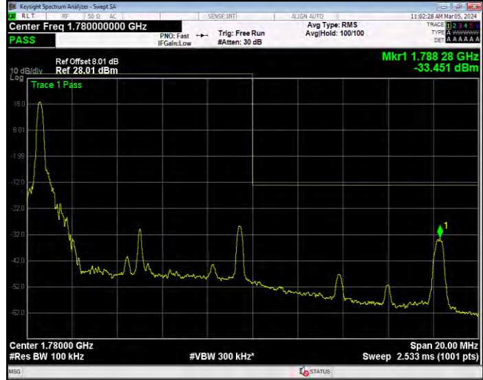
Band66 16QAM BW=10MHz Channel=132622 RB Size=50 Position=#0
