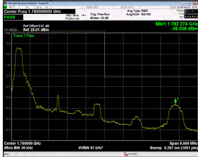
Band66 16QAM BW=3MHz Channel=132657 RB Size=15 Position=#0
