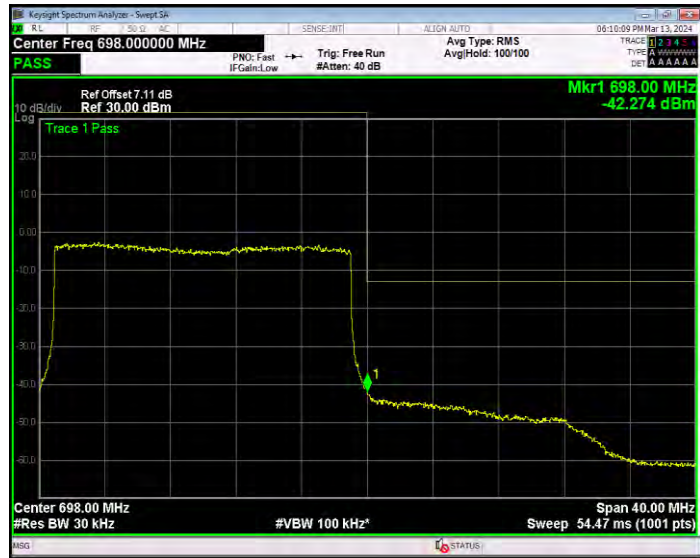
Band71 16QAM BW=5MHz Channel=133147 RB Size=1 Position=#0
