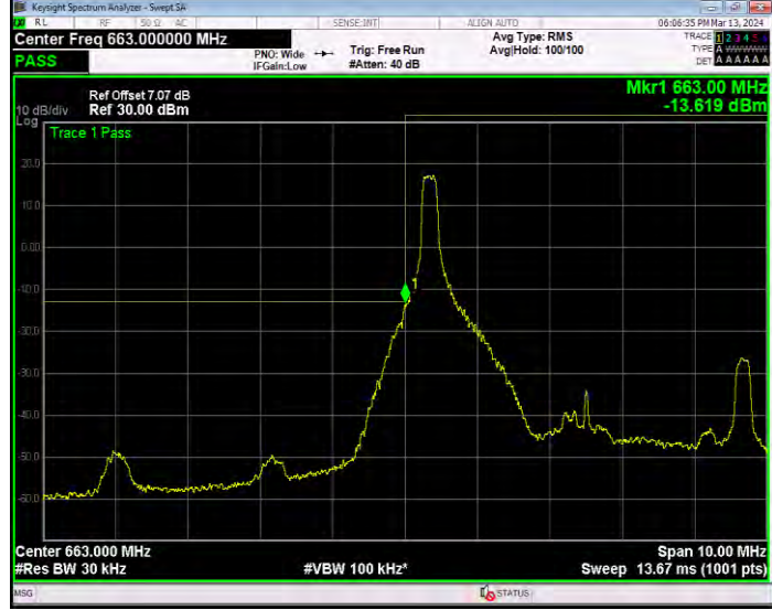
Band71 16QAM BW=5MHz Channel=133147 RB Size=25 Position=#0
