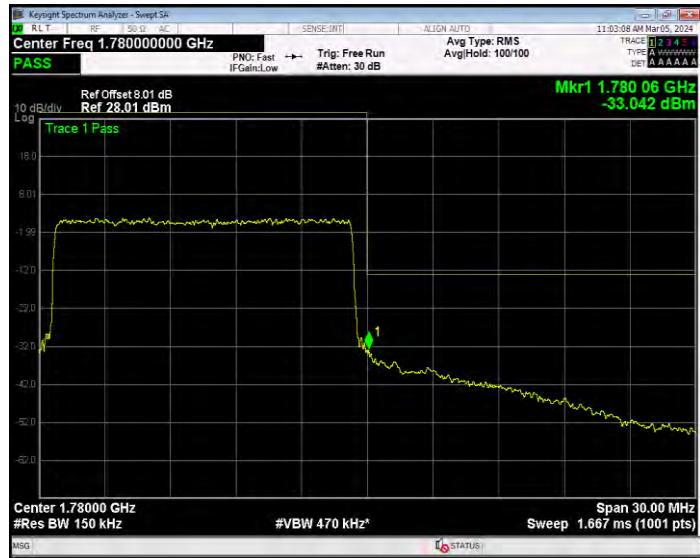
Band66 16QAM BW=20MHz Channel=132072 RB Size=1 Position=#0
