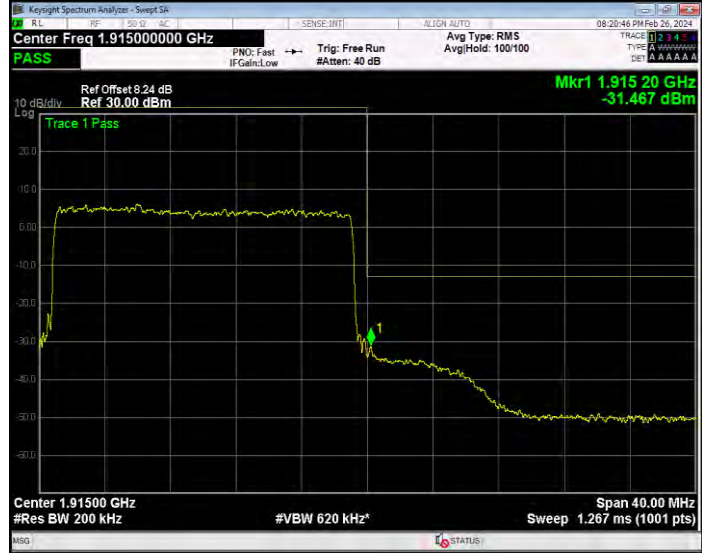
Band25 QPSK BW=3MHz Channel=26055 RB Size=15 Position=#0
