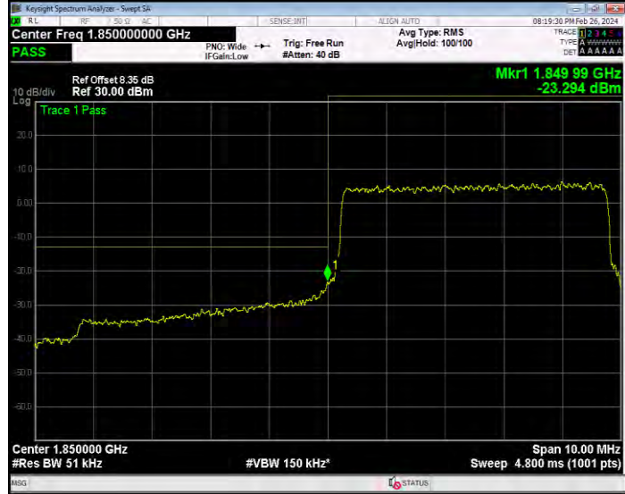
Band25 QPSK BW=5MHz Channel=26665 RB Size=25 Position=#0
