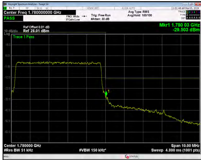
Band71 16QAM BW=10MHz Channel=133172 RB Size=1 Position=#0
