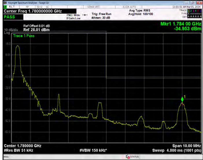
Band66 16QAM BW=5MHz Channel=132647 RB Size=25 Position=#0
