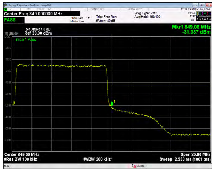
Band26(824-849) 16QAM BW=15MHz Channel=26865 RB Size=75 Position=#0
