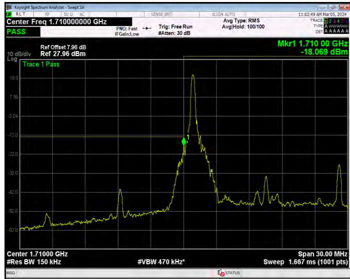
Band66 16QAM BW=15MHz Channel=132047 RB Size=75 Position=#0
