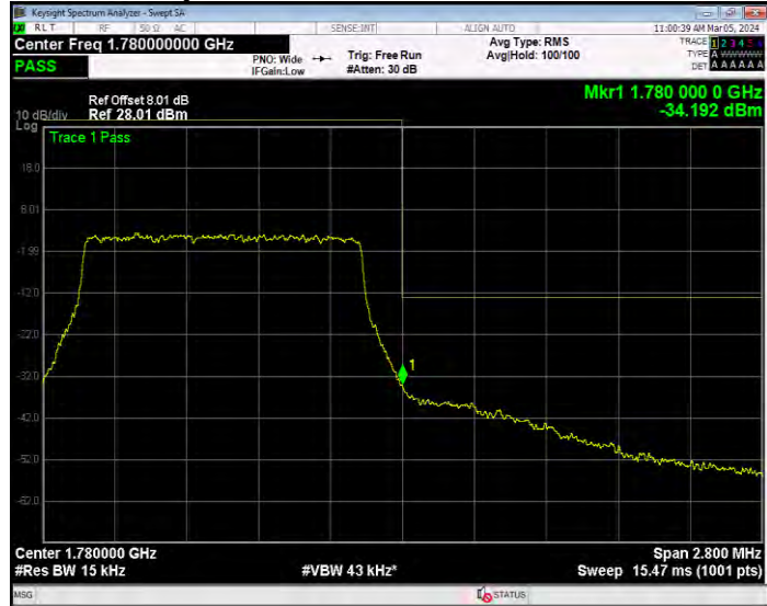
Band66 16QAM BW=10MHz Channel=132022 RB Size=1 Position=#0
