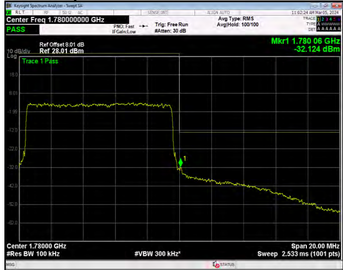
Band66 QPSK BW=15MHz Channel=132047 RB Size=1 Position=#0
