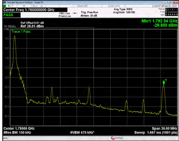
Band66 QPSK BW=15MHz Channel=132597 RB Size=75 Position=#0
