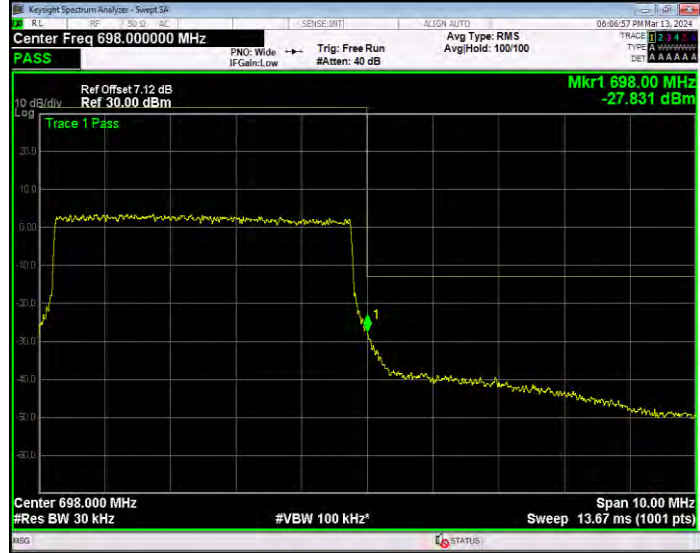
Band71 QPSK BW=10MHz Channel=133172 RB Size=1 Position=#0
