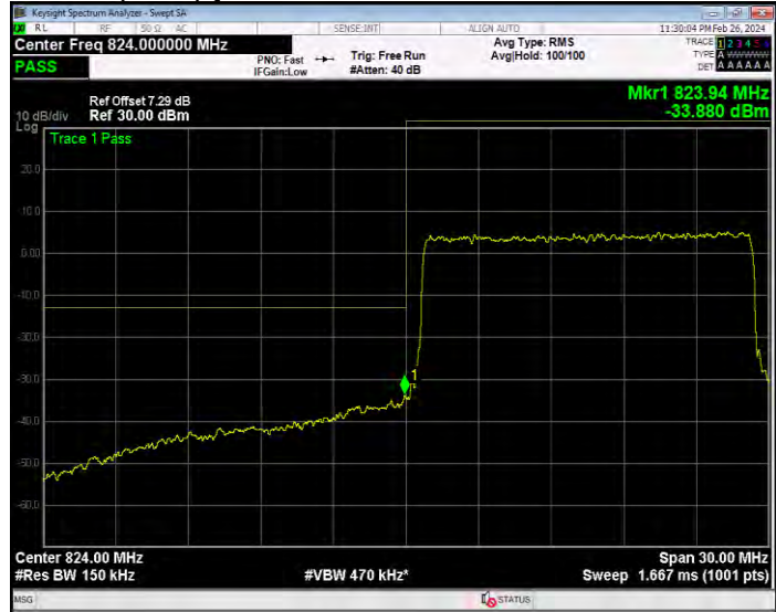
Band26(824-849) QPSK BW=15MHz Channel=26965 RB Size=75 Position=#0
