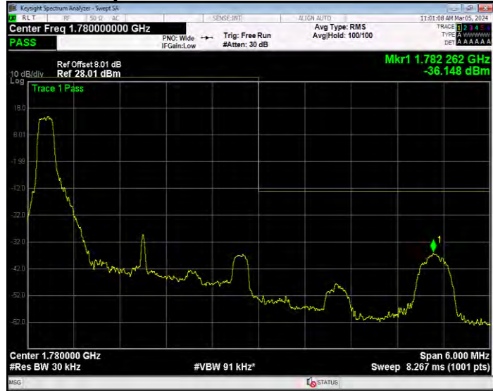
Band66 QPSK BW=3MHz Channel=132657 RB Size=15 Position=#0
