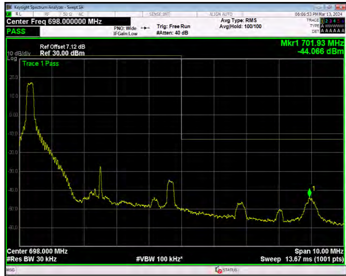
Band71 16QAM BW=5MHz Channel=133447 RB Size=25 Position=#0
