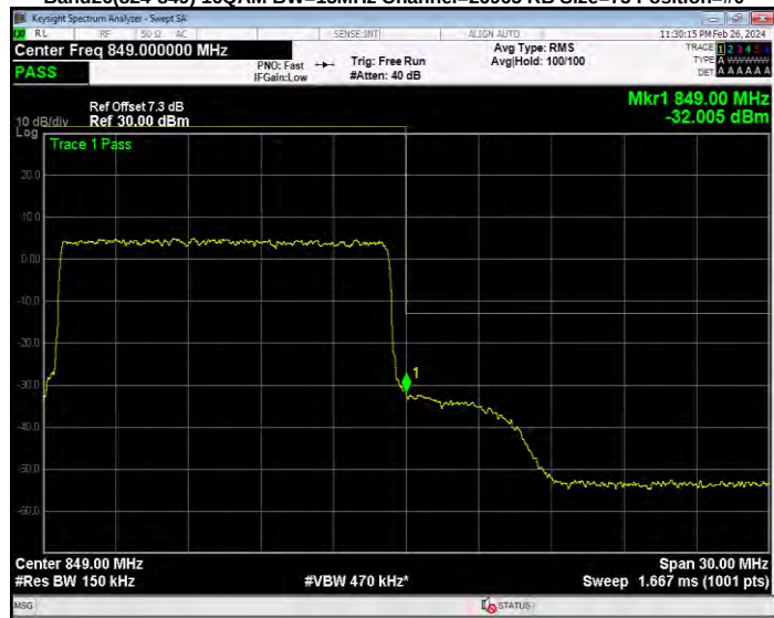
Band26(824-849) 16QAM BW=3MHz Channel=26805 RB Size=15 Position=#0
