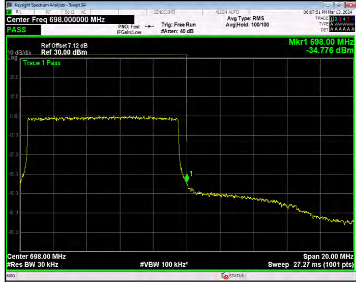
Band71 16QAM BW=15MHz Channel=133197 RB Size=1 Position=#0
