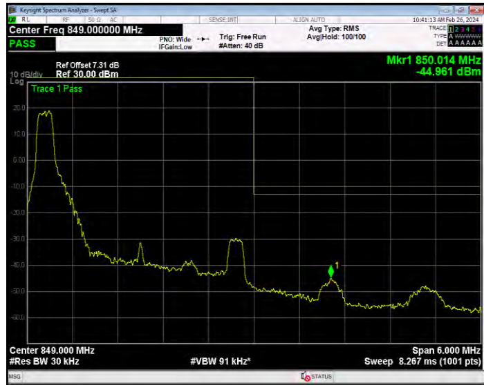
Band5 16QAM BW=3MHz Channel=20635 RB Size=15 Position=#0
