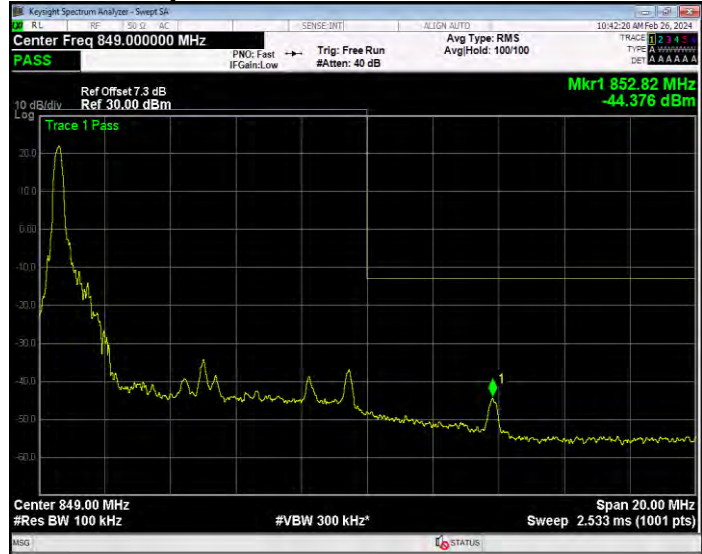
Band5 16QAM BW=10MHz Channel=20600 RB Size=50 Position=#0
