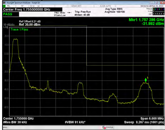
Band4 16QAM BW=3MHz Channel=20385 RB Size=15 Position=#0
