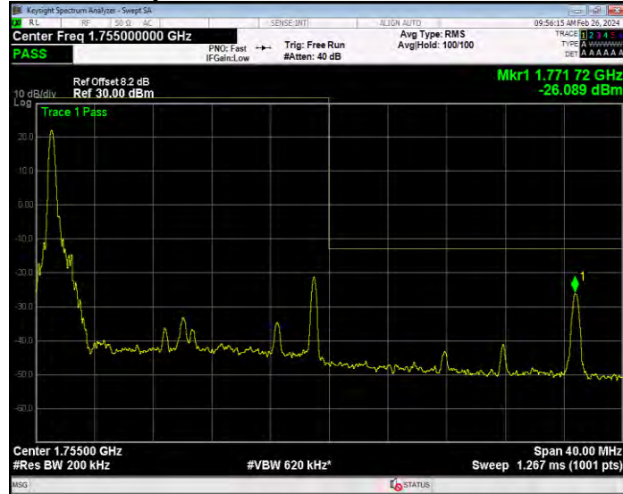
Band4 16QAM BW=20MHz Channel=20300 RB Size=100 Position=#0
