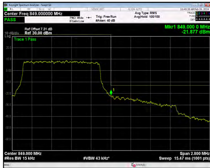
Band5 QPSK BW=10MHz Channel=20450 RB Size=1 Position=#0
