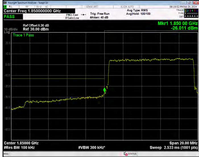
Band25 QPSK BW=10MHz Channel=26640 RB Size=50 Position=#0
