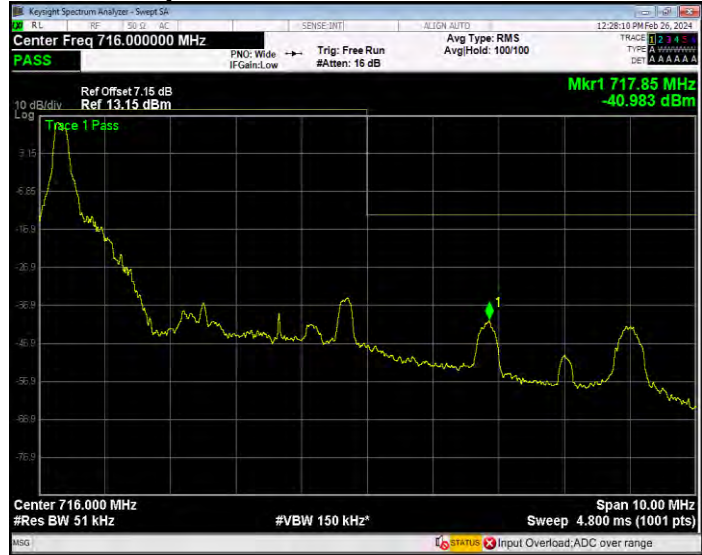
Band17 QPSK BW=5MHz Channel=23825 RB Size=25 Position=#0
