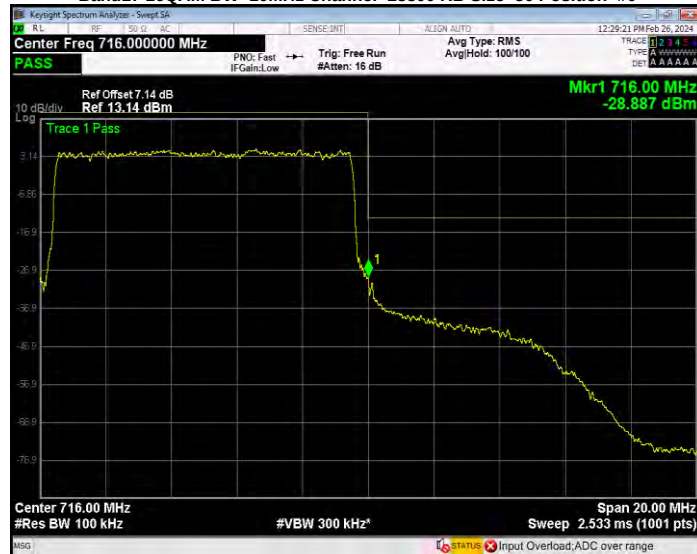
Band17 16QAM BW=5MHz Channel=23755 RB Size=1 Position=#0
