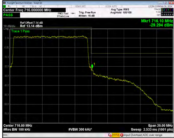
Band17 QPSK BW=5MHz Channel=23755 RB Size=1 Position=#0
