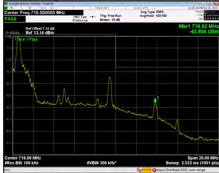
Band17 16QAM BW=10MHz Channel=23800 RB Size=50 Position=#0
