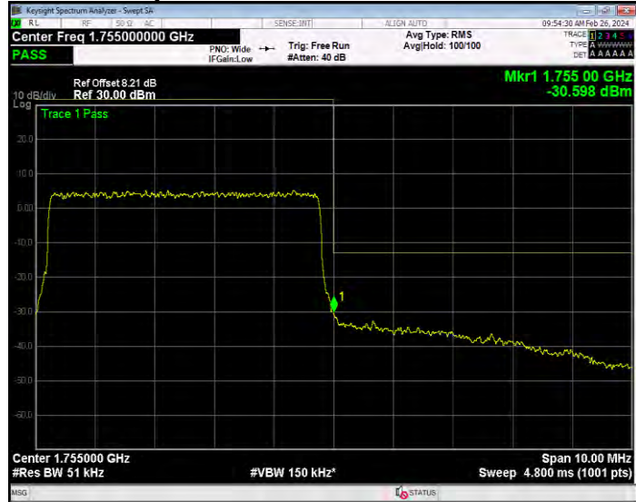
Band4 QPSK BW=1.4MHz Channel=19957 RB Size=1 Position=#0
