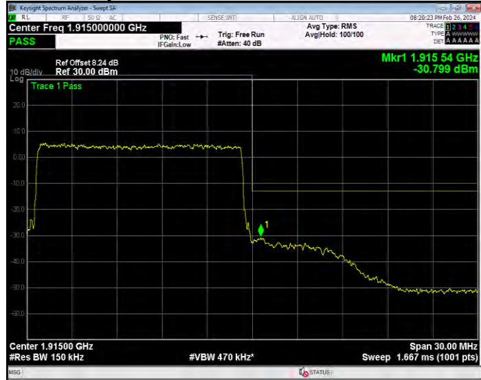
Band25 QPSK BW=20MHz Channel=26140 RB Size=100 Position=#0
