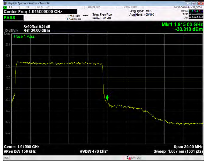
Band25 16QAM BW=20MHz Channel=26140 RB Size=100 Position=#0
