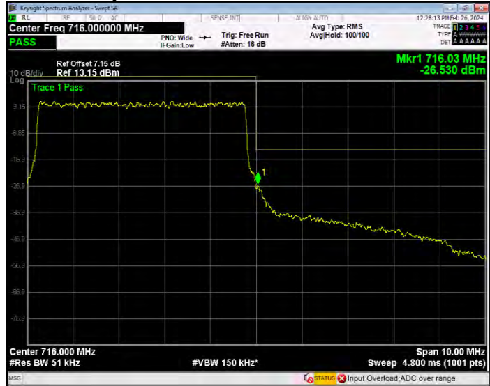
Band25 16QAM BW=1.4MHz Channel=26047 RB Size=6 Position=#0
