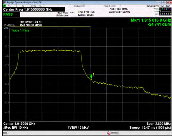
Band25 QPSK BW=10MHz Channel=26090 RB Size=50 Position=#0
