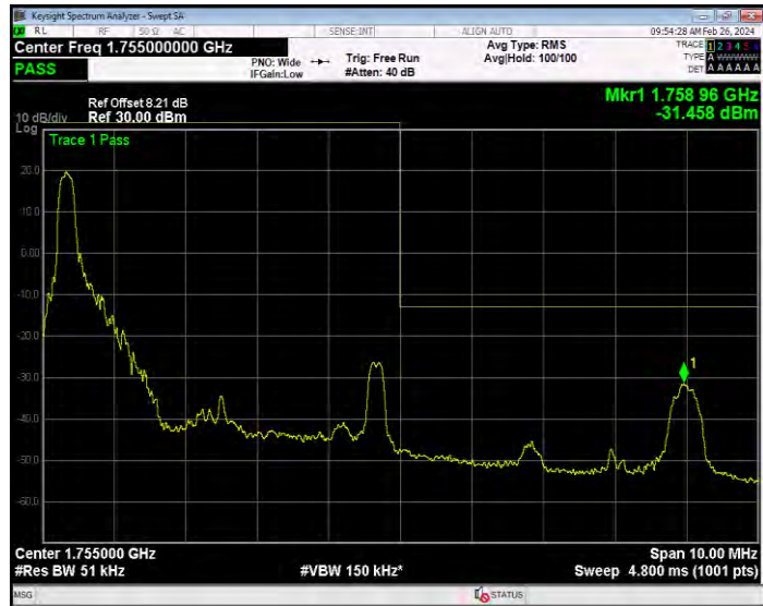
Band4 16QAM BW=5MHz Channel=20375 RB Size=25 Position=#0
