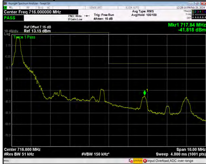
Band17 16QAM BW=5MHz Channel=23825 RB Size=25 Position=#0
