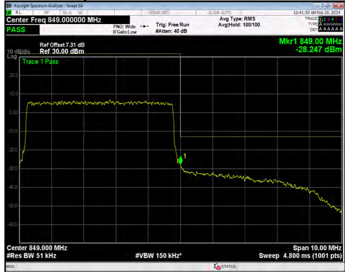
Band5 QPSK BW=1.4MHz Channel=20407 RB Size=1 Position=#0
