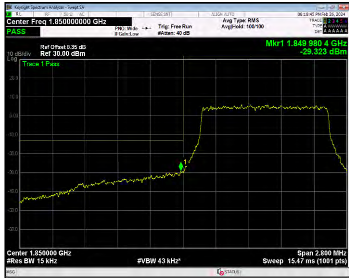
Band25 16QAM BW=1.4MHz Channel=26683 RB Size=6 Position=#0
