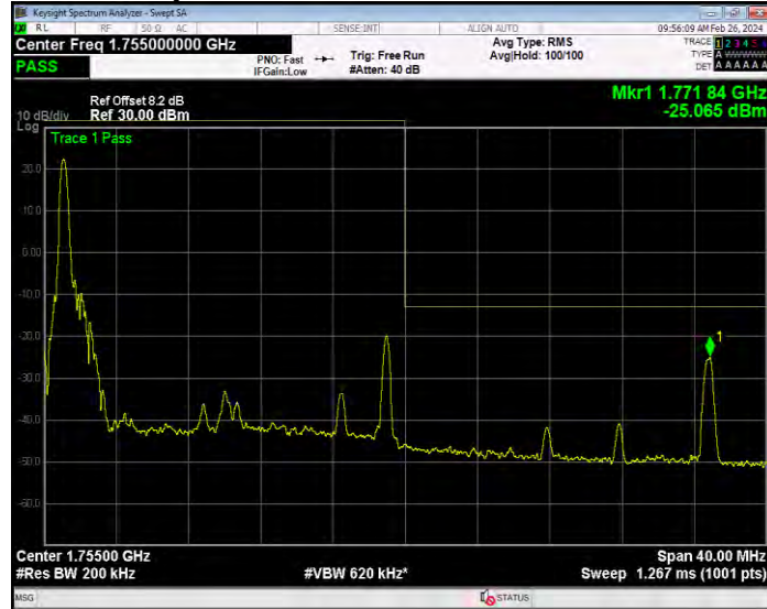
Band4 QPSK BW=20MHz Channel=20300 RB Size=100 Position=#0
