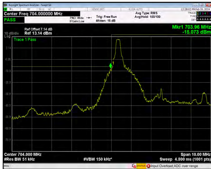
Band17 16QAM BW=5MHz Channel=23755 RB Size=25 Position=#0
