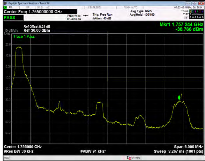
Band4 QPSK BW=3MHz Channel=20385 RB Size=15 Position=#0
