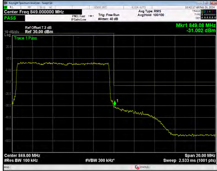
Band5 QPSK BW=3MHz Channel=20415 RB Size=1 Position=#0
