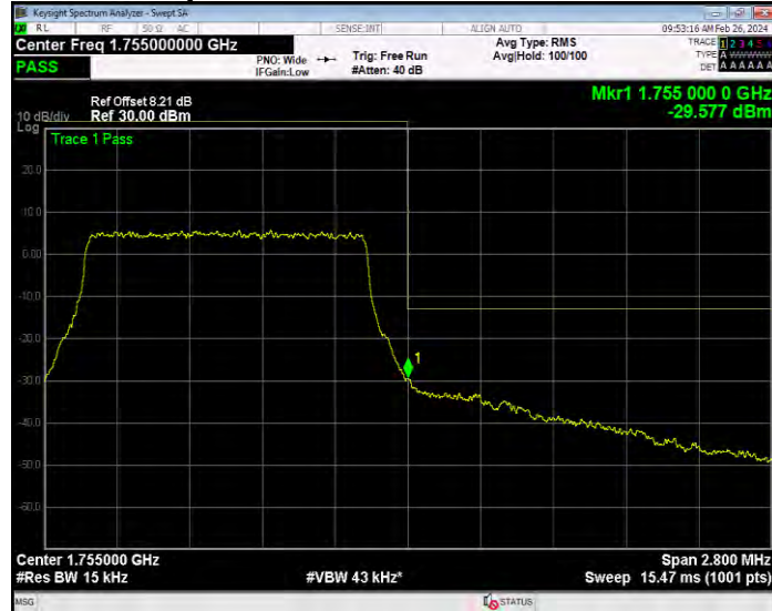
Band4 16QAM BW=10MHz Channel=20000 RB Size=1 Position=#0
