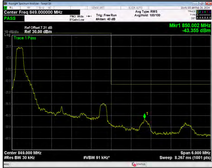
Band5 QPSK BW=3MHz Channel=20635 RB Size=15 Position=#0
