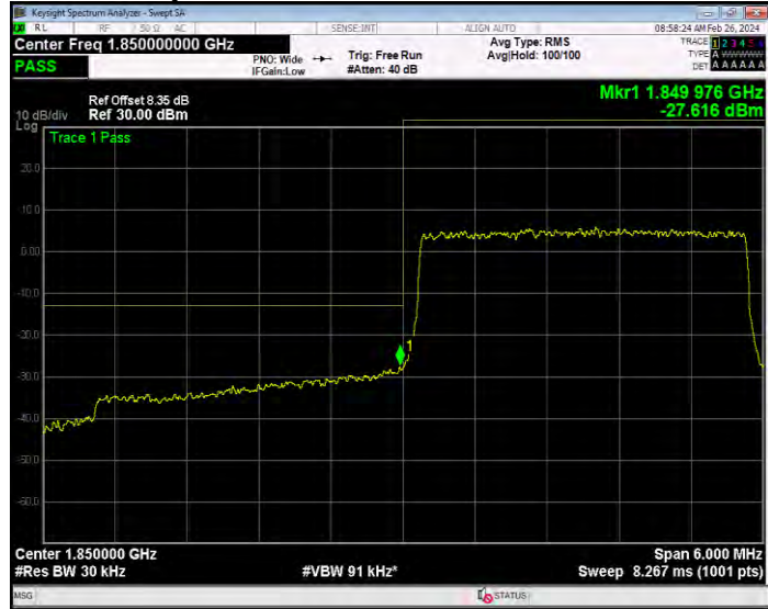
Band2 QPSK BW=3MHz Channel=19185 RB Size=1 Position=#0
