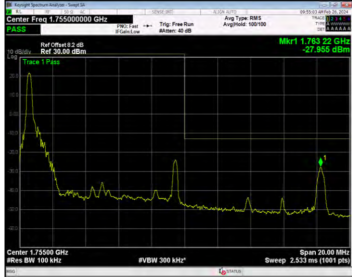
Band4 16QAM BW=10MHz Channel=20350 RB Size=50 Position=#0
