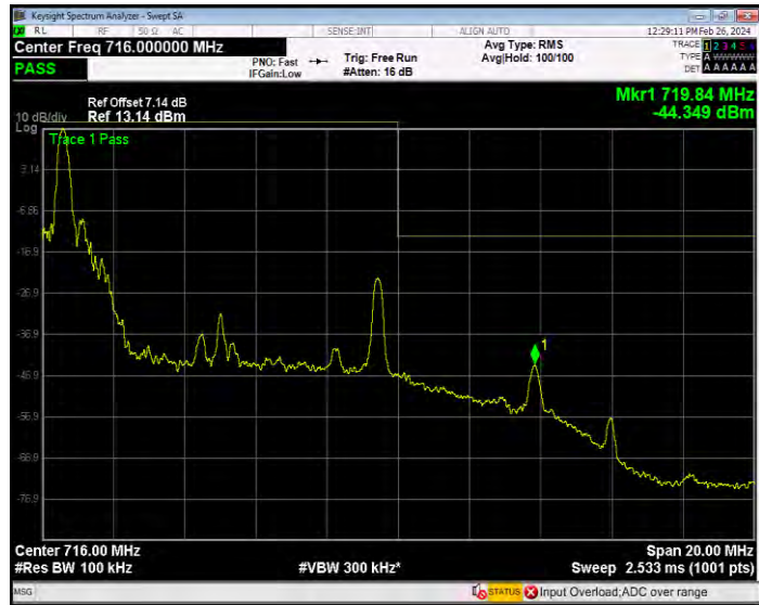
Band17 QPSK BW=10MHz Channel=23800 RB Size=50 Position=#0
