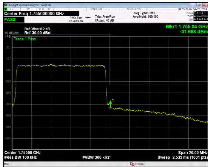
Band4 16QAM BW=15MHz Channel=20025 RB Size=1 Position=#0
