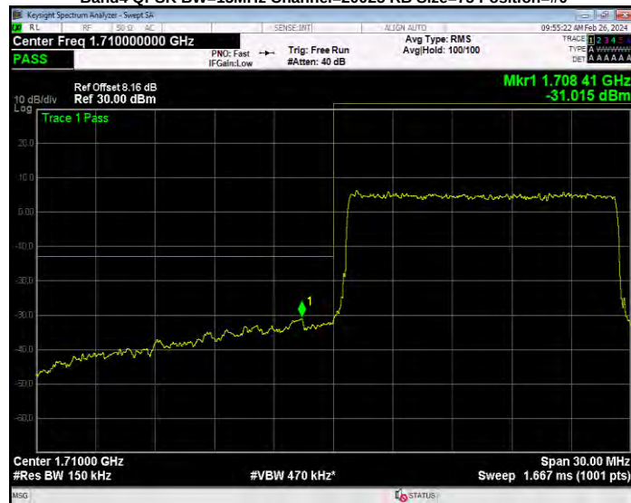
Band4 QPSK BW=15MHz Channel=20325 RB Size=1 Position=#0
