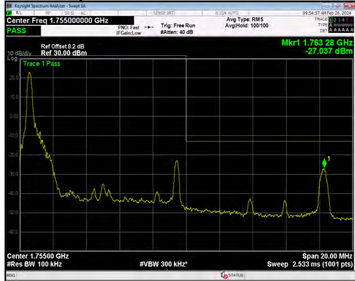
Band4 QPSK BW=10MHz Channel=20350 RB Size=50 Position=#0
