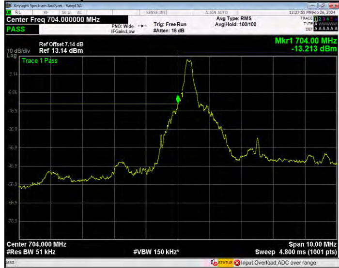
Band17 QPSK BW=5MHz Channel=23755 RB Size=25 Position=#0
