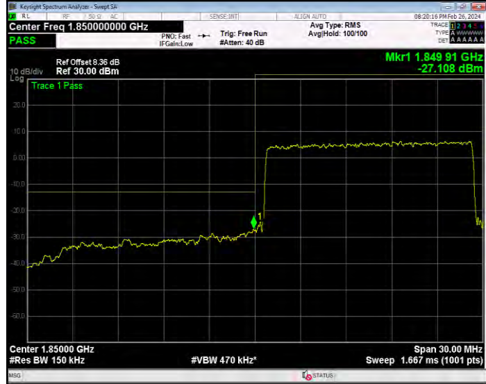
Band25 QPSK BW=15MHz Channel=26615 RB Size=75 Position=#0
