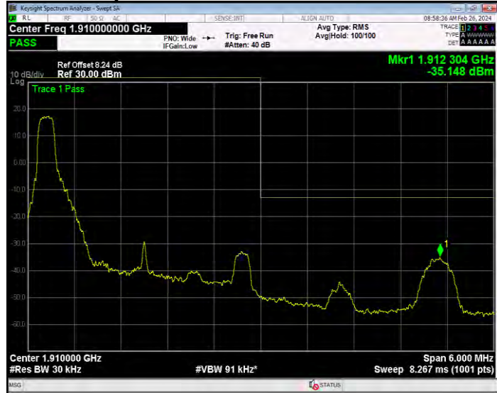
Band2 QPSK BW=3MHz Channel=19185 RB Size=15 Position=#0
