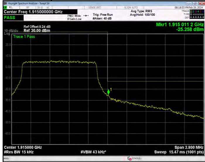
Band25 16QAM BW=10MHz Channel=26090 RB Size=50 Position=#0
