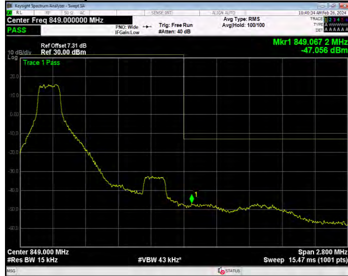
Band5 16QAM BW=1.4MHz Channel=20643 RB Size=6 Position=#0
