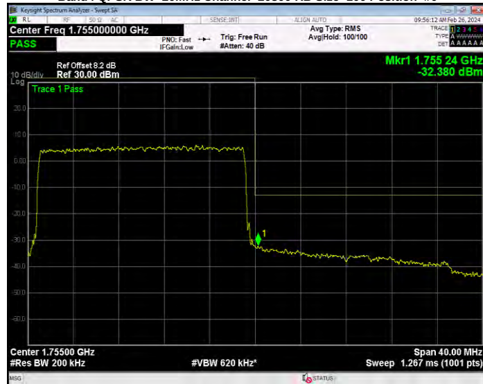
Band4 QPSK BW=3MHz Channel=19965 RB Size=1 Position=#0
