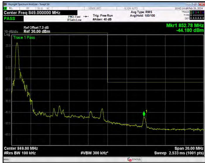
Band5 QPSK BW=10MHz Channel=20600 RB Size=50 Position=#0
