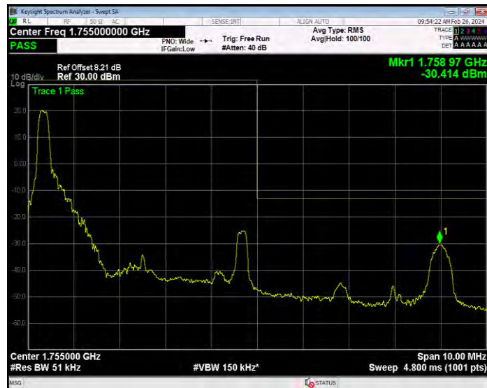
Band4 QPSK BW=5MHz Channel=20375 RB Size=25 Position=#0
