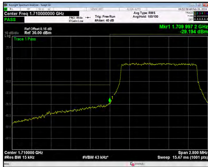
Band4 16QAM BW=1.4MHz Channel=20393 RB Size=1 Position=#0
