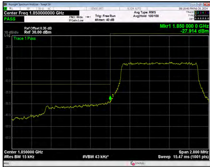
Band25 QPSK BW=1.4MHz Channel=26683 RB Size=6 Position=#0
