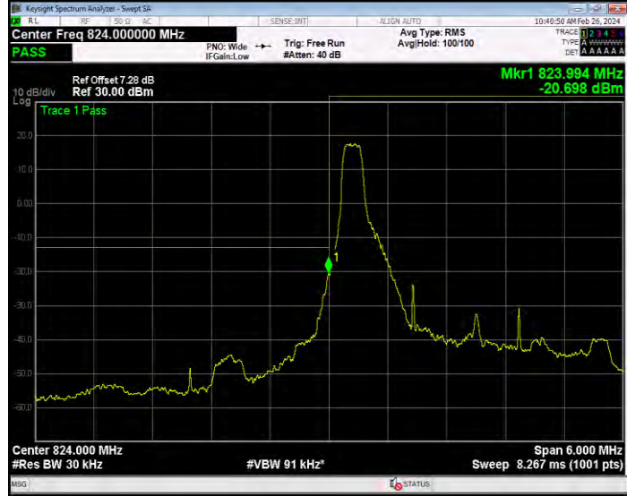
Band5 QPSK BW=3MHz Channel=20415 RB Size=15 Position=#0
