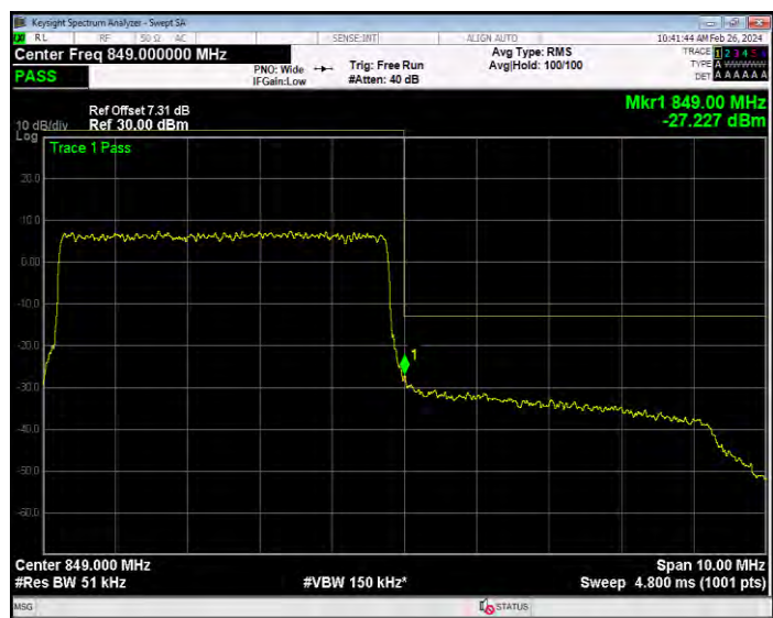
Band7 16QAM BW=10MHz Channel=20800 RB Size=1 Position=#0
