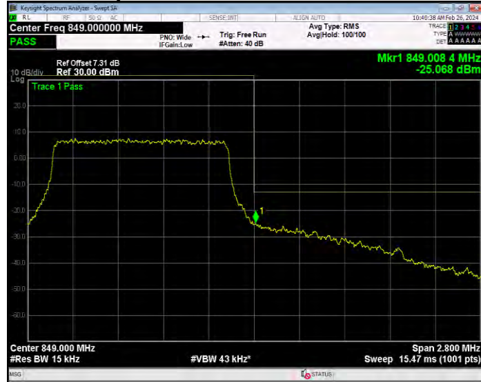
Band5 16QAM BW=10MHz Channel=20450 RB Size=1 Position=#0
