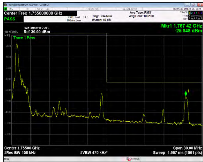
Band4 16QAM BW=15MHz Channel=20325 RB Size=75 Position=#0
