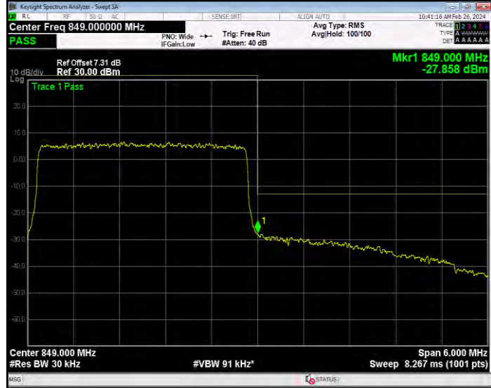
Band5 16QAM BW=5MHz Channel=20425 RB Size=1 Position=#0
