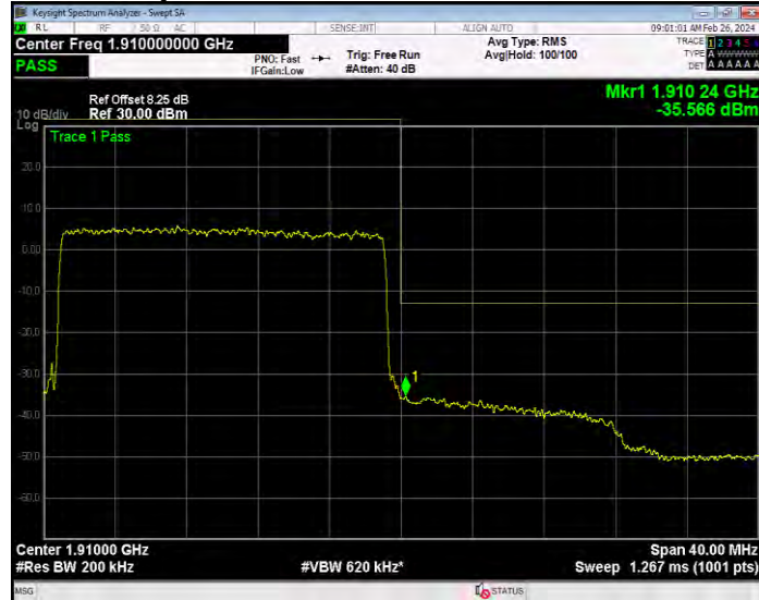
Band2 QPSK BW=3MHz Channel=18615 RB Size=1 Position=#0
