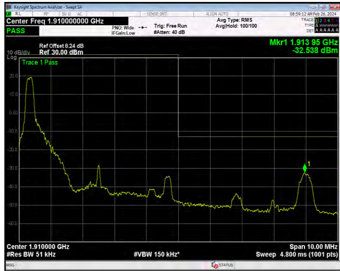
Band2 QPSK BW=5MHz Channel=19175 RB Size=25 Position=#0
