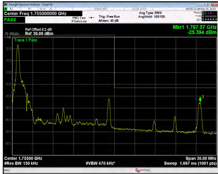
Band4 QPSK BW=15MHz Channel=20325 RB Size=75 Position=#0
