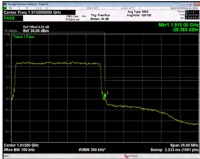
Band25 16QAM BW=15MHz Channel=26115 RB Size=75 Position=#0
