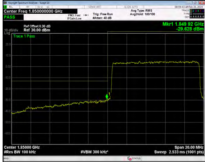
Band2 16QAM BW=10MHz Channel=19150 RB Size=1 Position=#0
