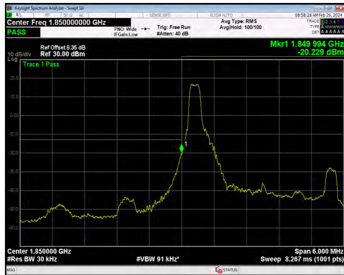
Band2 16QAM BW=3MHz Channel=18615 RB Size=15 Position=#0
