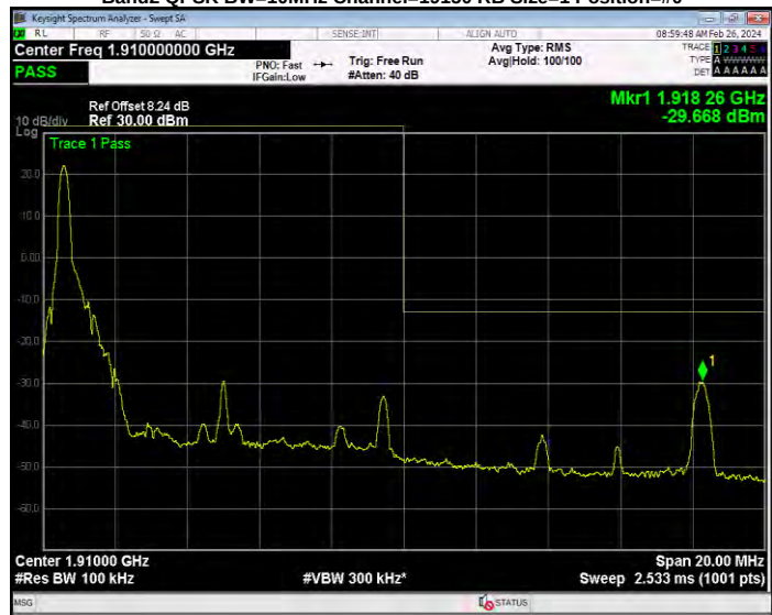
Band2 QPSK BW=10MHz Channel=19150 RB Size=50 Position=#0
