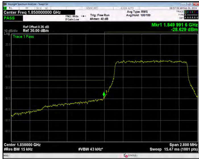
Band2 16QAM BW=1.4MHz Channel=19193 RB Size=1 Position=#0
