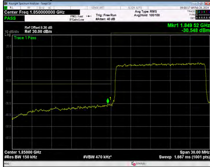
Band2 16QAM BW=15MHz Channel=19125 RB Size=1 Position=#0
