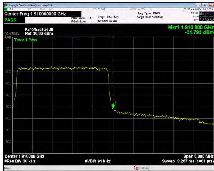
Band2 16QAM BW=5MHz Channel=18625 RB Size=1 Position=#0
