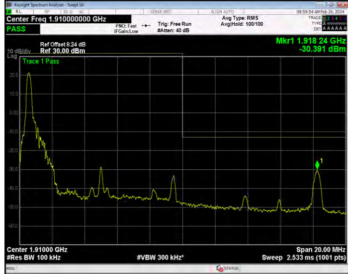
Band2 16QAM BW=10MHz Channel=19150 RB Size=50 Position=#0
