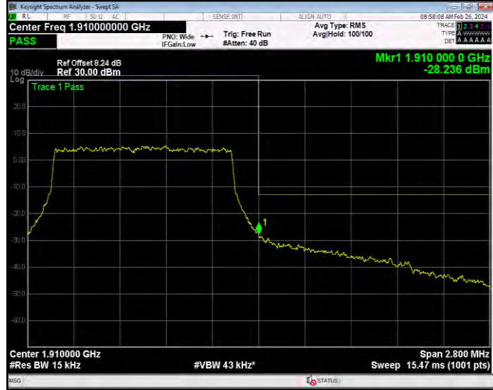
Band2 16QAM BW=10MHz Channel=18650 RB Size=1 Position=#0
