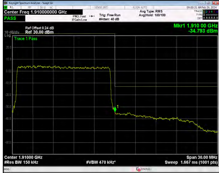
Band2 16QAM BW=20MHz Channel=18700 RB Size=1 Position=#0
