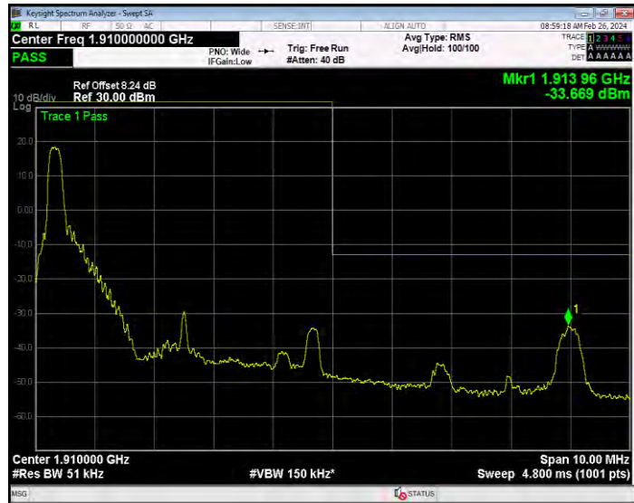
Band2 16QAM BW=5MHz Channel=19175 RB Size=25 Position=#0
