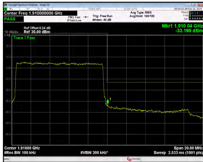
Band2 QPSK BW=15MHz Channel=18675 RB Size=1 Position=#0
