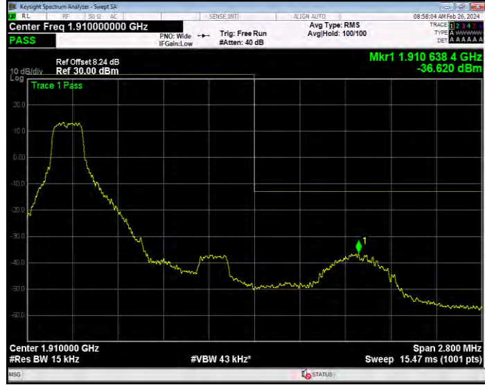
Band2 16QAM BW=1.4MHz Channel=19193 RB Size=6 Position=#0
