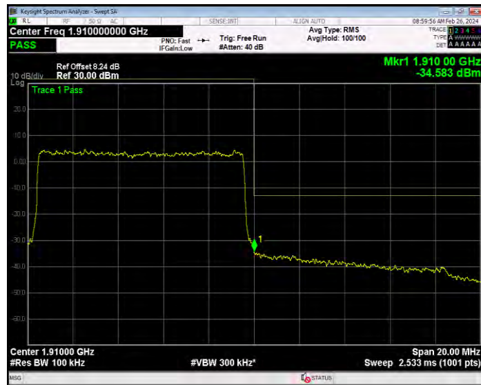
Band2 16QAM BW=15MHz Channel=18675 RB Size=1 Position=#0
