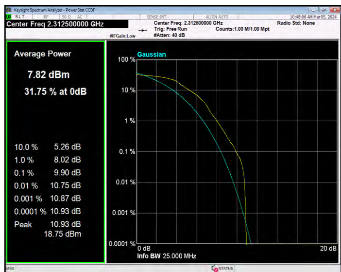
Band40(2350-2360) 16QAM BW=10MHz Channel=39200 RB Size=1 Position=#0
