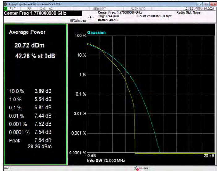
Band66 16QAM BW=3MHz Channel=131987 RB Size=1 Position=#0
