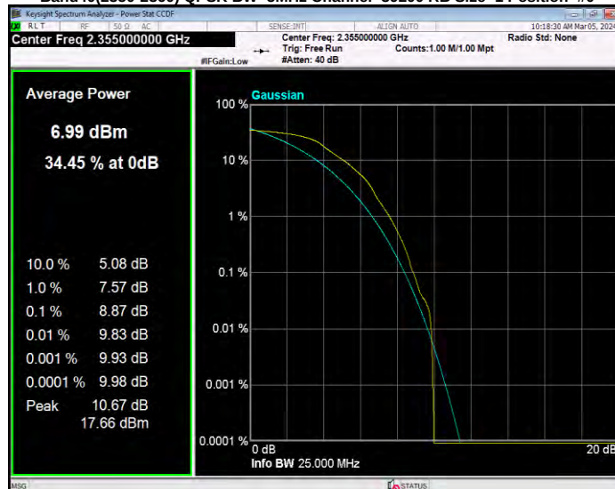
Band40(2350-2360) QPSK BW=5MHz Channel=39225 RB Size=1 Position=#0
