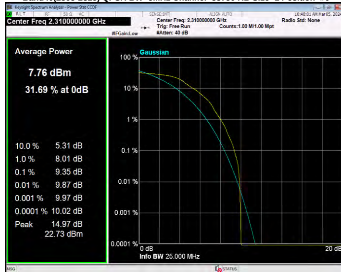
Band40(2305-2315) QPSK BW=5MHz Channel=38775 RB Size=1 Position=#0
