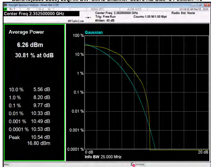
Band40(2350-2360) 16QAM BW=5MHz Channel=39200 RB Size=1 Position=#0
