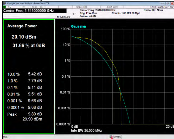
Band38 QPSK BW=15MHz Channel=37825 RB Size=1 Position=#0
