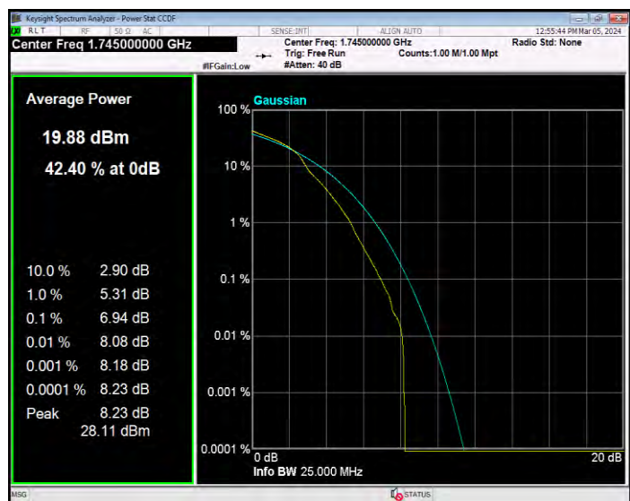
Band66 16QAM BW=20MHz Channel=132572 RB Size=1 Position=#0
