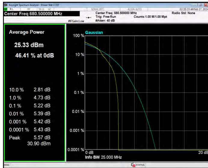
Band71 16QAM BW=20MHz Channel=133372 RB Size=1 Position=#0
