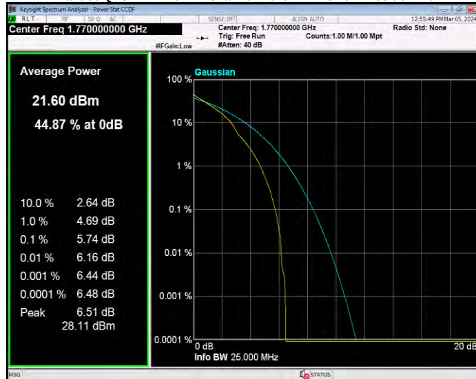
Band66 QPSK BW=3MHz Channel=131987 RB Size=1 Position=#0
