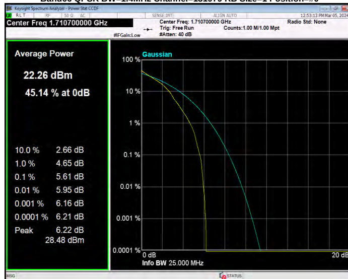
Band66 QPSK BW=1.4MHz Channel=132322 RB Size=1 Position=#0
