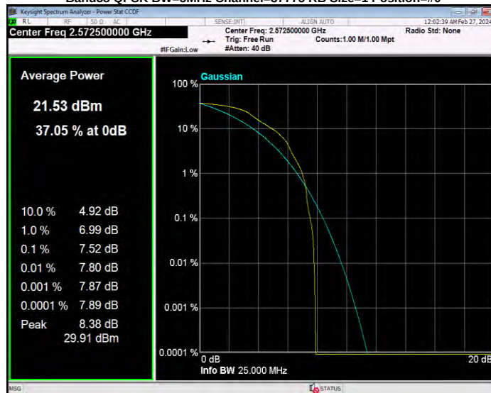
Band38 QPSK BW=5MHz Channel=38000 RB Size=1 Position=#0
