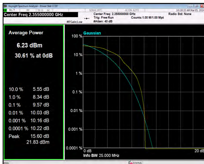
Band40(2350-2360) 16QAM BW=5MHz Channel=39225 RB Size=1 Position=#0
