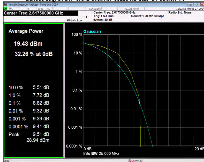
Band38 QPSK BW=10MHz Channel=37800 RB Size=1 Position=#0
