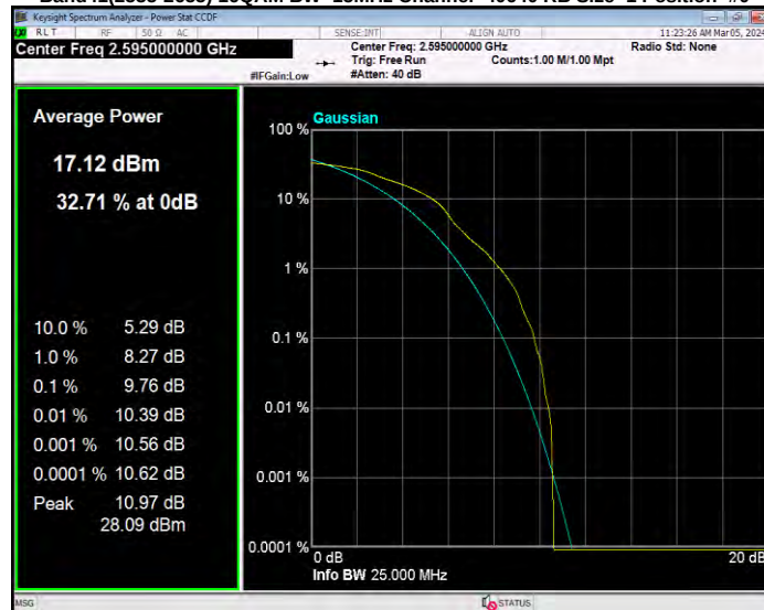
Band41(2535-2655) 16QAM BW=20MHz Channel=40640 RB Size=1 Position=#0
