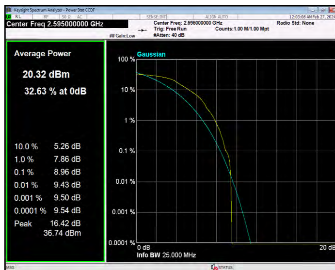
Band38 QPSK BW=10MHz Channel=38200 RB Size=1 Position=#0
