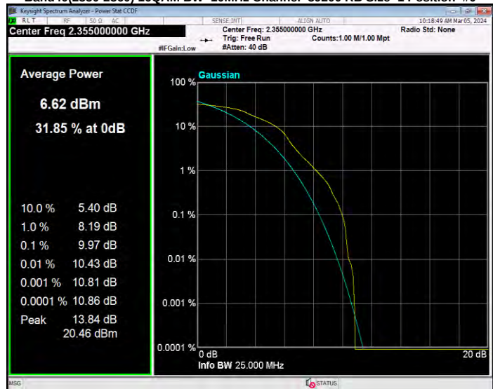
Band40(2350-2360) 16QAM BW=5MHz Channel=39175 RB Size=1 Position=#0
