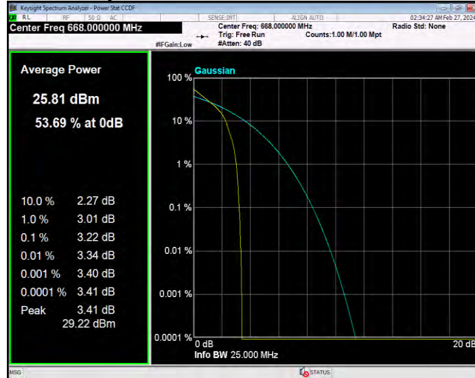
Band71 QPSK BW=10MHz Channel=133297 RB Size=1 Position=#0
