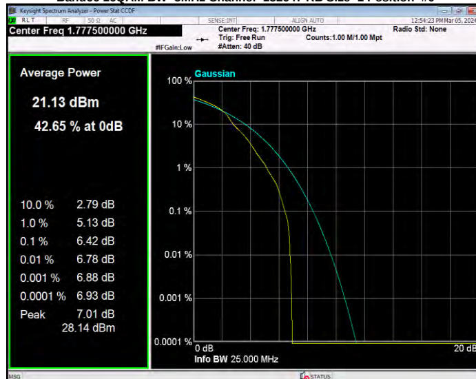
Band66 QPSK BW=1.4MHz Channel=131979 RB Size=1 Position=#0
