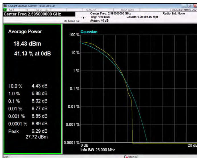
Band41(2535-2655) QPSK BW=5MHz Channel=40640 RB Size=1 Position=#0
