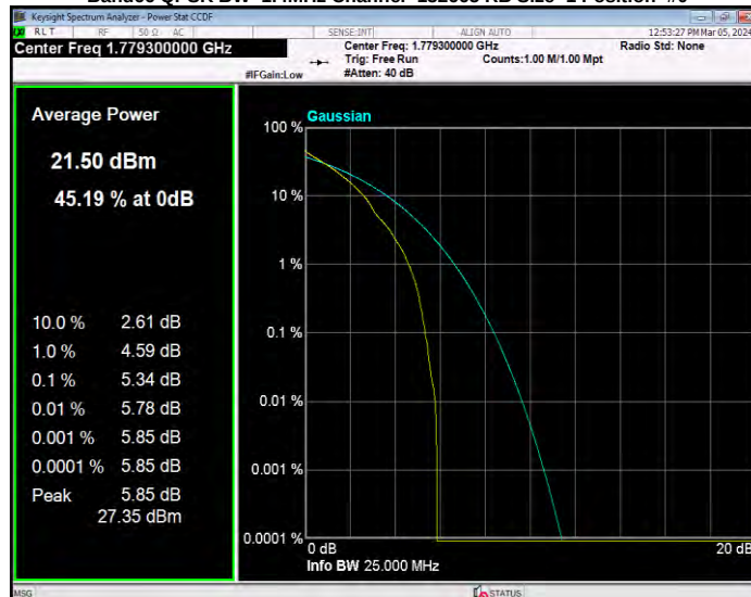
Band66 QPSK BW=10MHz Channel=132022 RB Size=1 Position=#0
