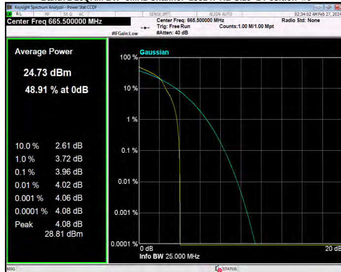
Band71 16QAM BW=5MHz Channel=133297 RB Size=1 Position=#0
