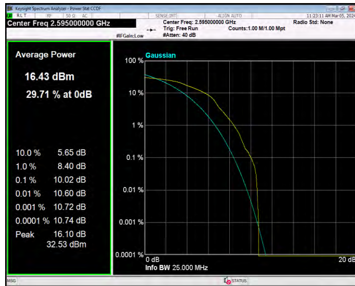
Band41(2535-2655) QPSK BW=10MHz Channel=40640 RB Size=1 Position=#0
