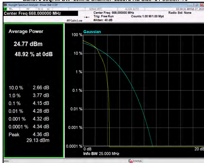
Band71 16QAM BW=10MHz Channel=133297 RB Size=1 Position=#0
