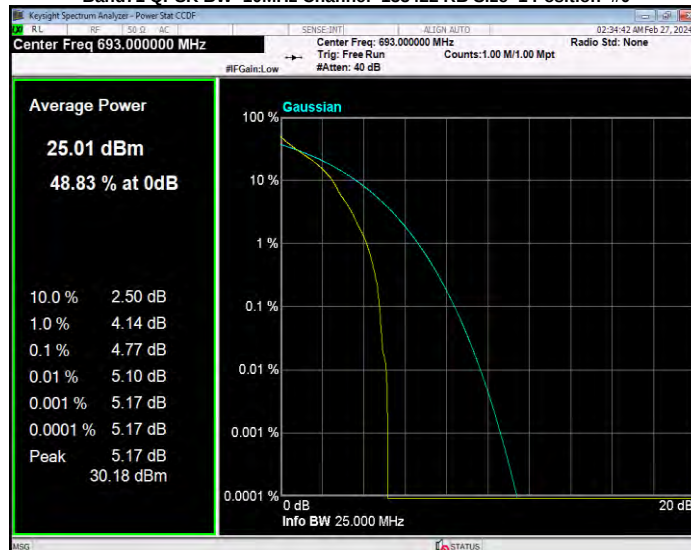
Band71 QPSK BW=15MHz Channel=133197 RB Size=1 Position=#0
