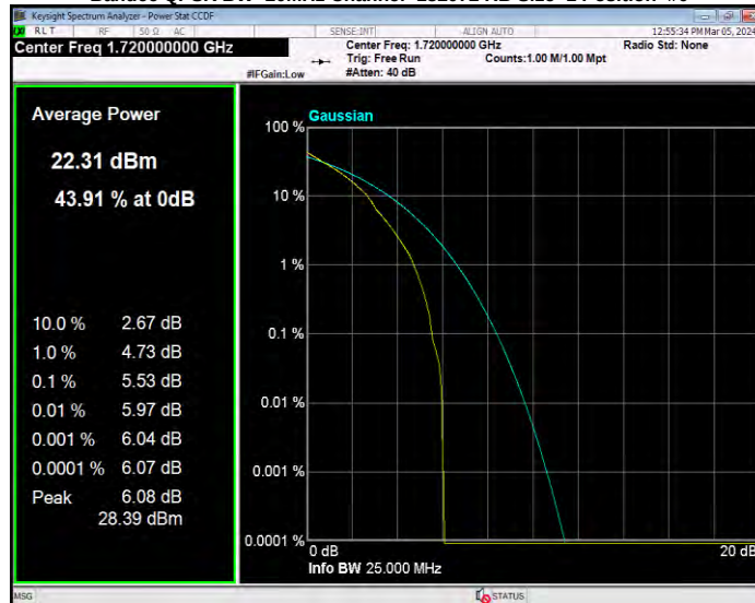
Band66 QPSK BW=20MHz Channel=132322 RB Size=1 Position=#0
