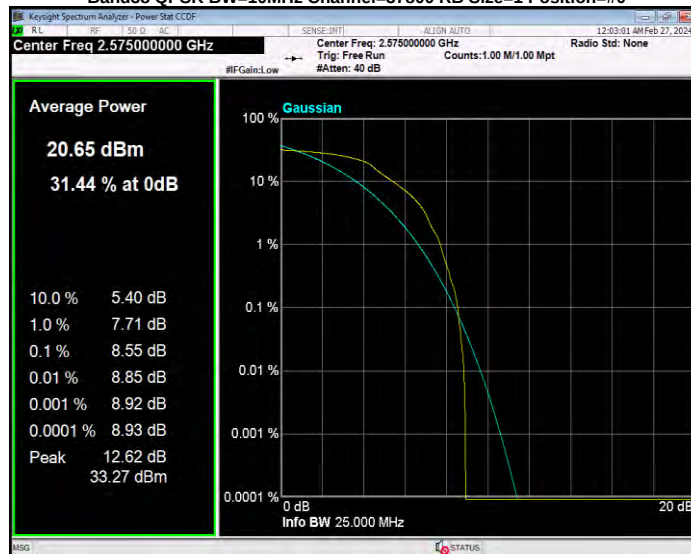
Band38 QPSK BW=10MHz Channel=38000 RB Size=1 Position=#0
