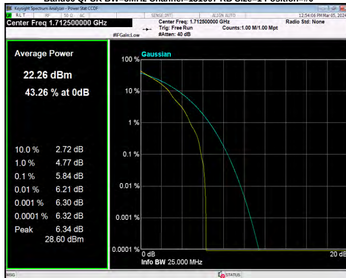
Band66 QPSK BW=5MHz Channel=132322 RB Size=1 Position=#0
