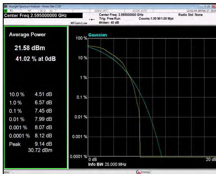
Band38 QPSK BW=5MHz Channel=38225 RB Size=1 Position=#0
