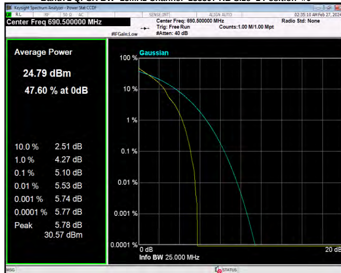
Band71 QPSK BW=20MHz Channel=133222 RB Size=1 Position=#0
