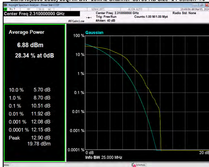
Band40(2305-2315) 16QAM BW=5MHz Channel=38725 RB Size=1 Position=#0
