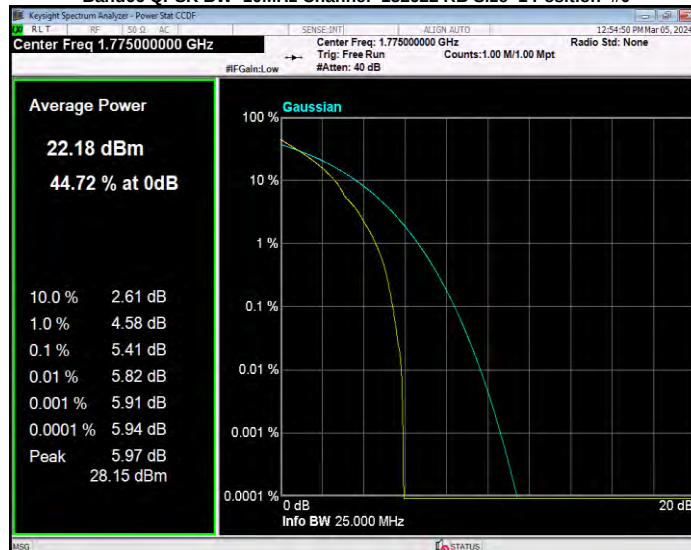
Band66 QPSK BW=15MHz Channel=132047 RB Size=1 Position=#0
