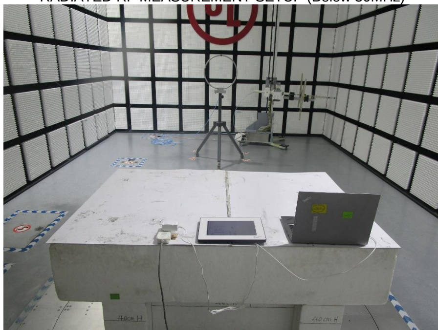
RADIATED RF MEASUREMENT SETUP (Below 30MHz)
