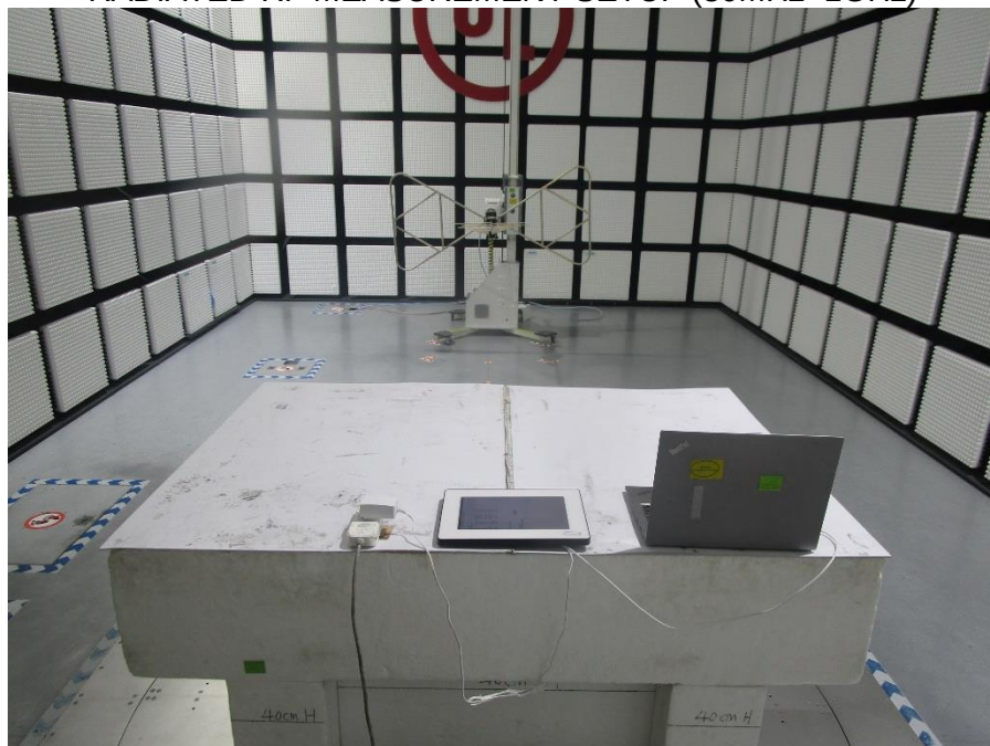
RADIATED RF MEASUREMENT SETUP (Below 30MHz)
