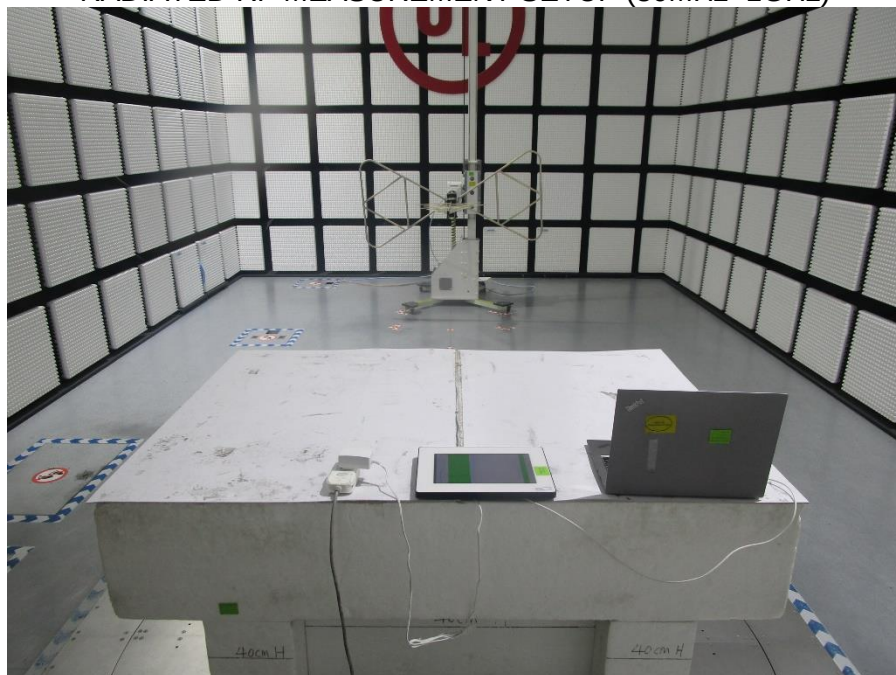
RADIATED RF MEASUREMENT SETUP (Below 30MHz)
