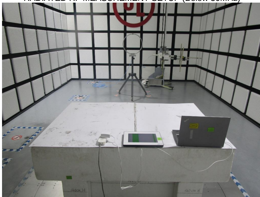
RADIATED RF MEASUREMENT SETUP (Below 30MHz)
