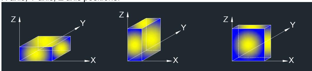
Note: For all radiated test, EUT in each of three orthogonal axis emissions had been tested, but only the worst case (Z axis) data recorded in the report.
