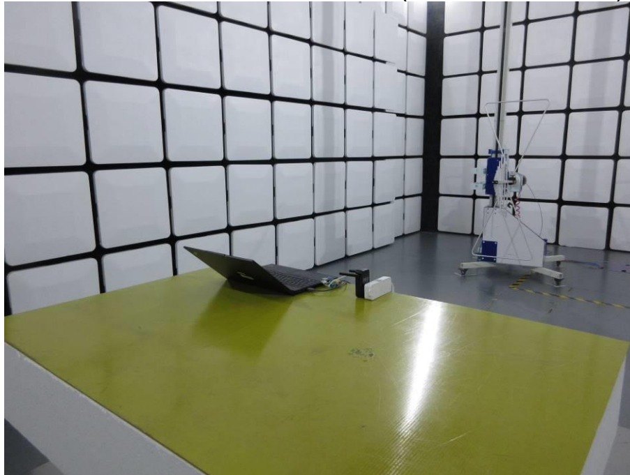
RADIATED RF MEASUREMENT SETUP (30MHz ~ 1 GHz-Y axis)
