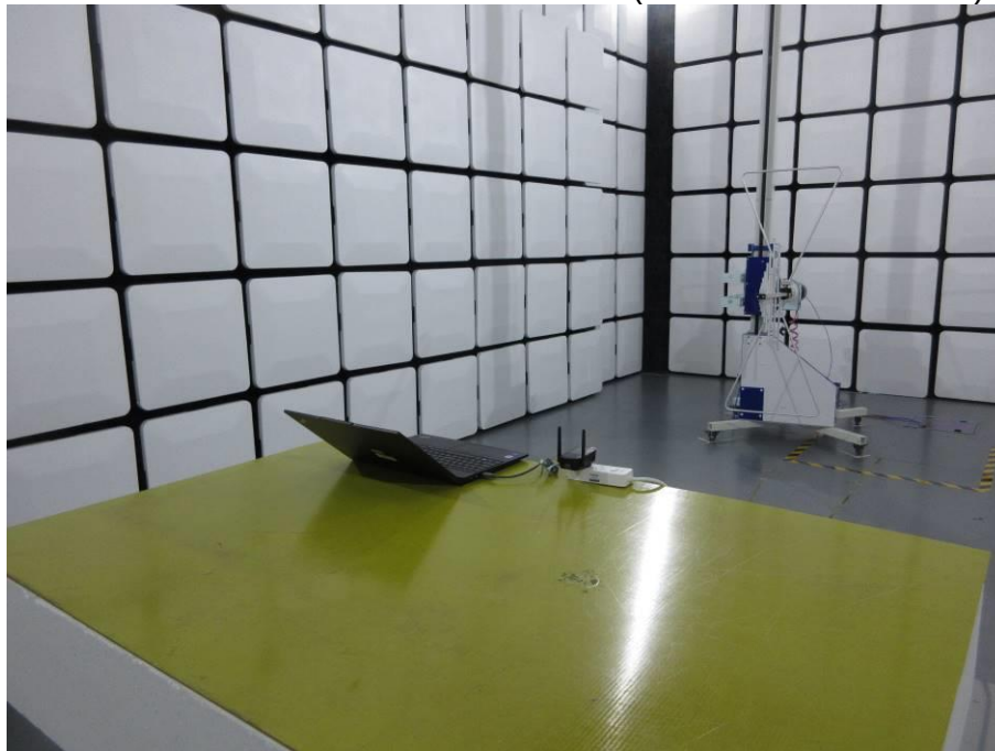
RADIATED RF MEASUREMENT SETUP (30MHz ~ 1 GHz-X axis)
