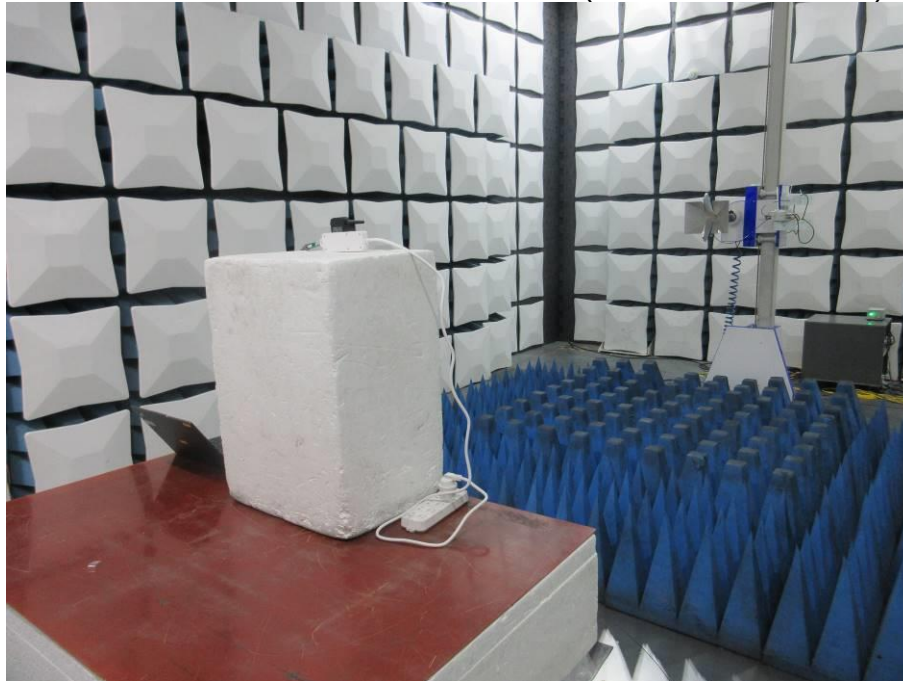
RADIATED RF MEASUREMENT SETUP (ABOVE 1 GHz-Z axis)
