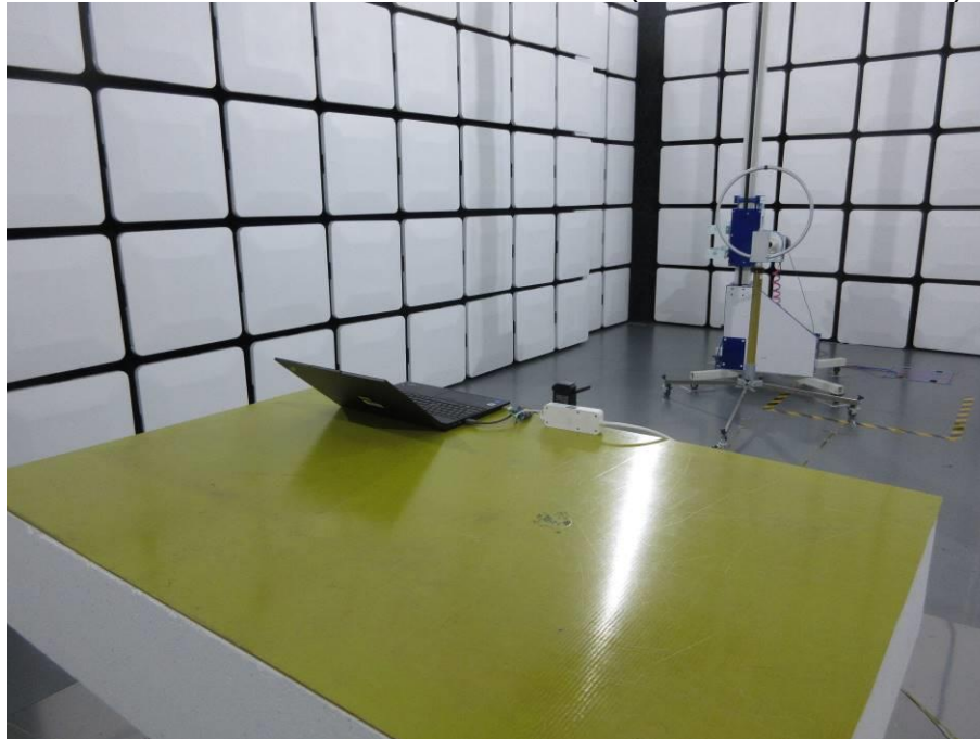
RADIATED RF MEASUREMENT SETUP (9kHz ~ 30 MHz-Z axis)
