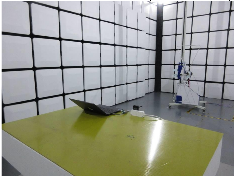
RADIATED RF MEASUREMENT SETUP (30MHz ~ 1 GHz-Z axis)
