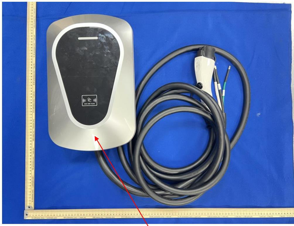
**Product Name: Wall mounted AC electric vehicle supply equipment**
