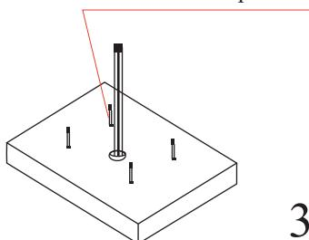
Uninstall the screws of base cover and lift the cover.
