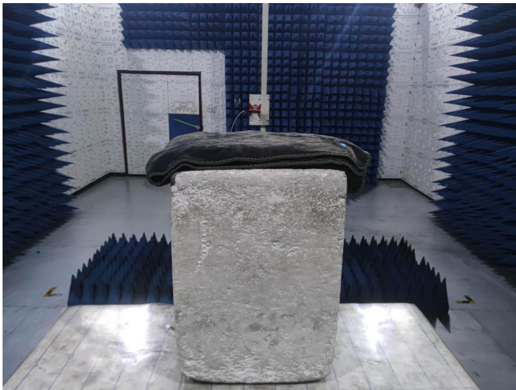
RADIATED EMISSION TEST SETUP ABOVE 1GHz
