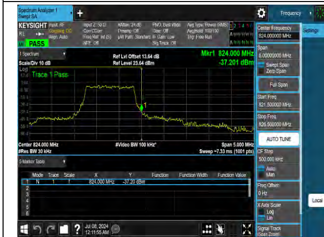
QPSK High channel-6 RB offset 0
