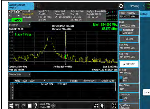
QPSK Low channel-6 RB offset 0
