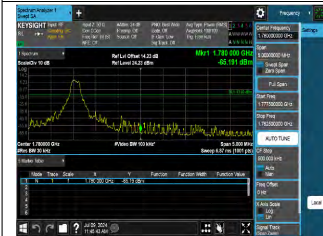
QPSK High channel-6 RB offset 0
