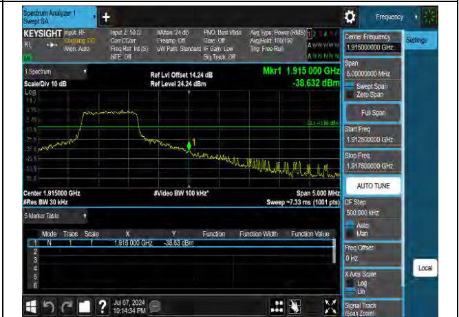
16QAM High channel-5 RB offset 0
