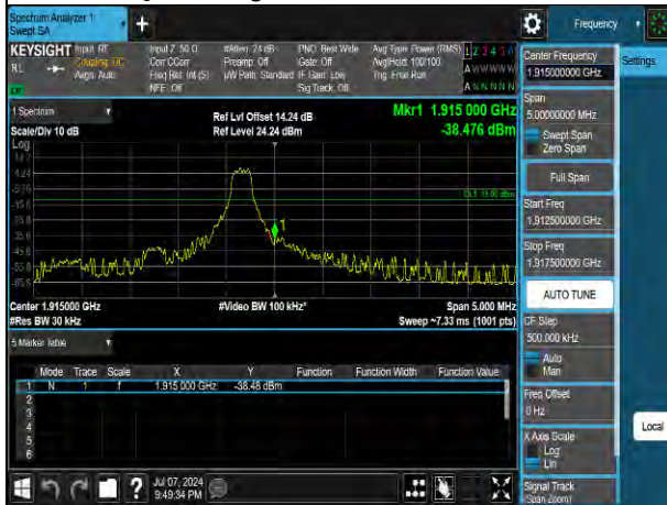
QPSK High channel-1 RB offset max
