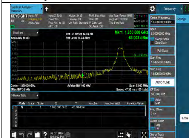
QPSK Low channel-1 RB offset 0
