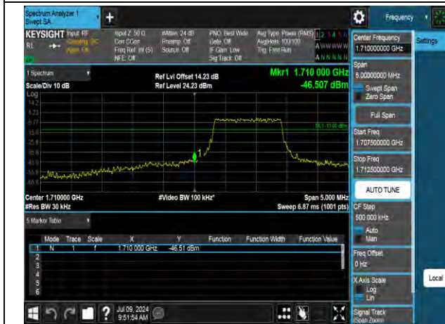
QPSK Low channel-6 RB offset 0
