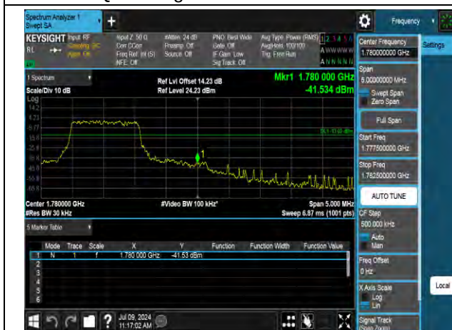
QPSK High channel-6 RB offset 0
