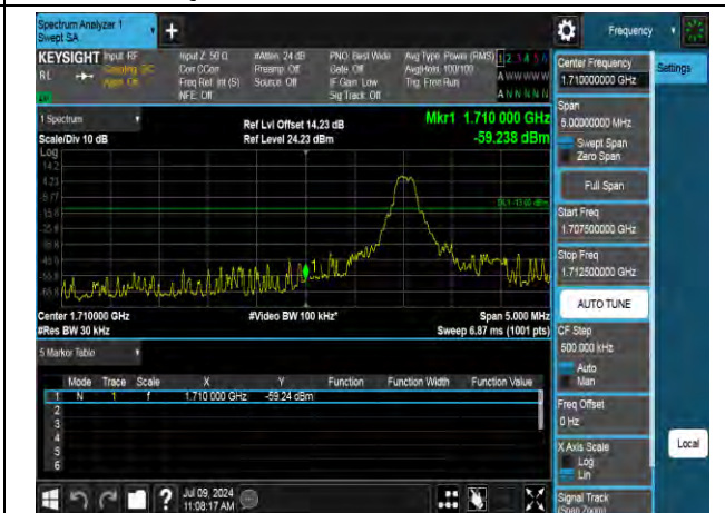
16QAM Low channel-5 RB offset 0
