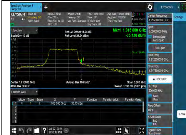
QPSK High channel-6 RB offset 0
