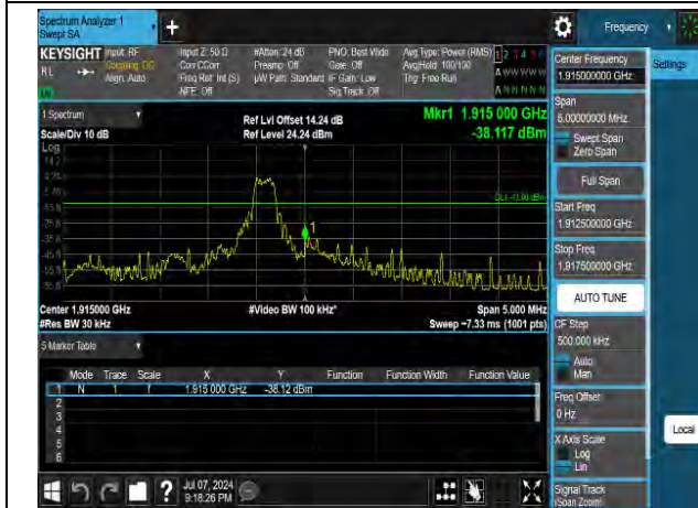
QPSK High channel-6 RB offset 0
