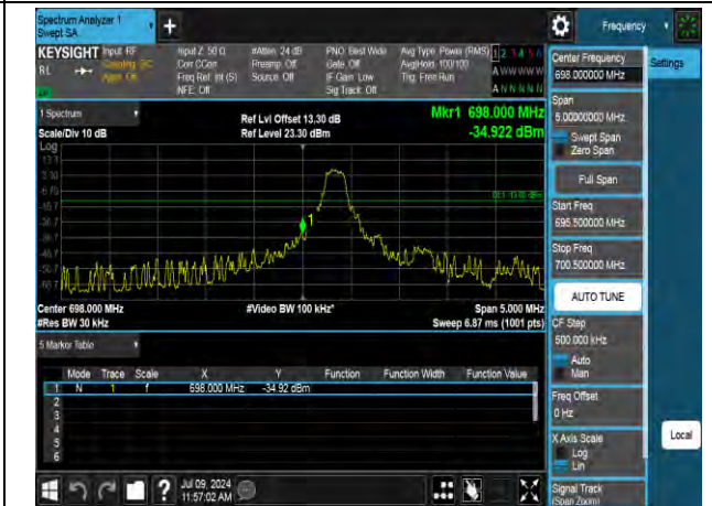
16QAM Low channel-5 RB offset 0
