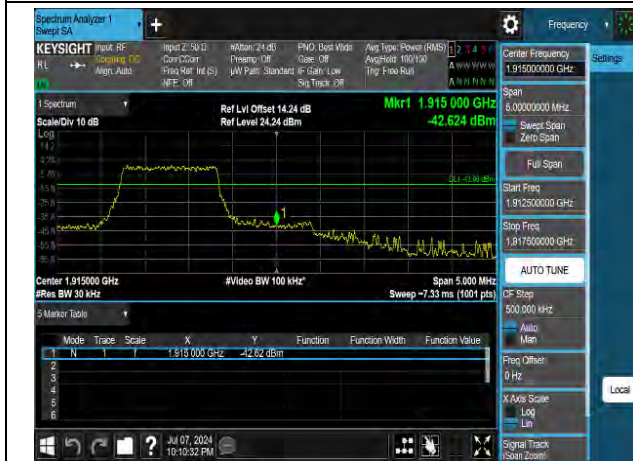
QPSK High channel-6 RB offset 0
