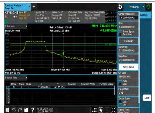
16QAM High channel-5 RB offset 0
