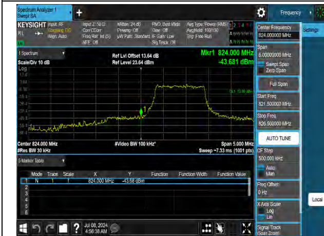
QPSK High channel-1 RB offset max
