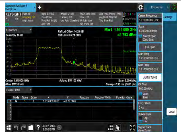
16QAM High channel-5 RB offset 0
