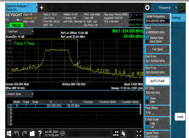
16QAM High channel-5 RB offset 0
