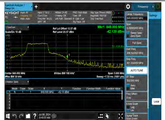
16QAM High channel-5 RB offset 0
