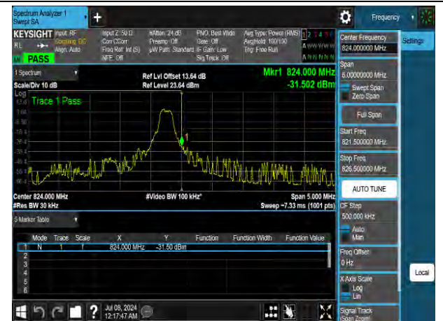
16QAM High channel-5 RB offset 0
