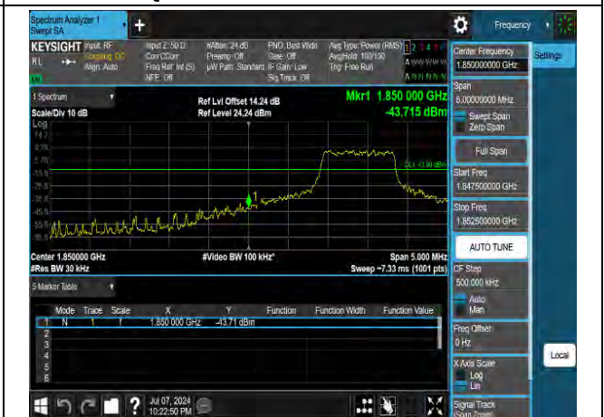
16QAM Low channel-5 RB offset 0
