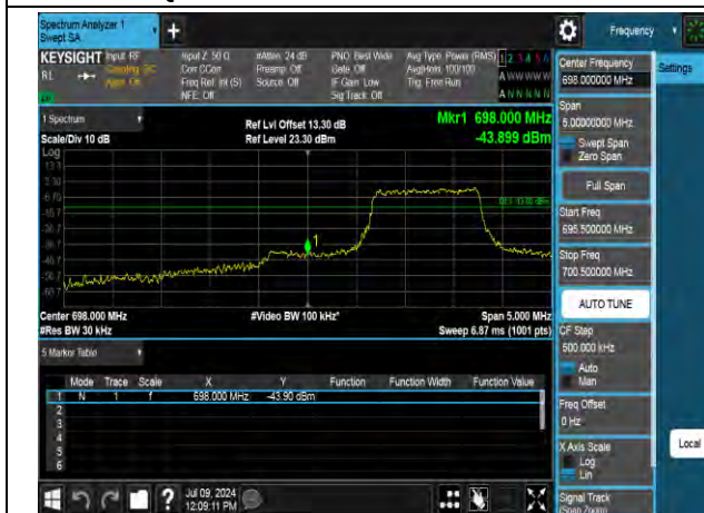
QPSK Low channel-6 RB offset 0
