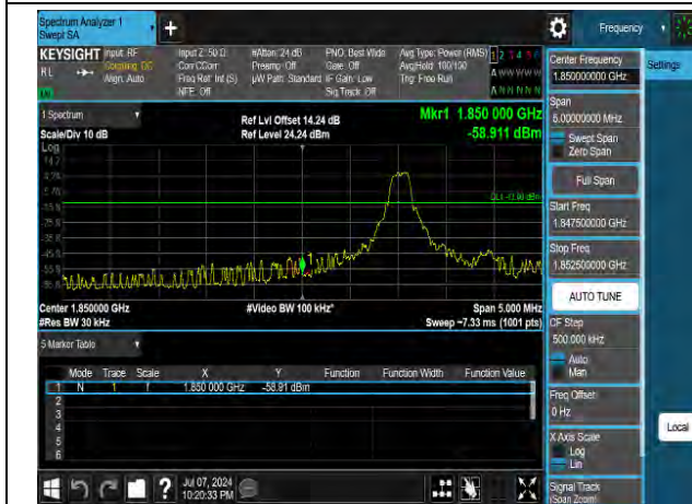
QPSK Low channel-6 RB offset 0
