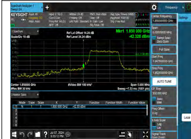
QPSK High channel-1 RB offset max
