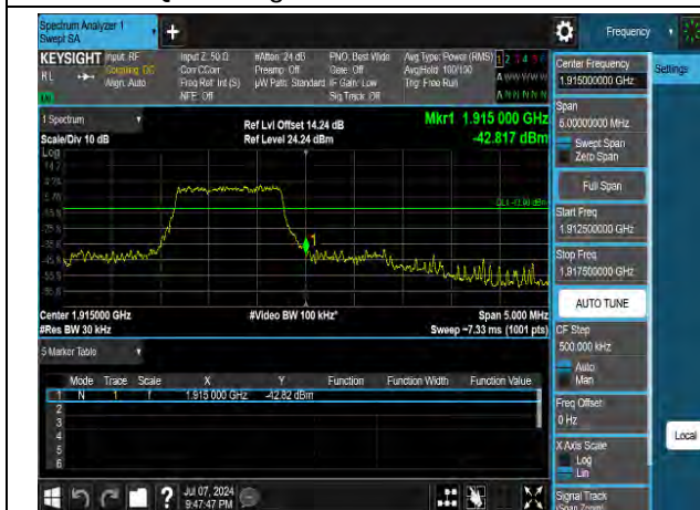
QPSK High channel-6 RB offset 0
