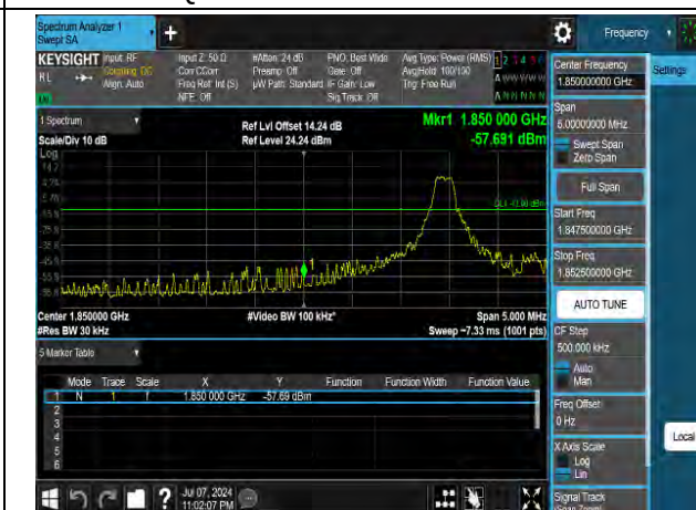
16QAM Low channel-1 RB offset 0
