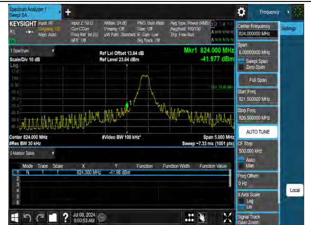
16QAM Low channel-1 RB offset 0
