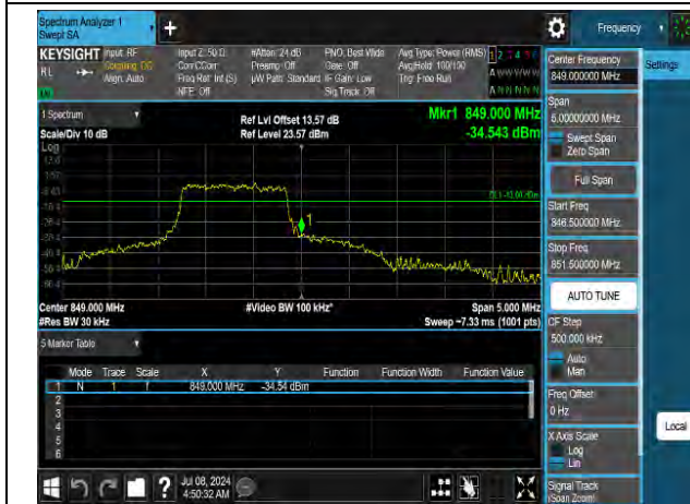
QPSK High channel-6 RB offset 0
