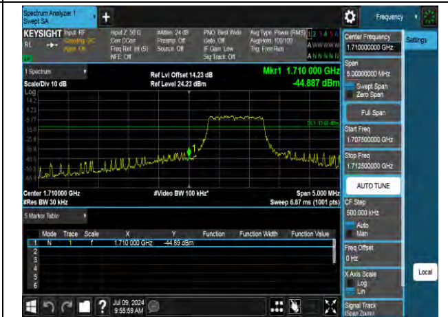
16QAM Low channel-5 RB offset 0
