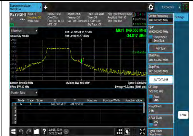
16QAM High channel-5 RB offset 0
