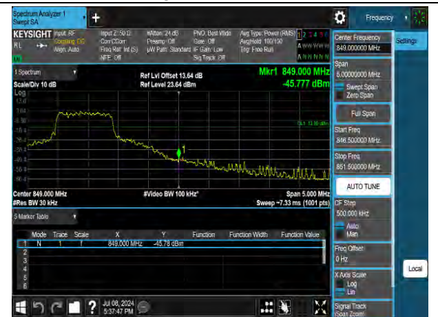
16QAM High channel-5 RB offset 0
