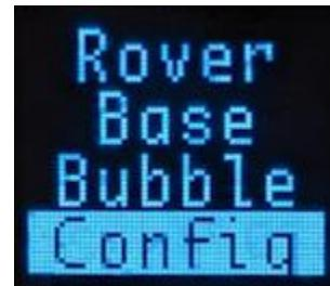
Now the wifi is turned on and a new Wifi SSID is available to connect to. You can connect to the 'RTK Config' SSID from your phone or computer without a password. After connecting, open a web browser and go to 192.168.4.1. This will show a menu to change the settings on the device.
