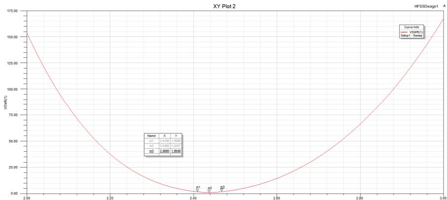
Central frequency point impedance: 50 ohm @2.438GHz
