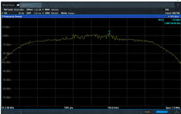
\pi/4 -DQPSK on Channel 78
