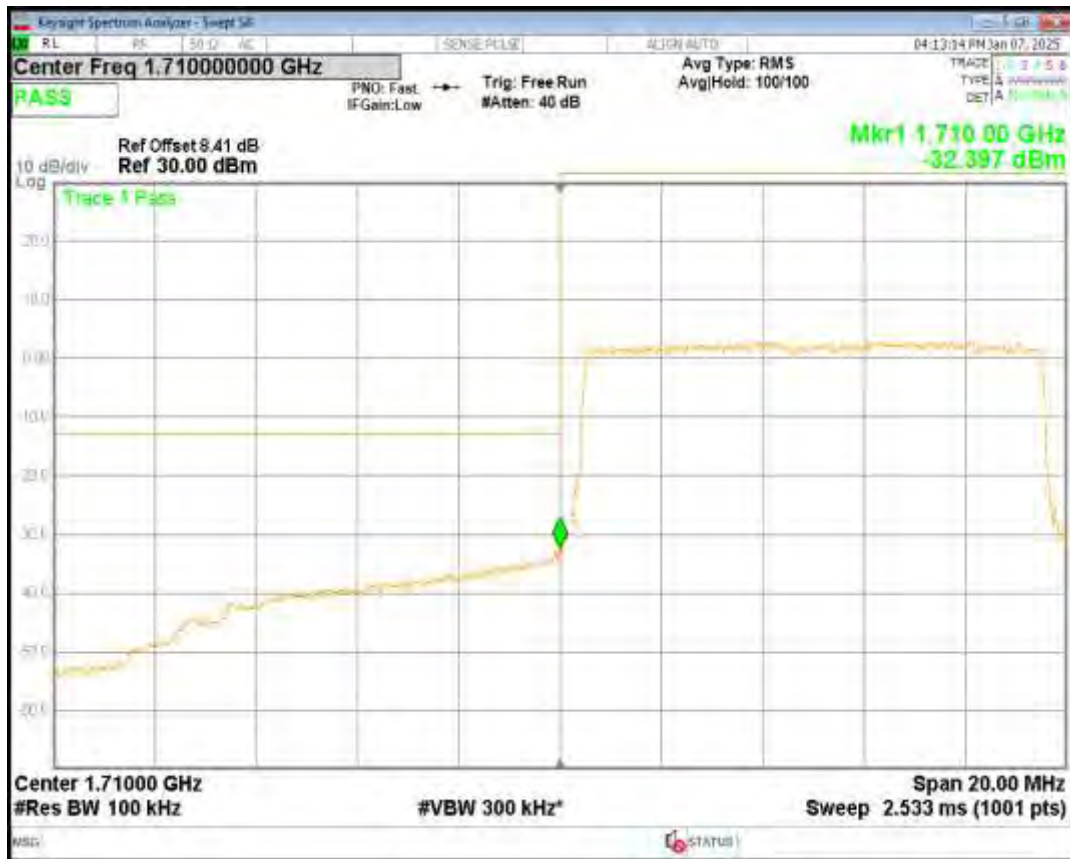
Band4 QPSK BW=10MHz Channel=20350 RB Size=50 Position=#0
