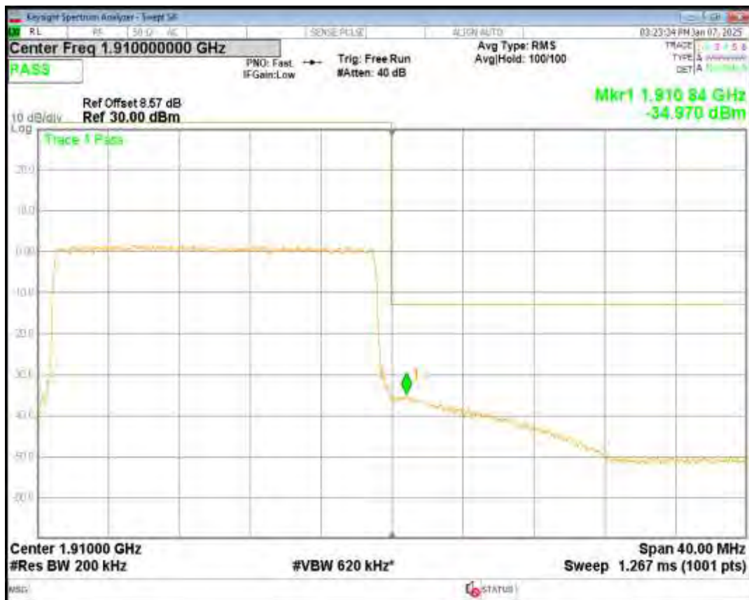
Band2 16QAM BW=3MHz Channel=18615 RB Size=15 Position=#0
