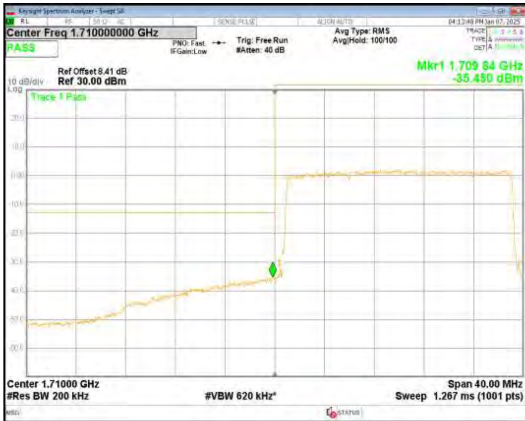
Band4 16QAM BW=20MHz Channel=20300 RB Size=100 Position=#0
