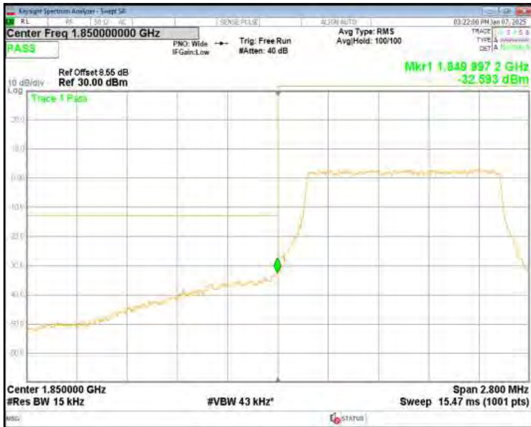
Band2 16QAM BW=1.4MHz Channel=19193 RB Size=6 Position=#0
