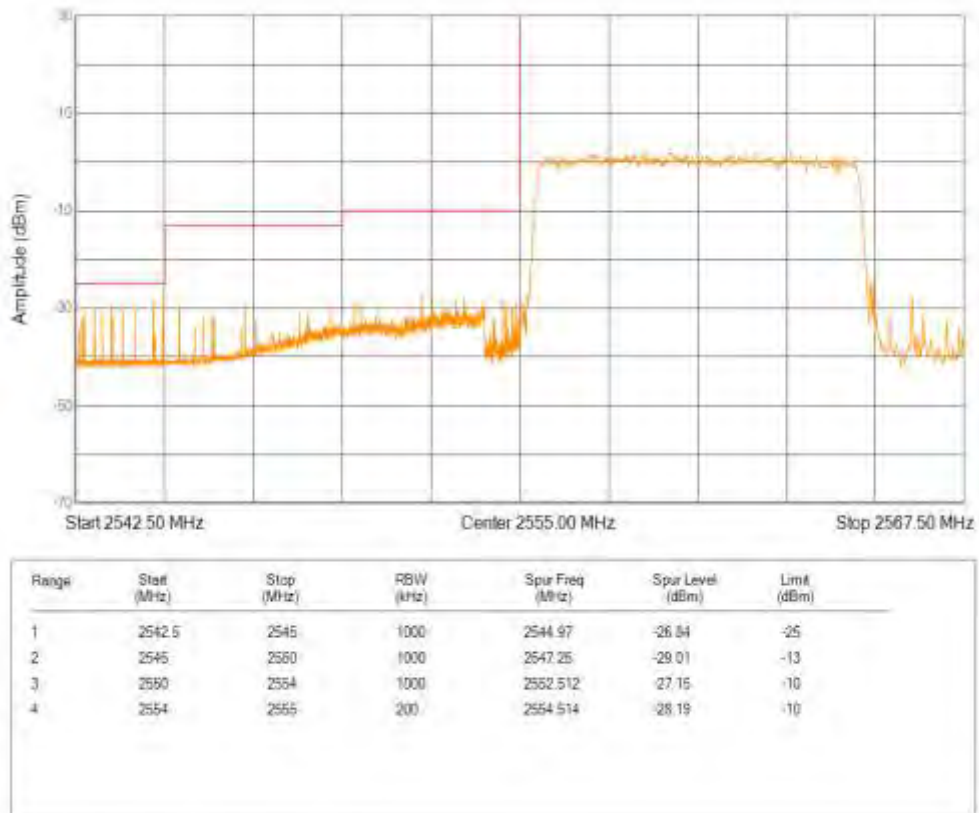
Band41(2555-2655) QPSK BW=10MHz Channel=41190 RB Size=50 Position=#0
