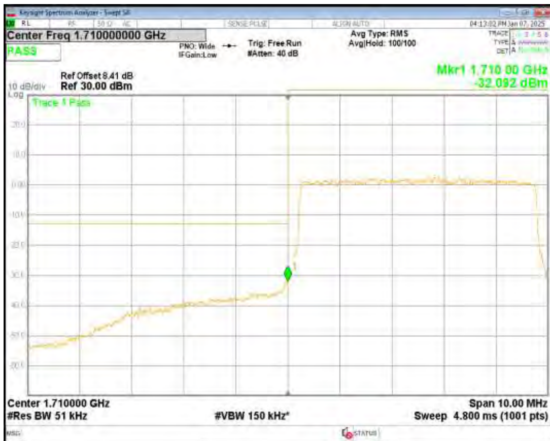
Band4 QPSK BW=1.4MHz Channel=19957 RB Size=6 Position=#0
