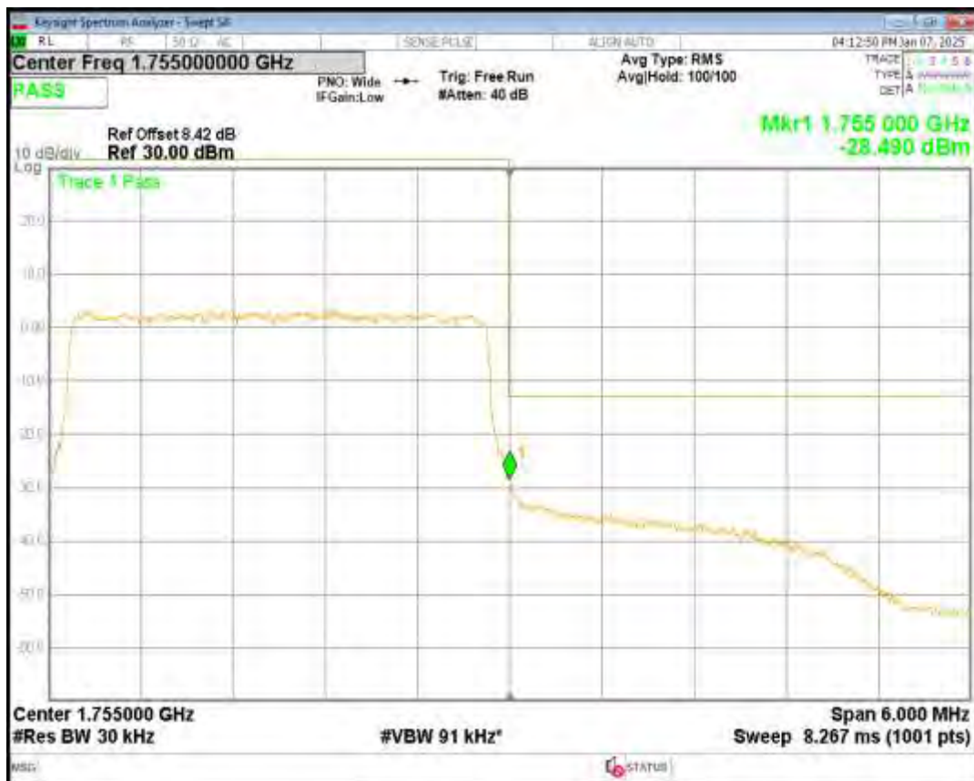
Band4 QPSK BW=5MHz Channel=19975 RB Size=25 Position=#0
