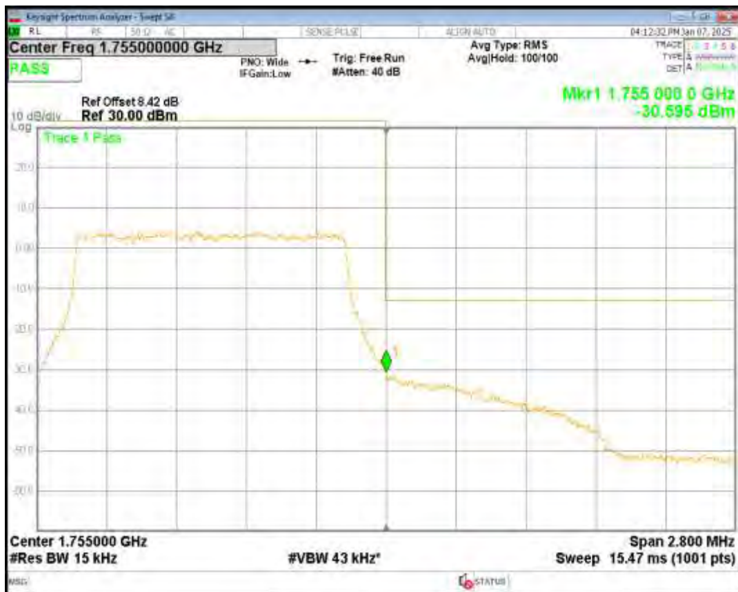
Band4 QPSK BW=10MHz Channel=20000 RB Size=50 Position=#0
