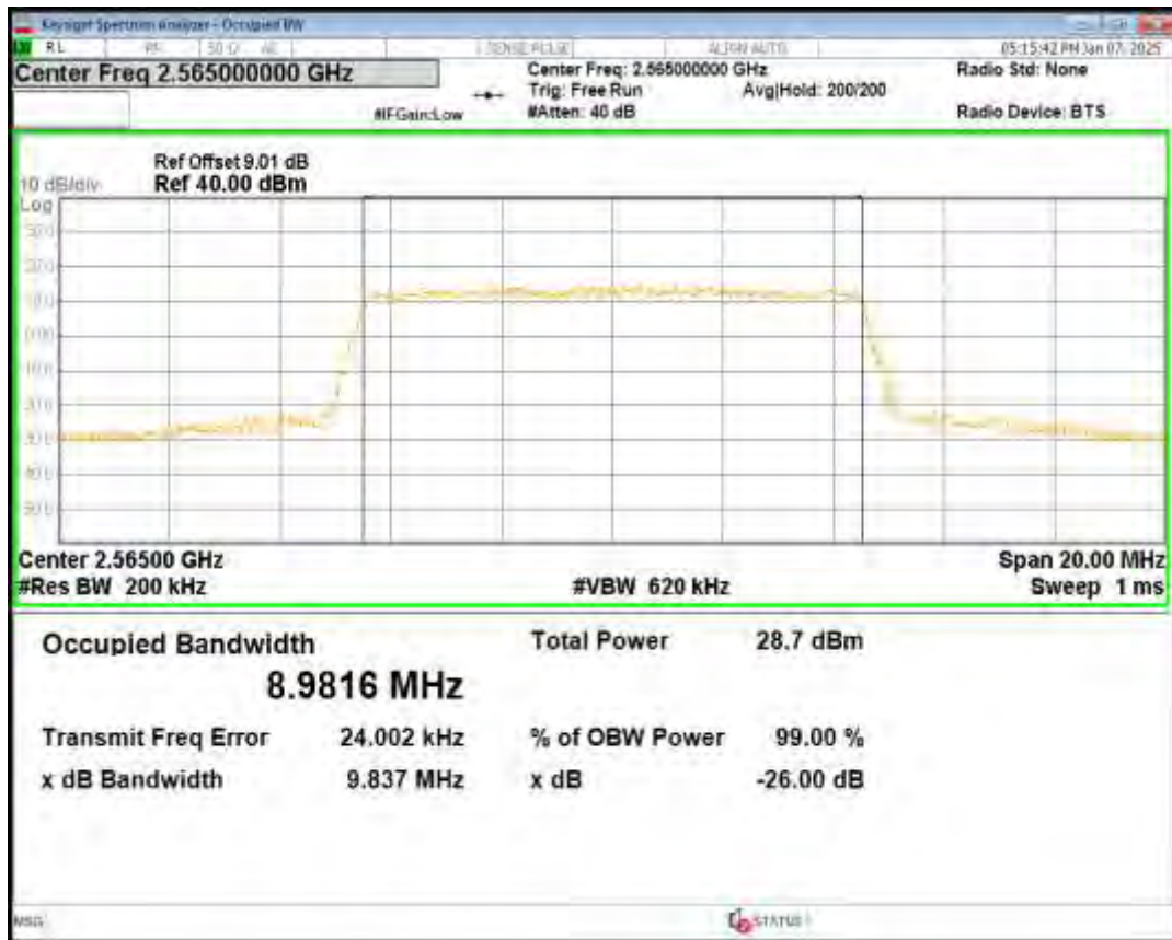
Band7 16QAM BW=15MHz Channel=20825 RB Size=75 Position=#0
