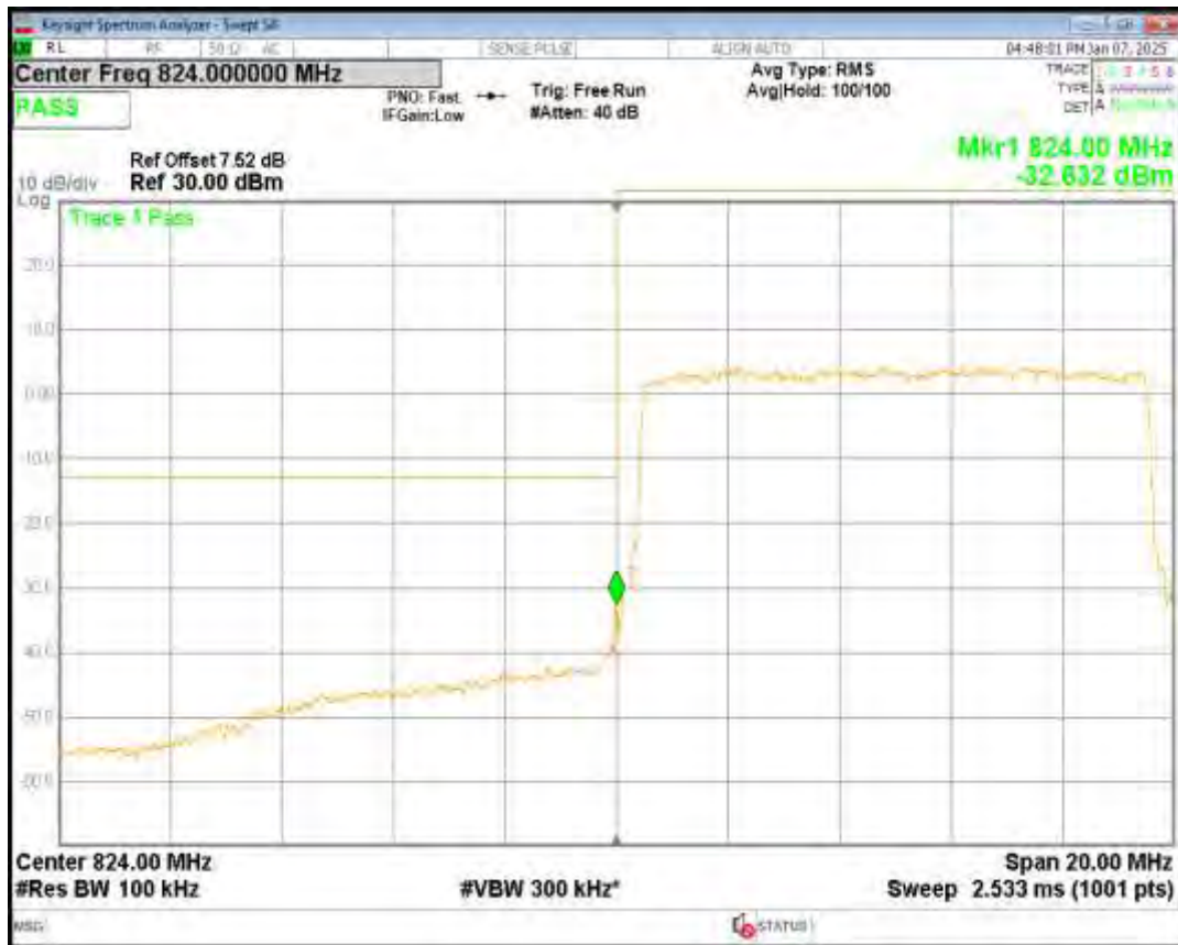
Band5 QPSK BW=10MHz Channel=20600 RB Size=50 Position=#0
