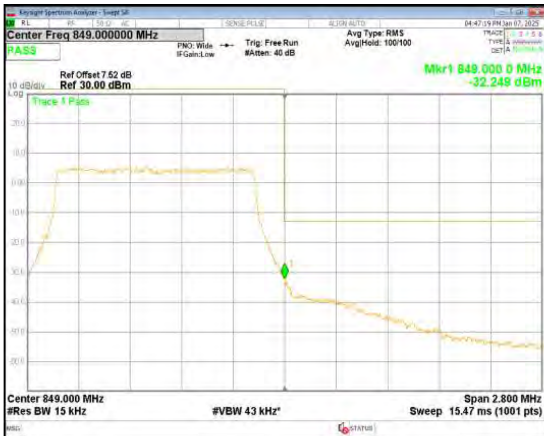
Band5 QPSK BW=10MHz Channel=20450 RB Size=50 Position=#0
