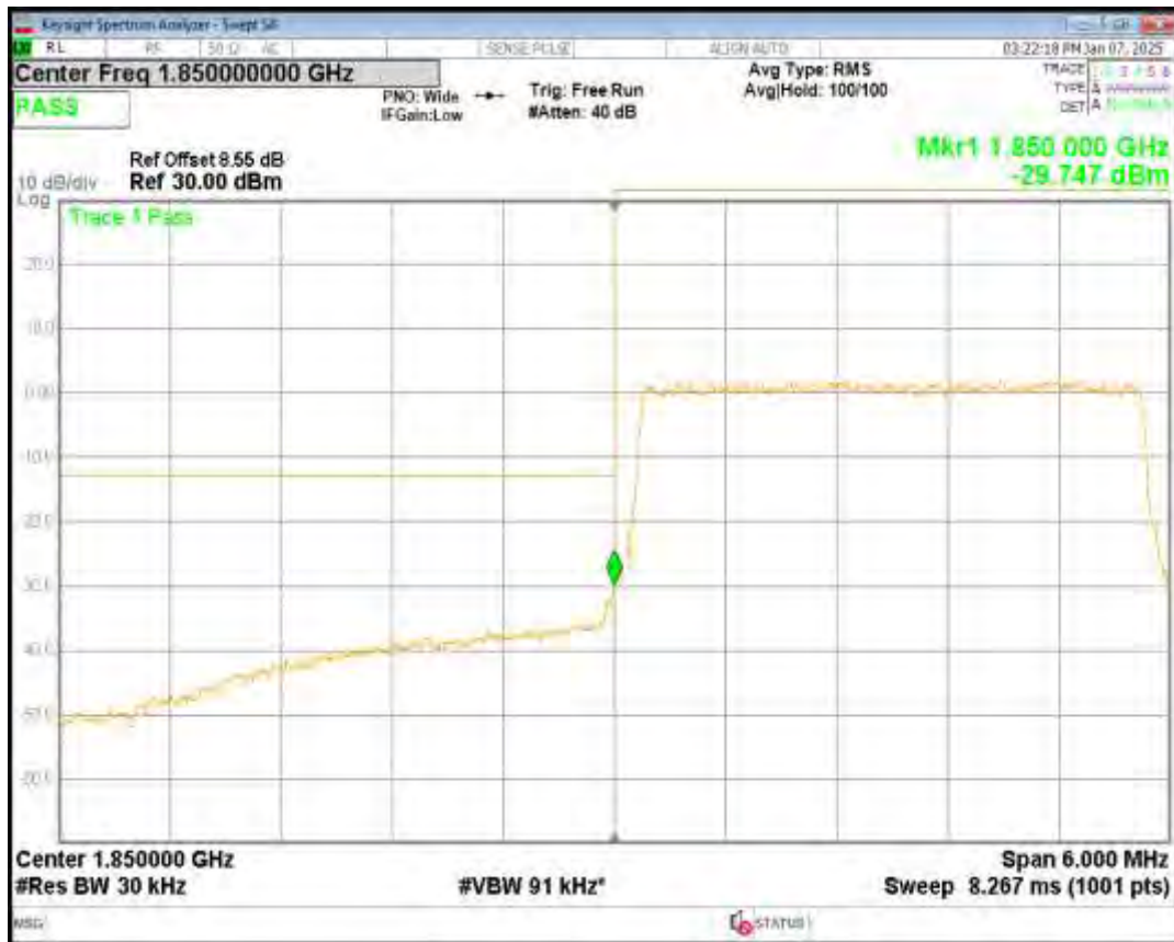
Band2 16QAM BW=3MHz Channel=19185 RB Size=15 Position=#0
