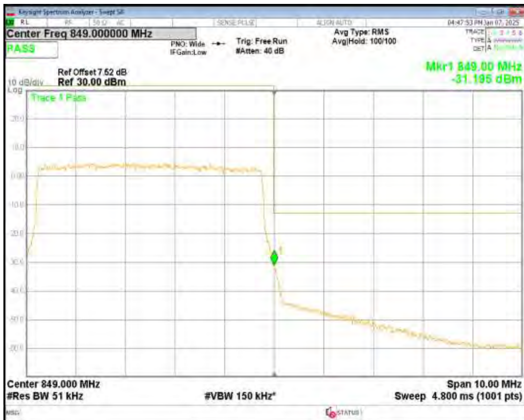
Band7 16QAM BW=10MHz Channel=20800 RB Size=50 Position=#0
