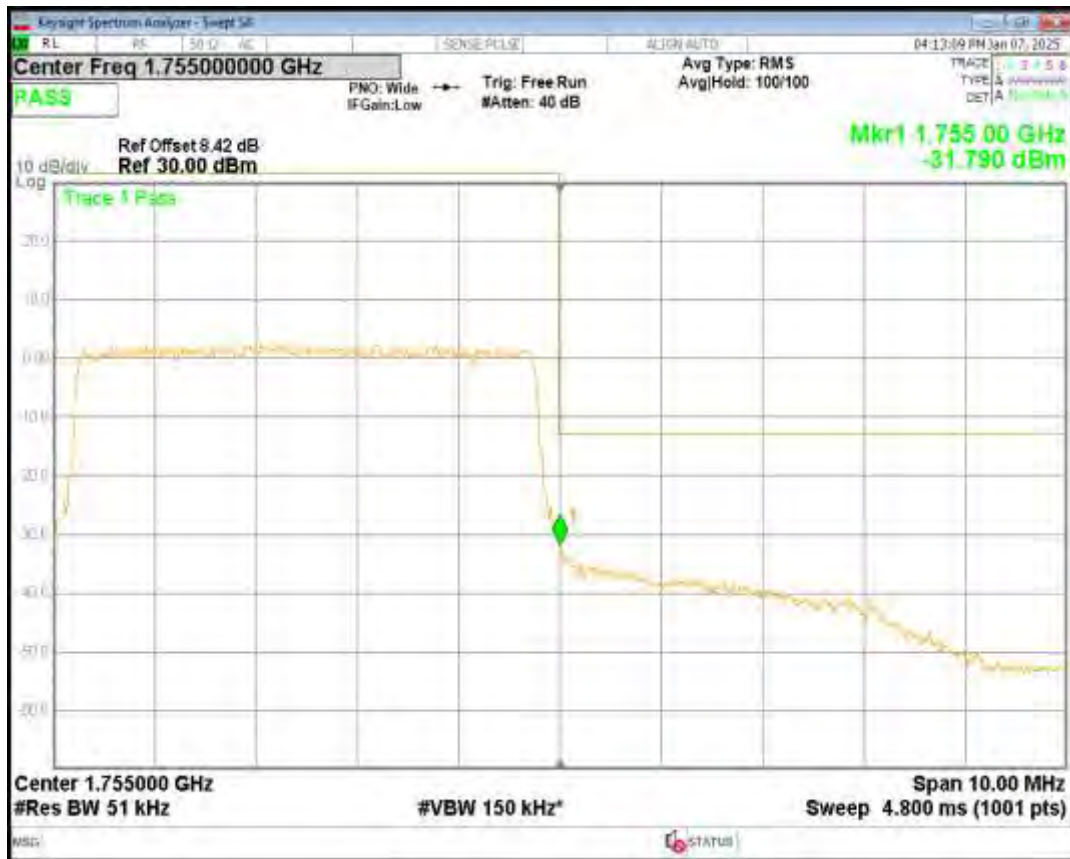
Band4 16QAM BW=5MHz Channel=19975 RB Size=25 Position=#0
