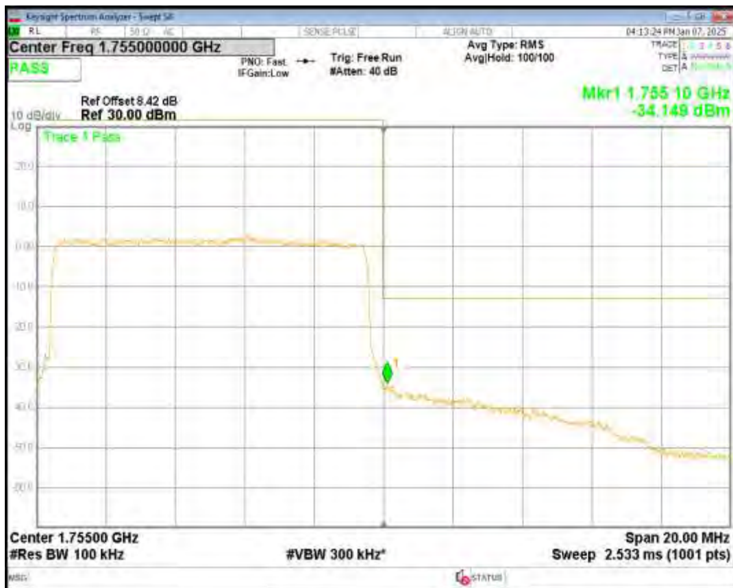
Band4 16QAM BW=15MHz Channel=20025 RB Size=75 Position=#0
