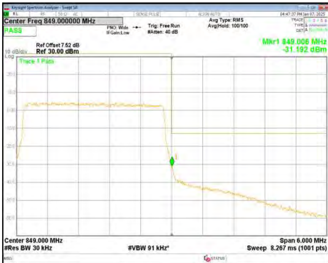
Band5 QPSK BW=5MHz Channel=20425 RB Size=25 Position=#0
