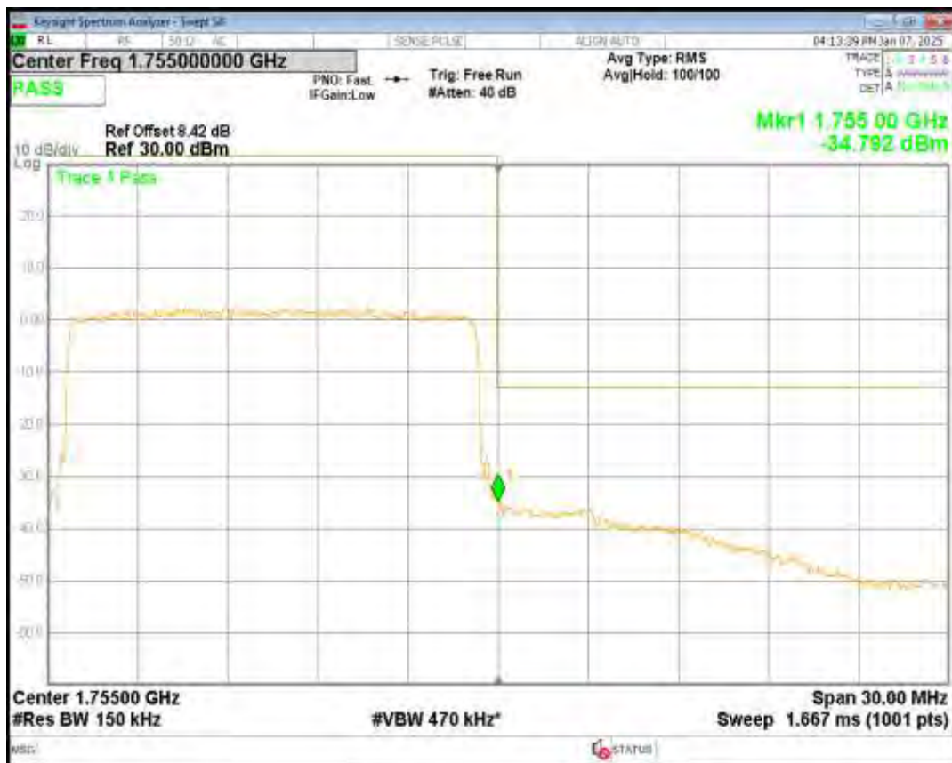
Band4 16QAM BW=20MHz Channel=20050 RB Size=100 Position=#0
