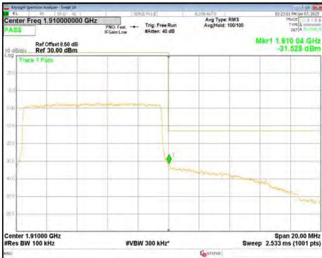
Band2 QPSK BW=15MHz Channel=18675 RB Size=75 Position=#0
