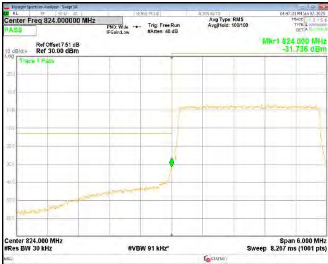
Band5 16QAM BW=3MHz Channel=20635 RB Size=15 Position=#0
