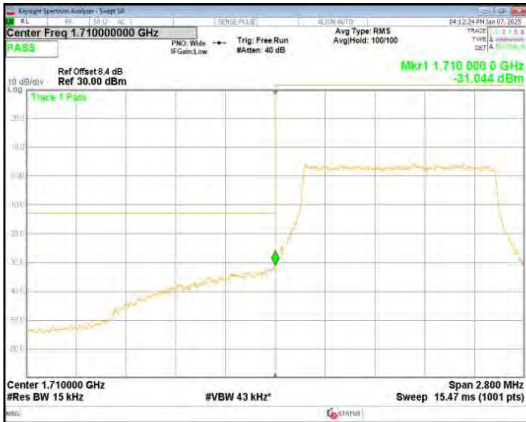
Band4 QPSK BW=1.4MHz Channel=20393 RB Size=6 Position=#0
