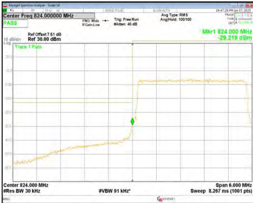
Band5 QPSK BW=3MHz Channel=20635 RB Size=15 Position=#0
