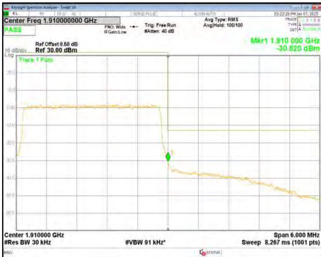
Band2 16QAM BW=5MHz Channel=18625 RB Size=25 Position=#0
