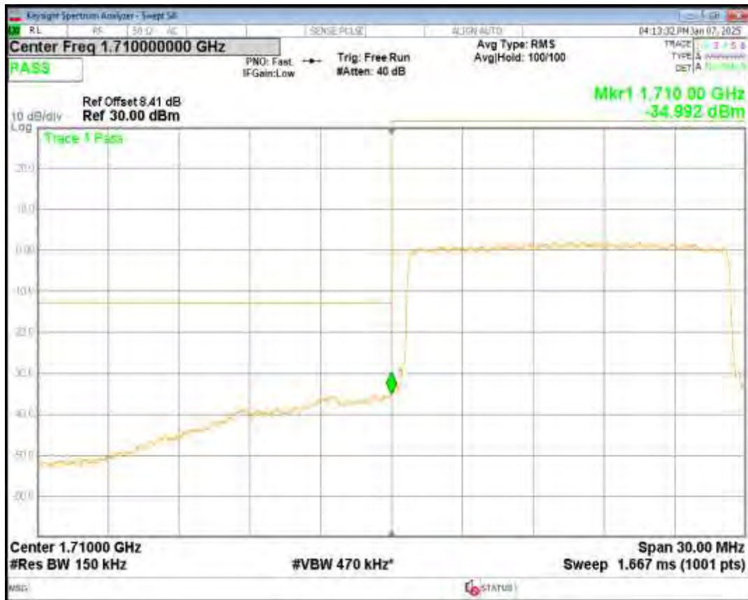
Band4 16QAM BW=15MHz Channel=20325 RB Size=75 Position=#0
