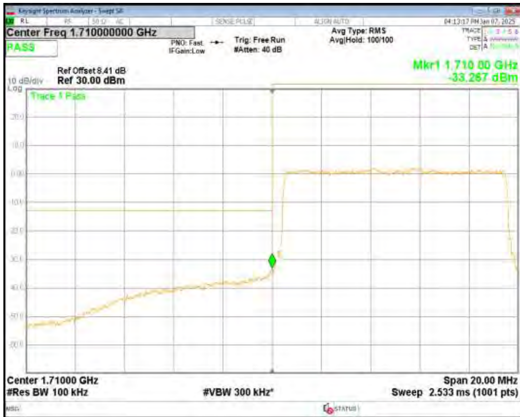
Band4 16QAM BW=10MHz Channel=20350 RB Size=50 Position=#0
