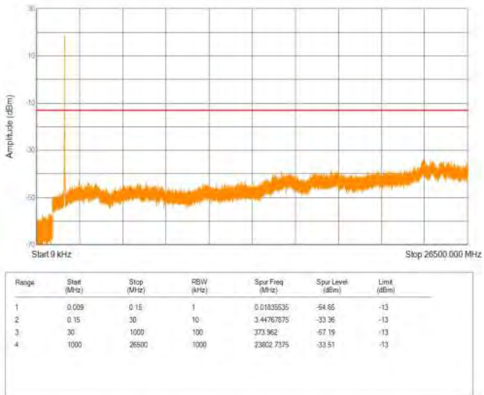
Band4 16QAM BW=20MHz Channel=20050 RB Size=100 Position=#0
