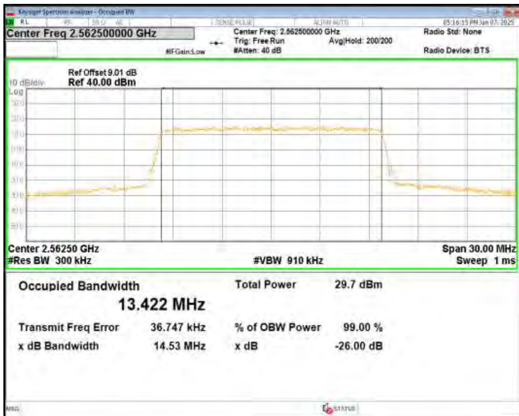
Band7 QPSK BW=15MHz Channel=21100 RB Size=75 Position=#0
