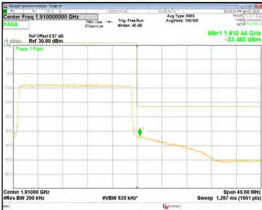
Band2 QPSK BW=3MHz Channel=18615 RB Size=15 Position=#0
