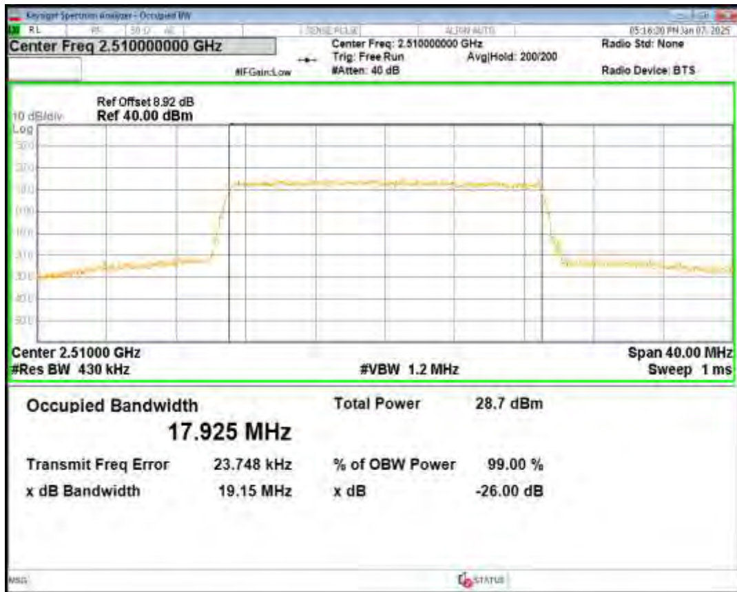
Band7 16QAM BW=20MHz Channel=21100 RB Size=100 Position=#0
