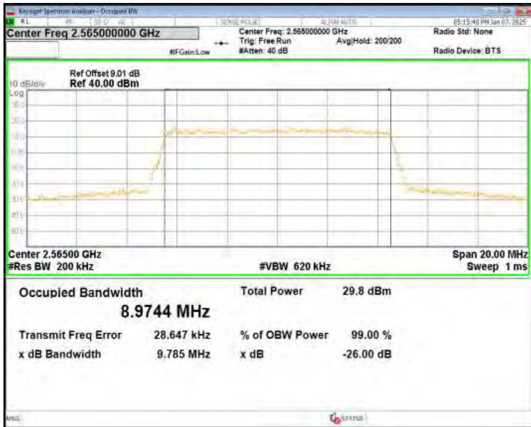
Band7 16QAM BW=5MHz Channel=21425 RB Size=25 Position=#0
