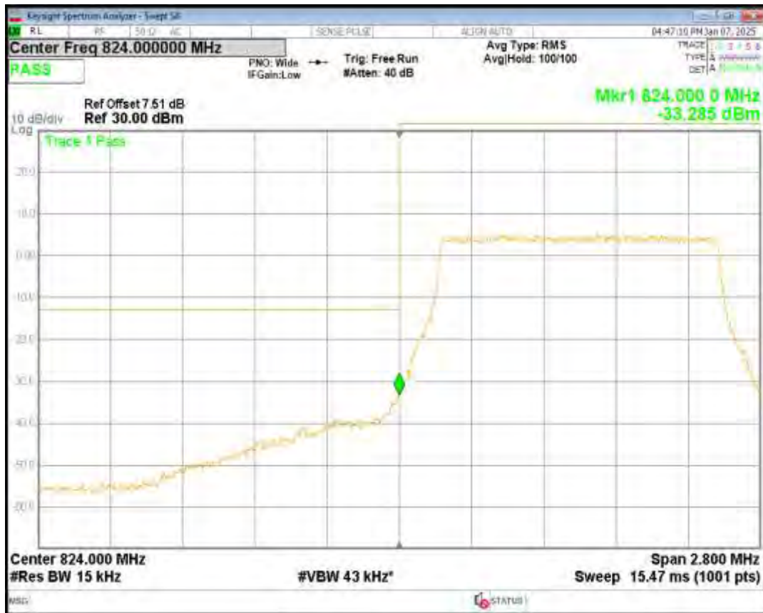
Band5 QPSK BW=1.4MHz Channel=20643 RB Size=6 Position=#0
