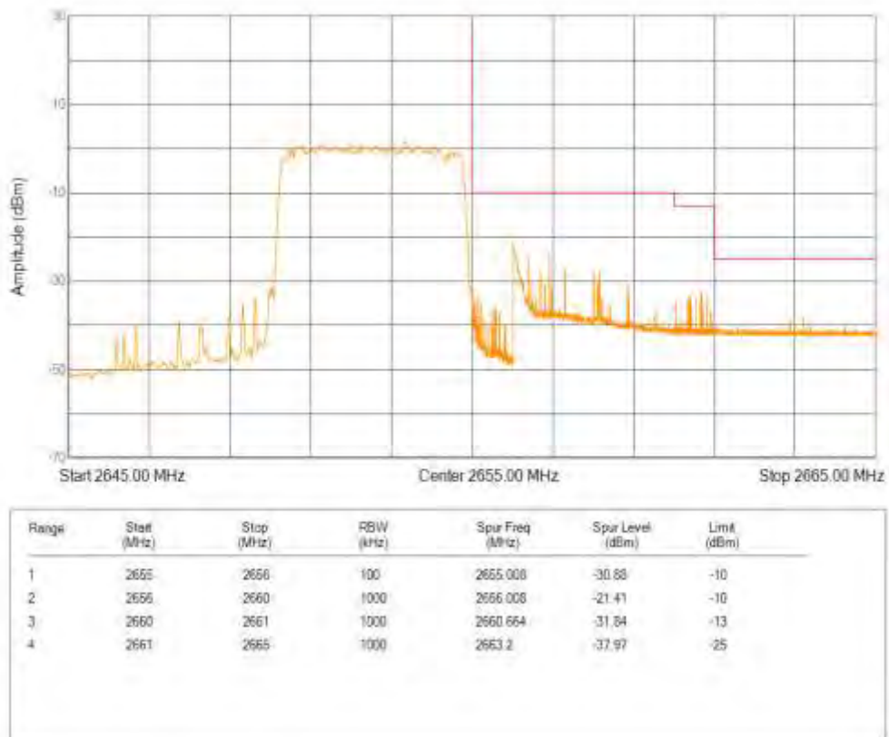
Band41(2555-2655) QPSK BW=10MHz Channel=40290 RB Size=50 Position=#0
