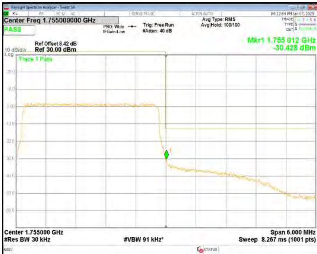
Band4 16QAM BW=5MHz Channel=20375 RB Size=25 Position=#0
