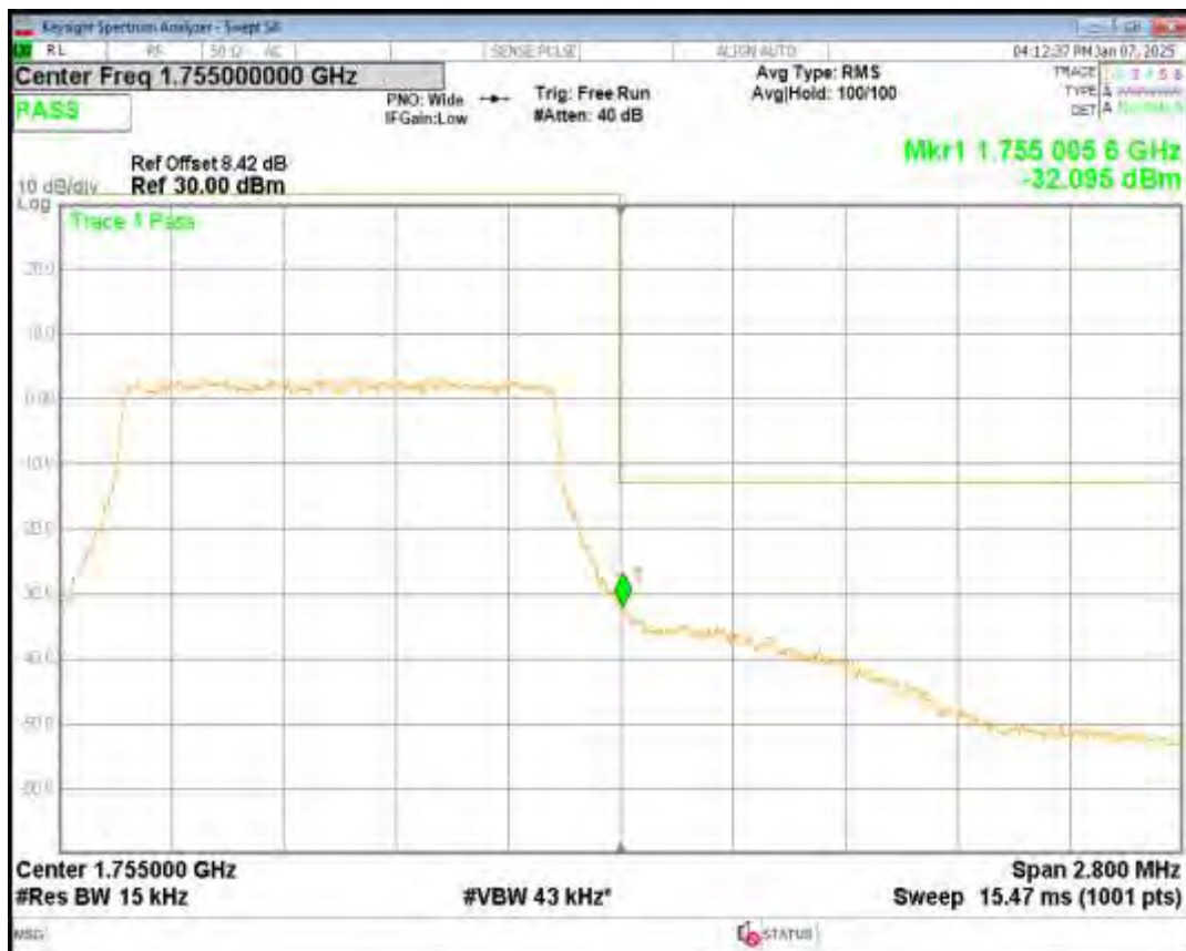
Band4 16QAM BW=10MHz Channel=20000 RB Size=50 Position=#0
