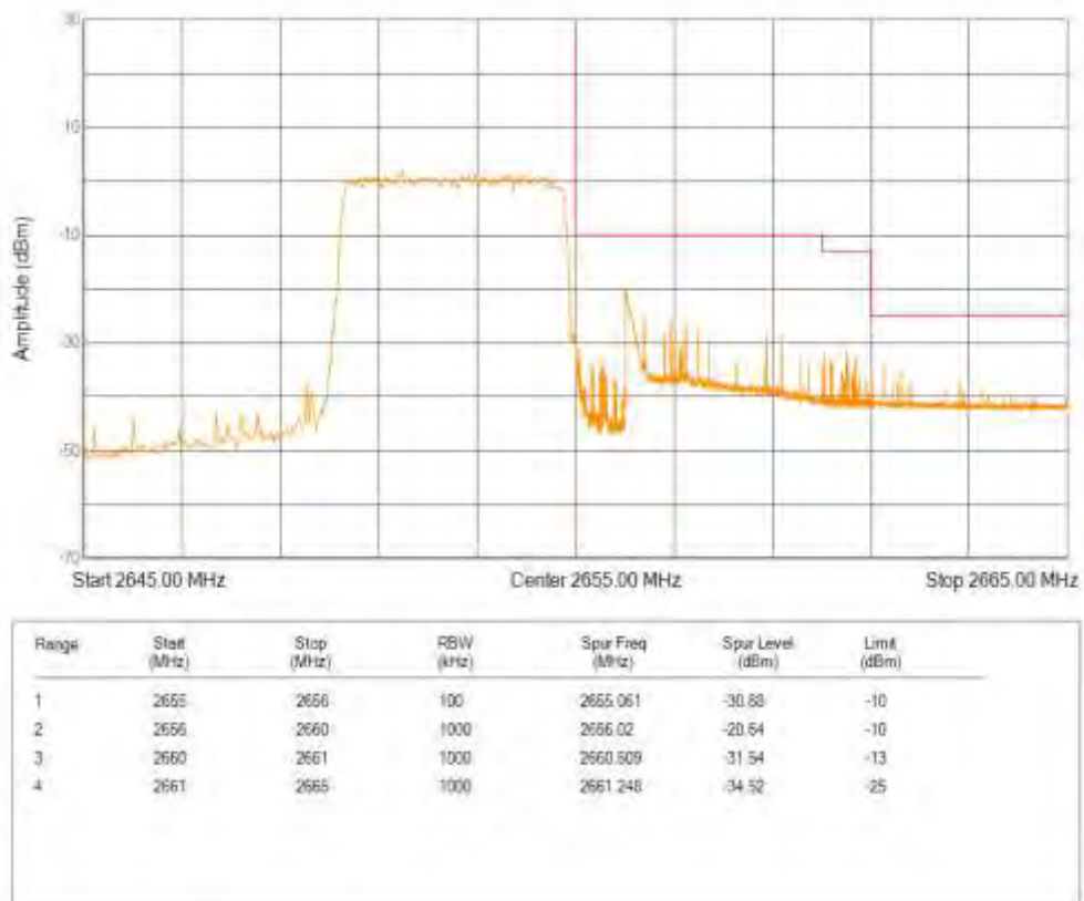
Band5 16QAM BW=1.4MHz Channel=20407 RB Size=6 Position=#0
