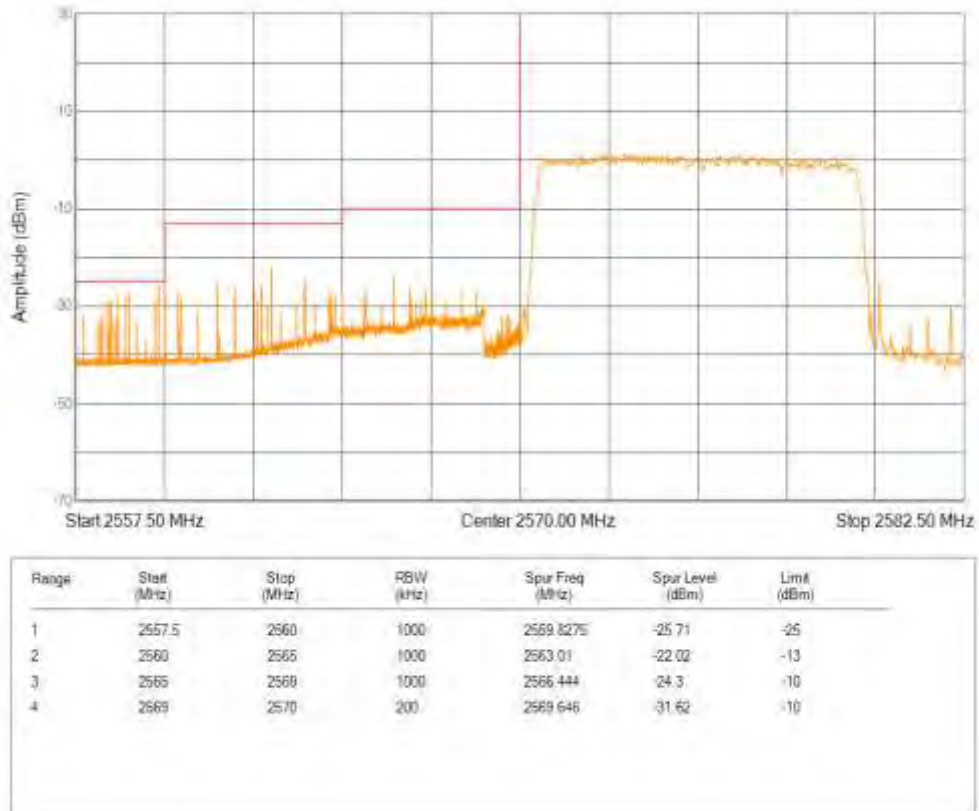
Band38 16QAM BW=10MHz Channel=38200 RB Size=50 Position=#0
