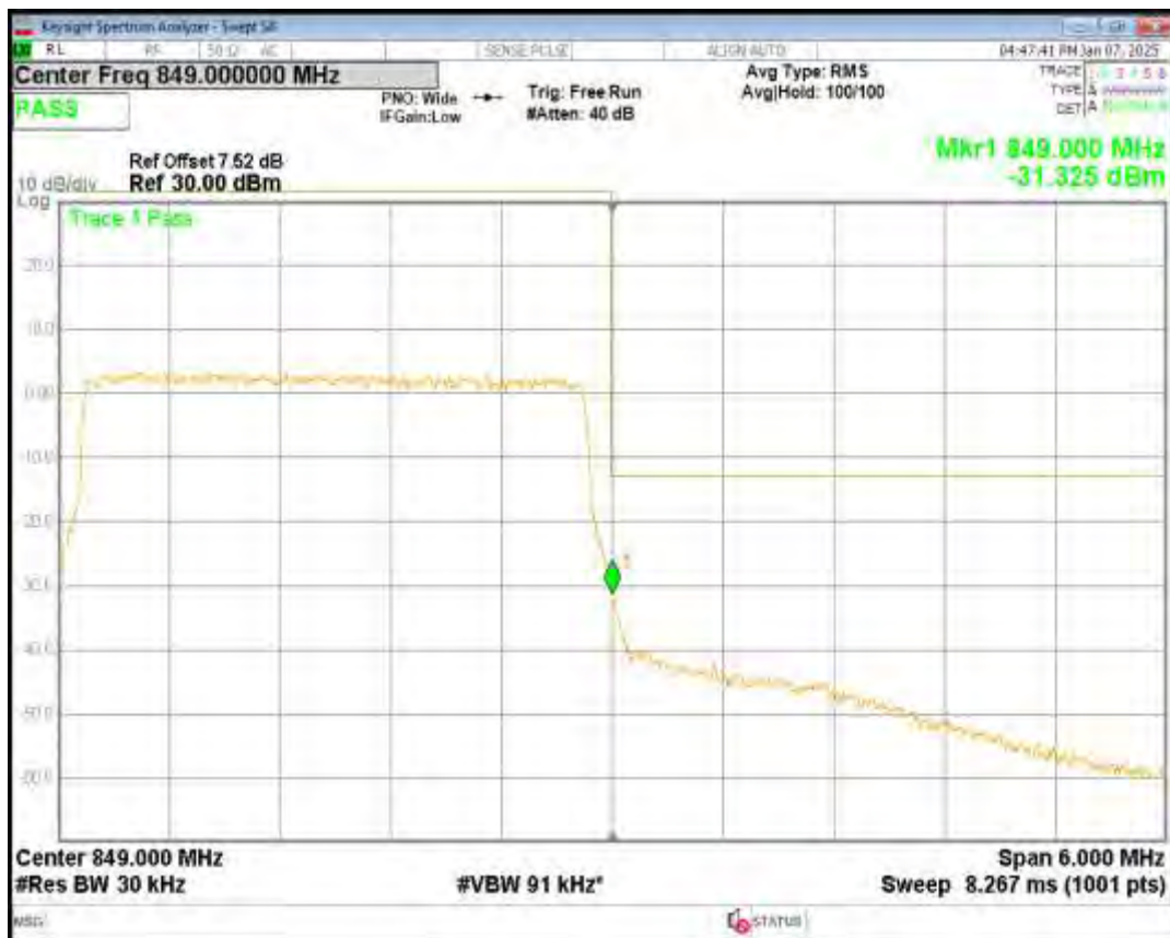
Band5 16QAM BW=5MHz Channel=20425 RB Size=25 Position=#0
