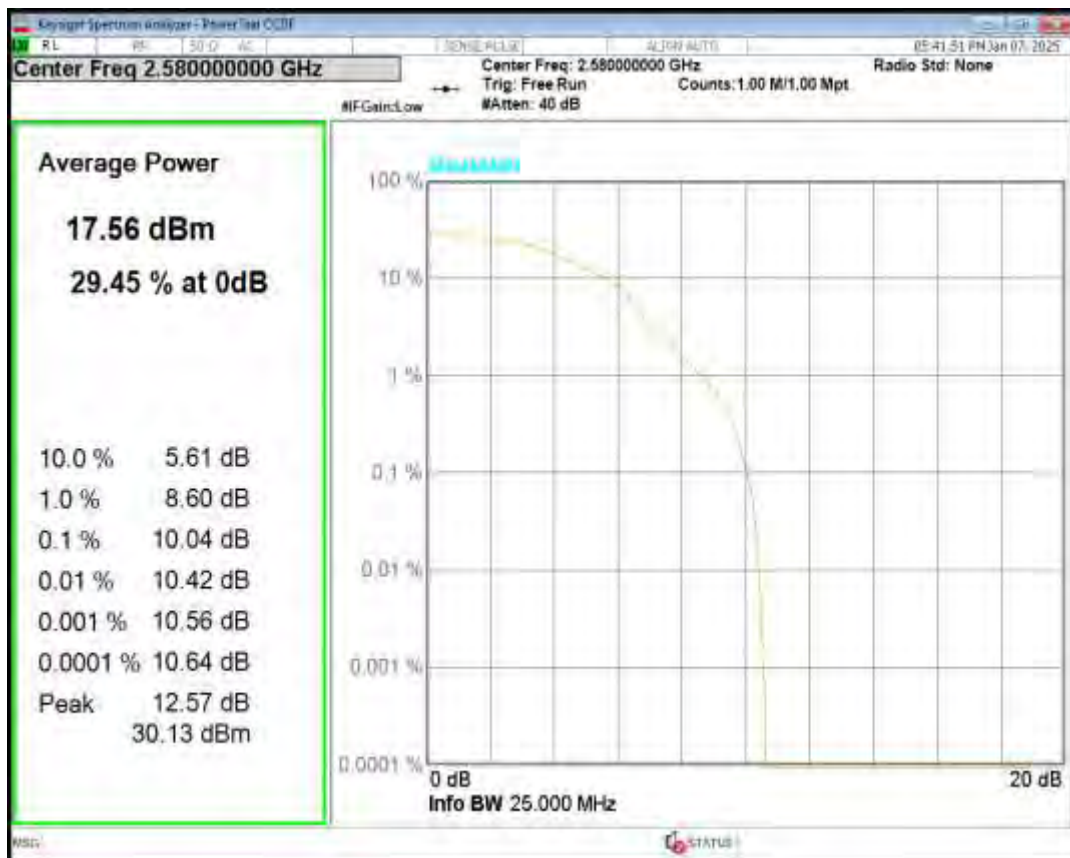
Band38 16QAM BW=20MHz Channel=38000 RB Size=1 Position=#0
