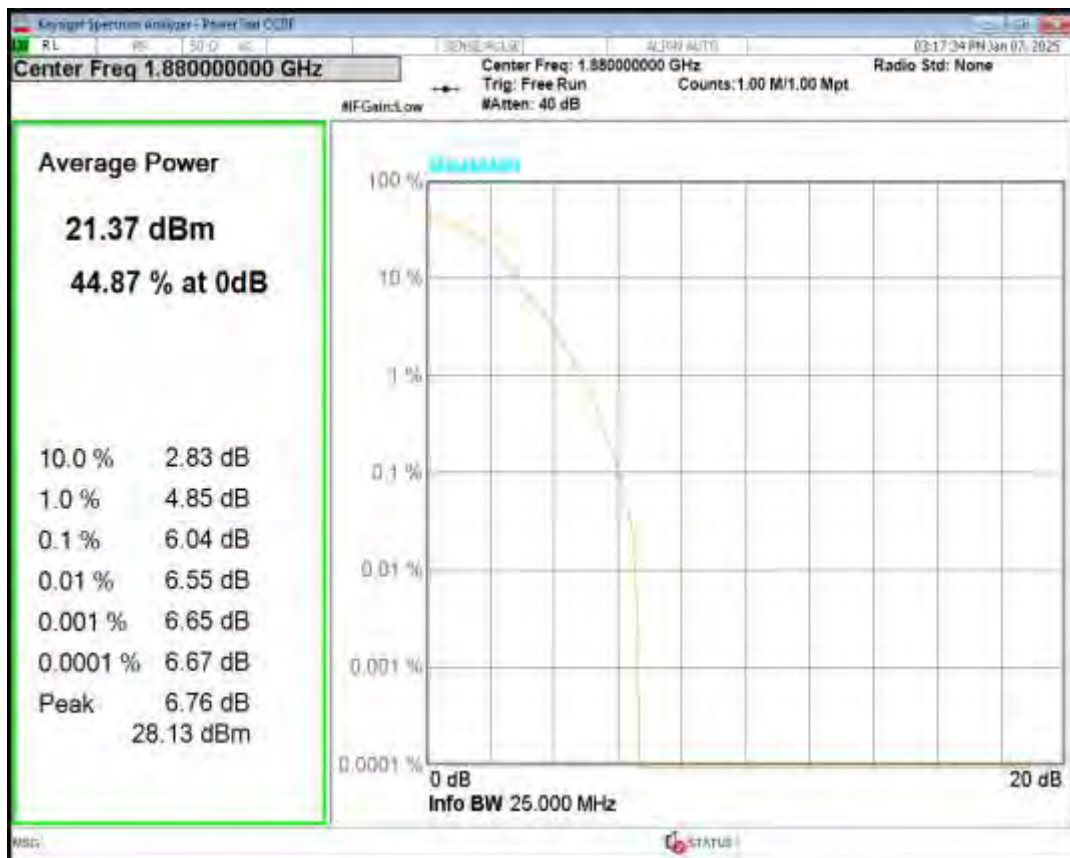
Band2 16QAM BW=15MHz Channel=18675 RB Size=1 Position=#0
