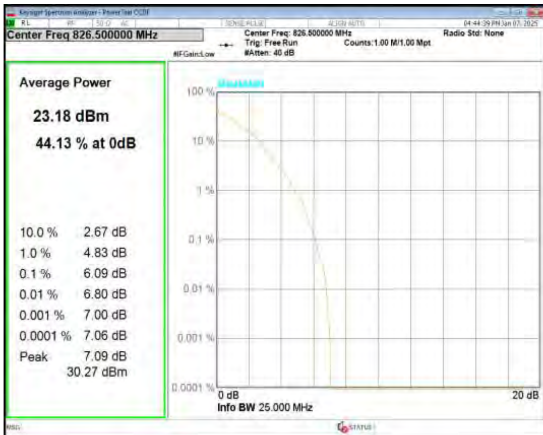
Band5 QPSK BW=5MHz Channel=20625 RB Size=1 Position=#0
