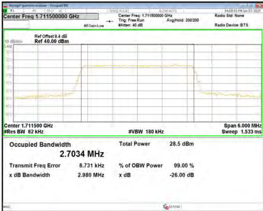
Band4 16QAM BW=3MHz Channel=20175 RB Size=15 Position=#0
