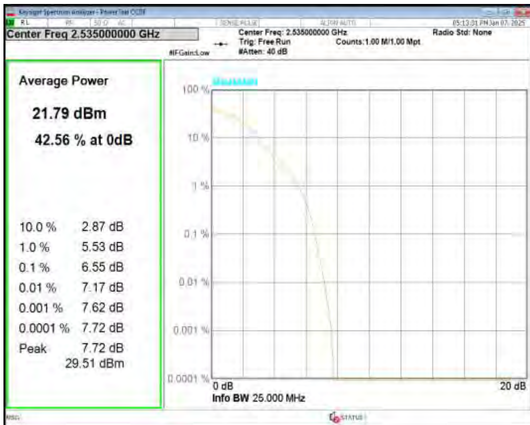
Band7 16QAM BW=5MHz Channel=20775 RB Size=1 Position=#0
