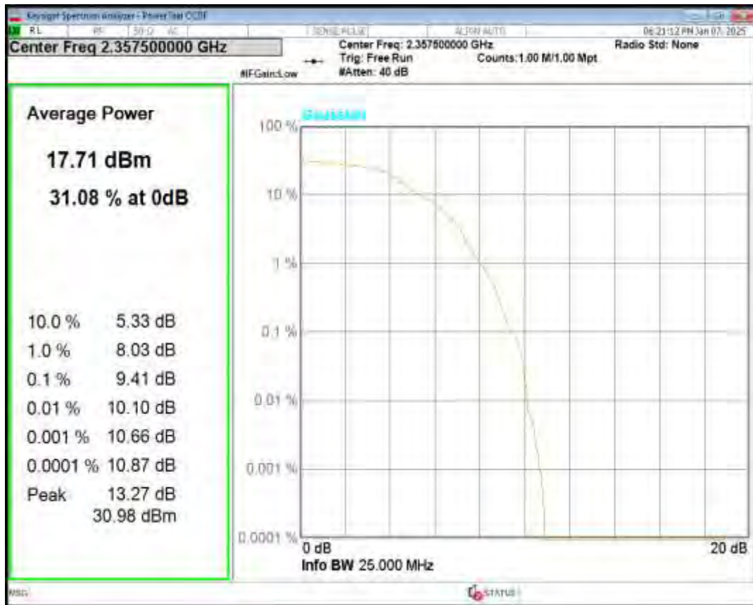
Band41(2555-2655) 16QAM BW=10MHz Channel=40290 RB Size=1 Position=#0
