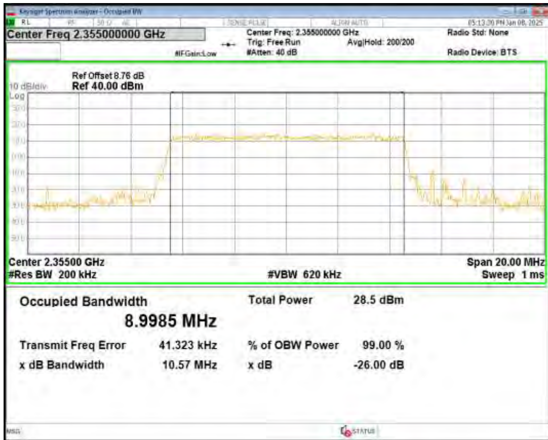
Band40(2350-2360) QPSK BW=5MHz Channel=39175 RB Size=25 Position=#0
