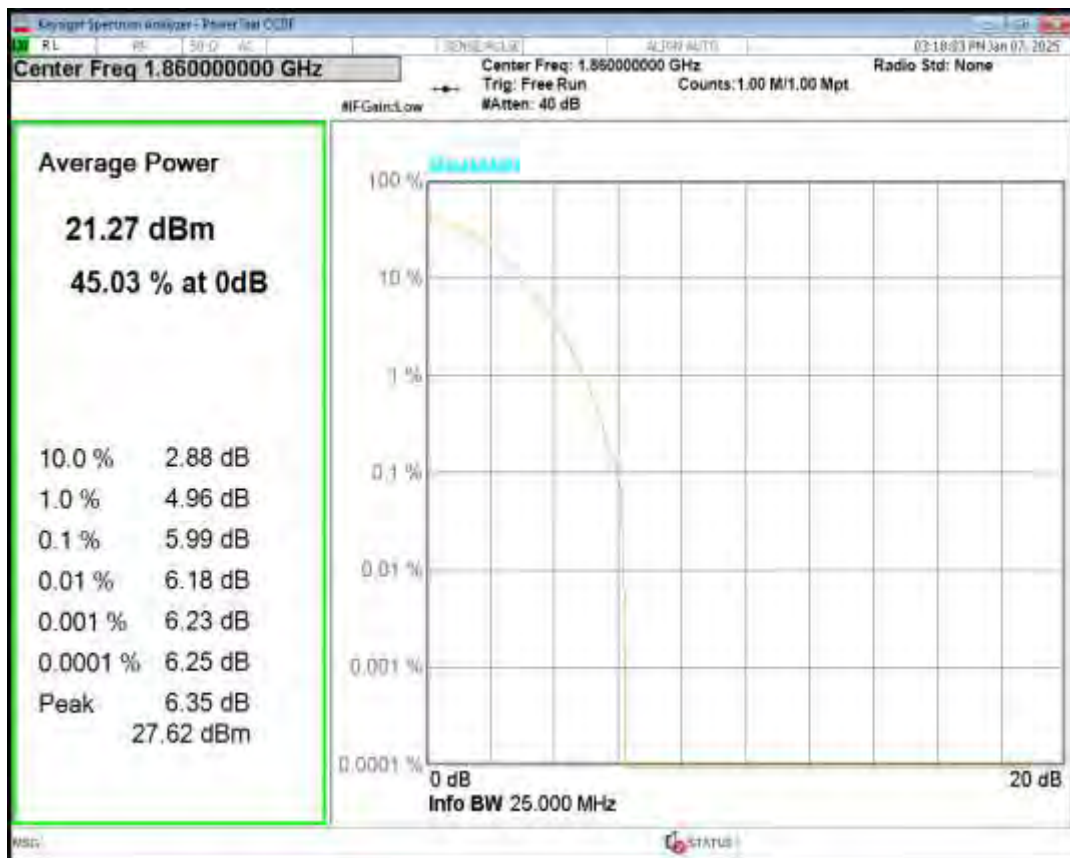
Band2 16QAM BW=15MHz Channel=19125 RB Size=1 Position=#0
