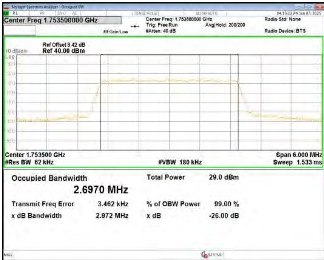
Band4 16QAM BW=5MHz Channel=19975 RB Size=25 Position=#0
