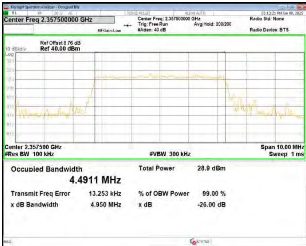
Band41(2555-2655) 16QAM BW=10MHz Channel=40290 RB Size=50 Position=#0
