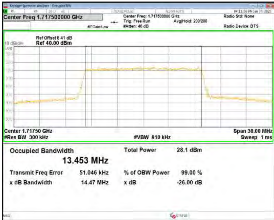
Band4 16QAM BW=15MHz Channel=20175 RB Size=75 Position=#0
