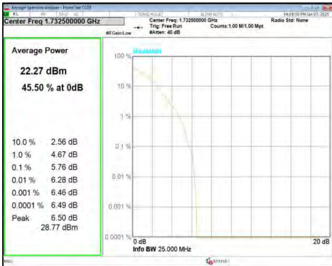
Band4 QPSK BW=15MHz Channel=20325 RB Size=1 Position=#0
