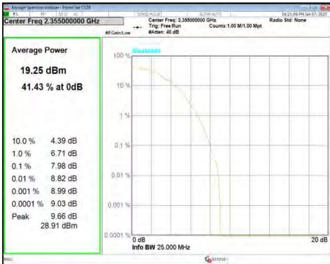
Band40(2350-2360) QPSK BW=5MHz Channel=39225 RB Size=1 Position=#0
