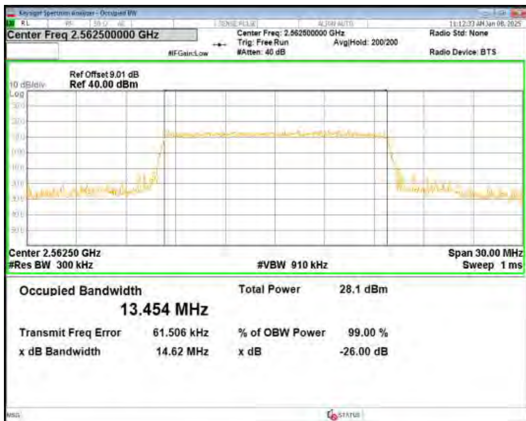
Band41(2555-2655) QPSK BW=15MHz Channel=40740 RB Size=75 Position=#0
