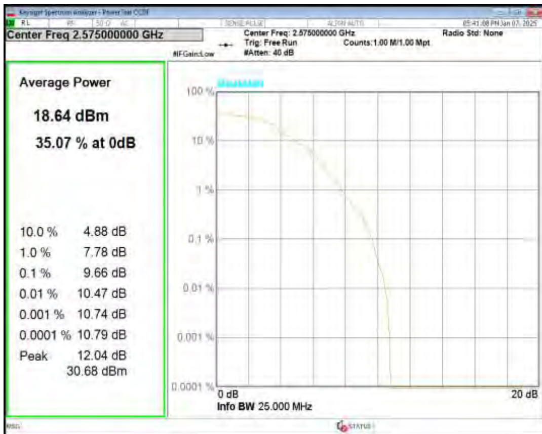
Band38 QPSK BW=10MHz Channel=38000 RB Size=1 Position=#0
