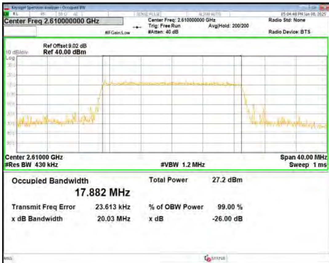
Band38 16QAM BW=5MHz Channel=38225 RB Size=25 Position=#0
