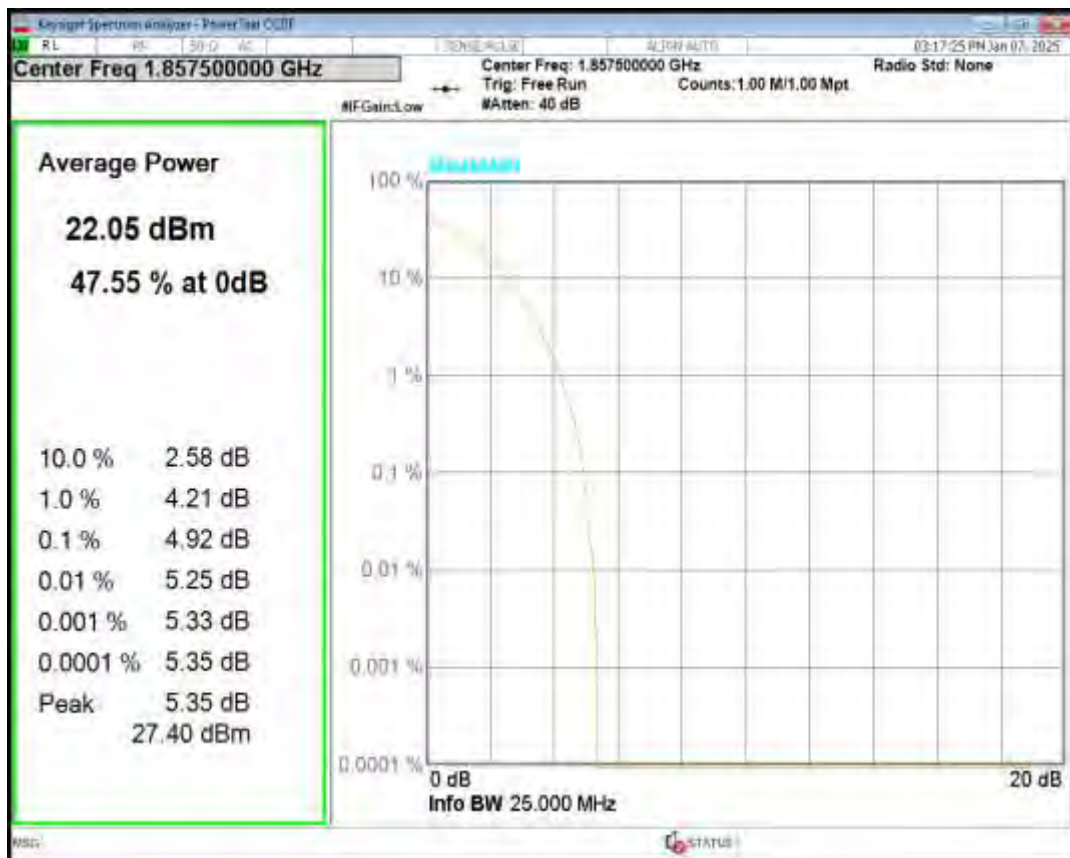
Band2 QPSK BW=15MHz Channel=18900 RB Size=1 Position=#0
