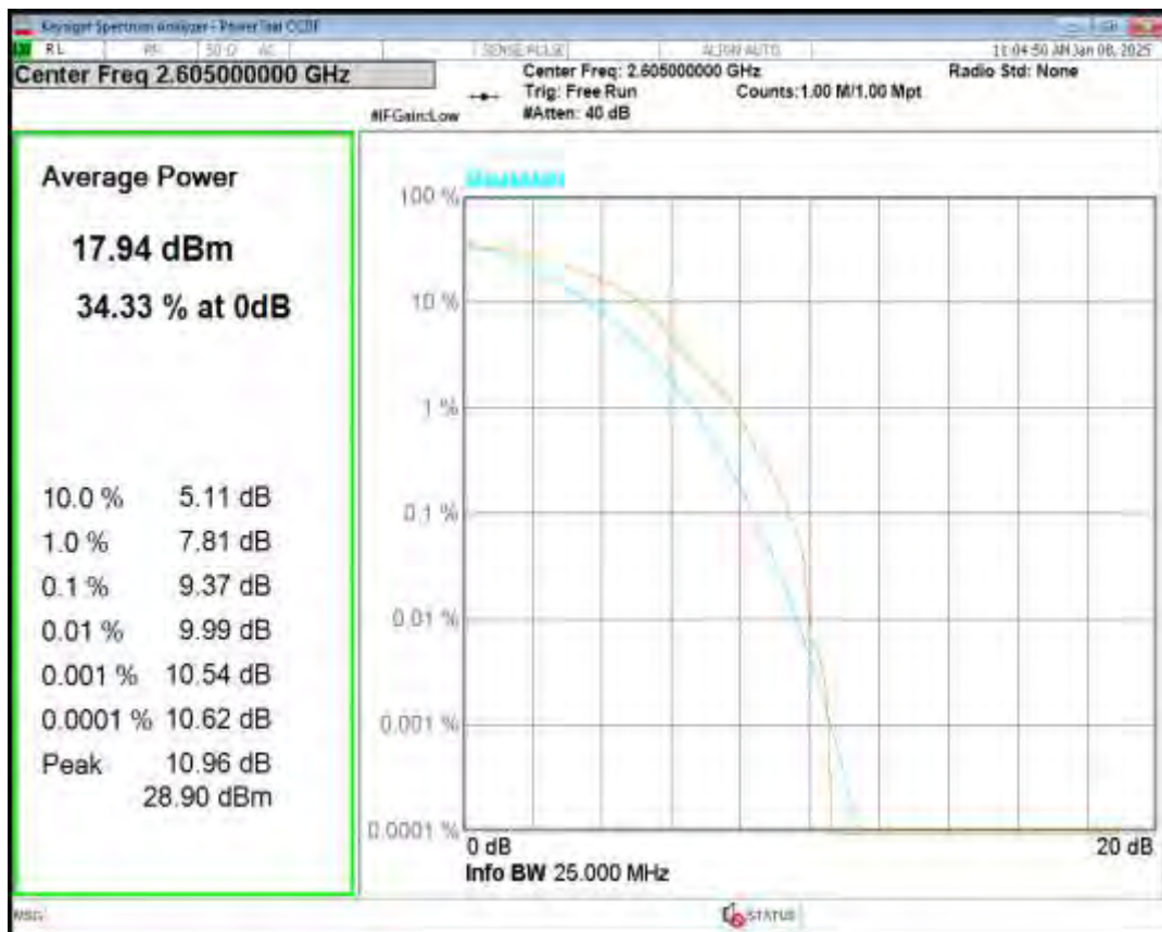
Band41(2555-2655) 16QAM BW=20MHz Channel=40740 RB Size=1 Position=#0
