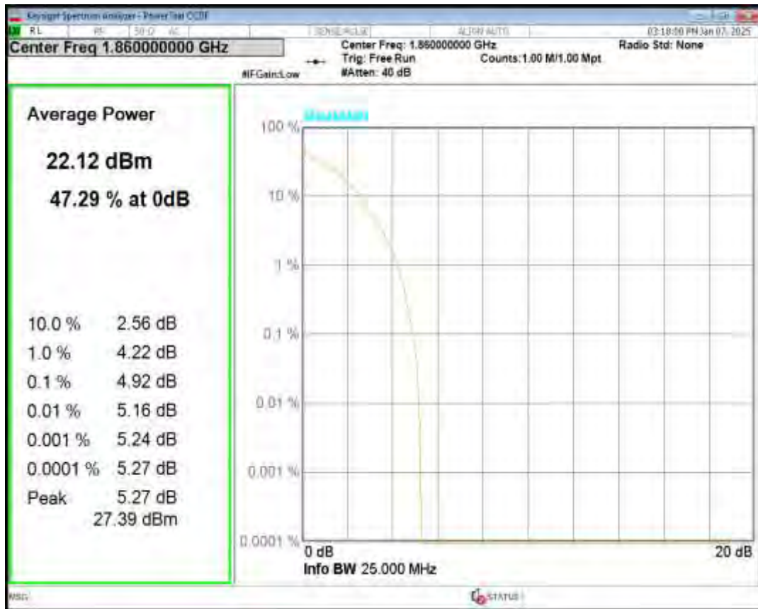
Band2 QPSK BW=20MHz Channel=18900 RB Size=1 Position=#0
