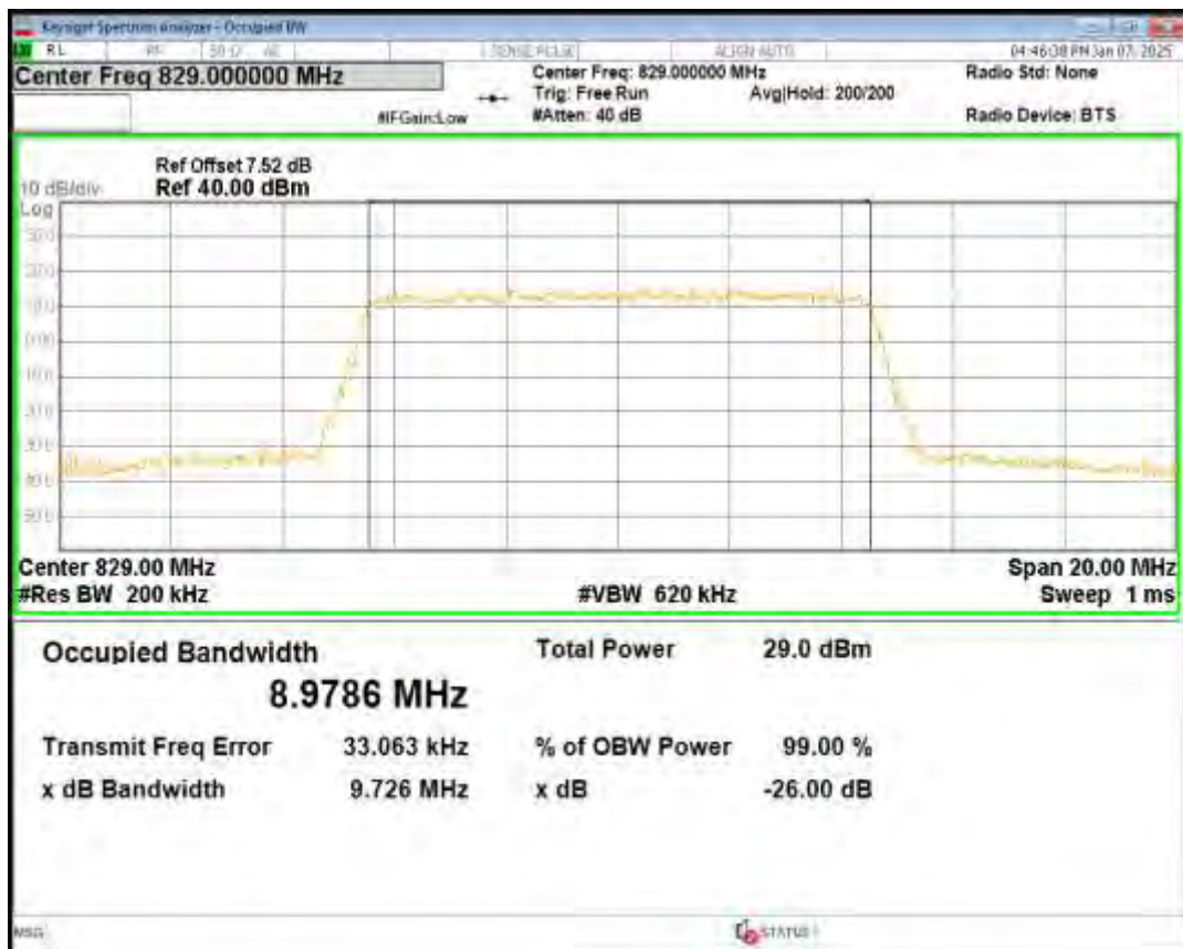
Band5 16QAM BW=10MHz Channel=20525 RB Size=50 Position=#0
