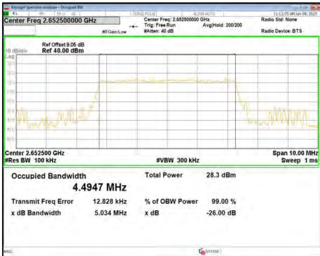
Band5 16QAM BW=1.4MHz Channel=20407 RB Size=6 Position=#0
