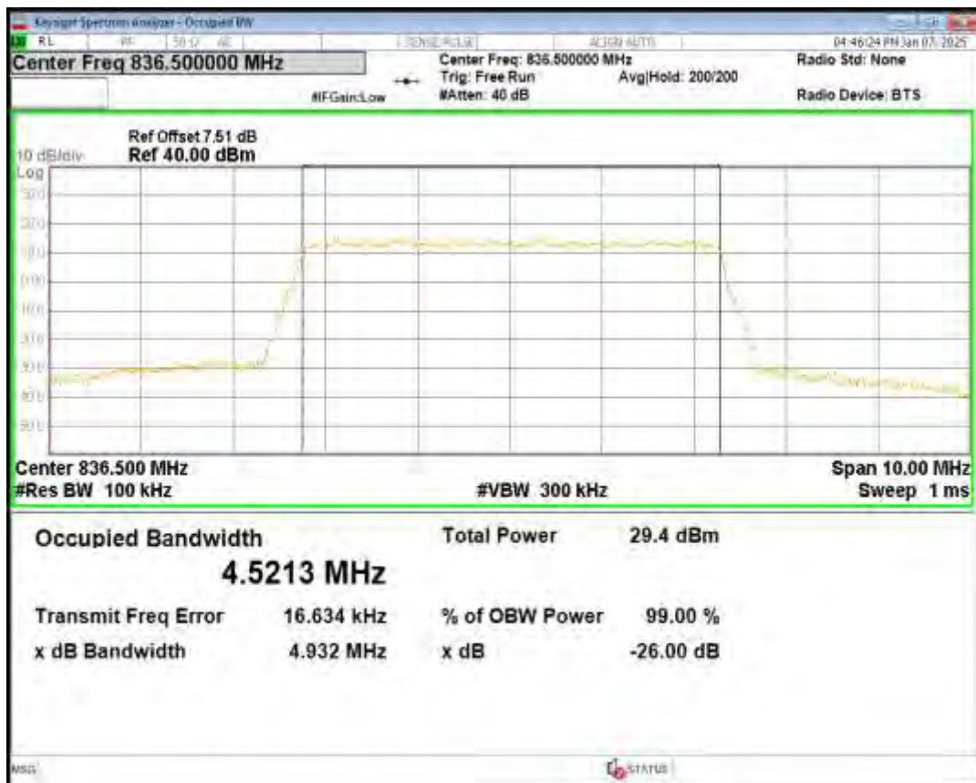
Band5 QPSK BW=1.4MHz Channel=20643 RB Size=6 Position=#0
