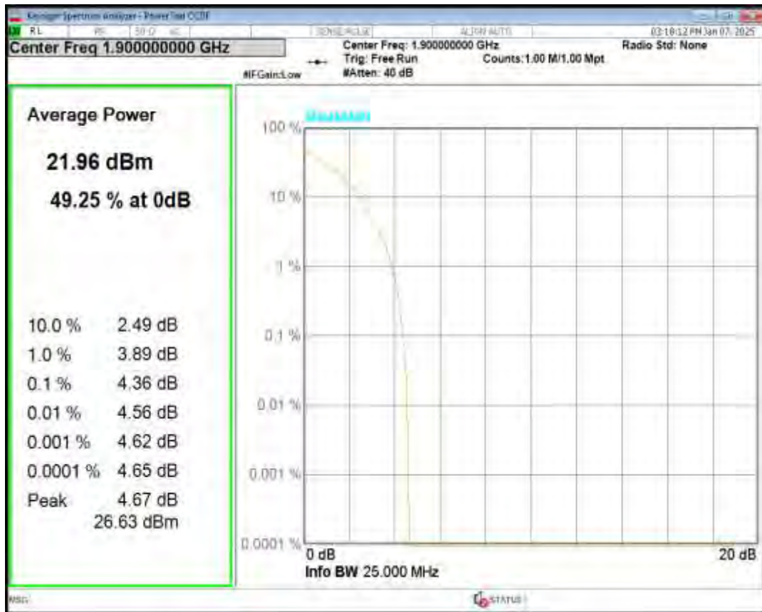
Band2 QPSK BW=3MHz Channel=18615 RB Size=1 Position=#0
