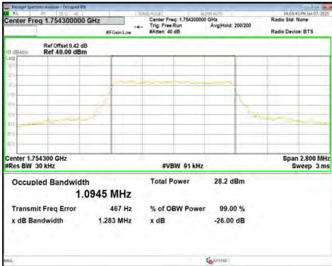
Band4 16QAM BW=10MHz Channel=20000 RB Size=50 Position=#0
