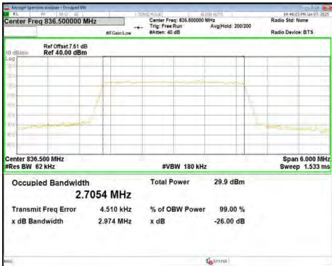
Band5 16QAM BW=3MHz Channel=20635 RB Size=15 Position=#0
