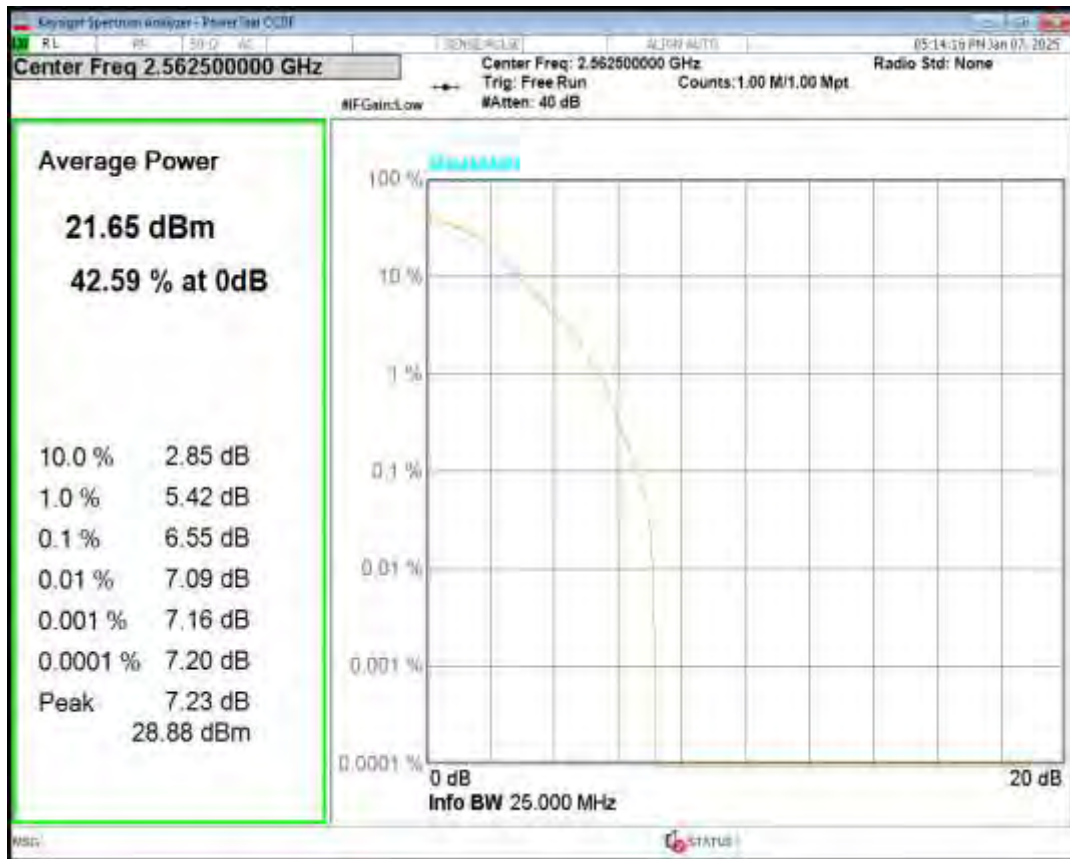
Band7 16QAM BW=15MHz Channel=21100 RB Size=1 Position=#0
