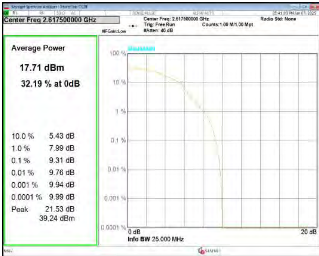
Band38 QPSK BW=10MHz Channel=37800 RB Size=1 Position=#0
