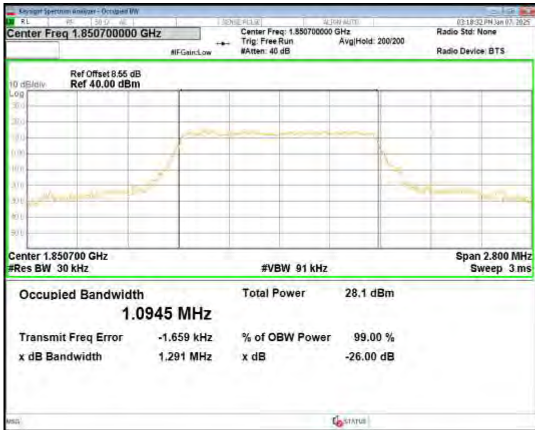
Band2 16QAM BW=1.4MHz Channel=18900 RB Size=6 Position=#0
