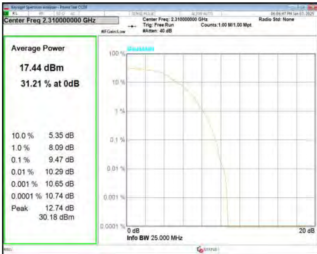
Band40(2305-2315) QPSK BW=5MHz Channel=38775 RB Size=1 Position=#0
