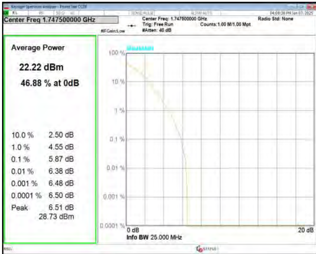
Band4 QPSK BW=15MHz Channel=20175 RB Size=1 Position=#0
