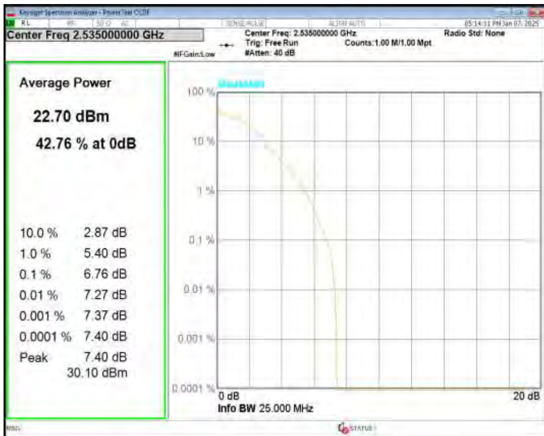
Band7 16QAM BW=20MHz Channel=21100 RB Size=1 Position=#0
