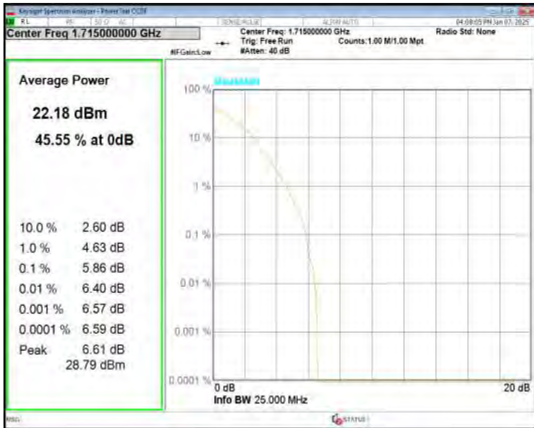
Band4 QPSK BW=10MHz Channel=20175 RB Size=1 Position=#0
