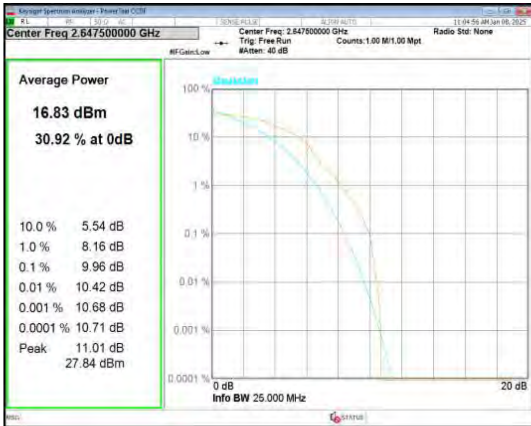
Band41(2555-2655) 16QAM BW=15MHz Channel=40740 RB Size=1 Position=#0
