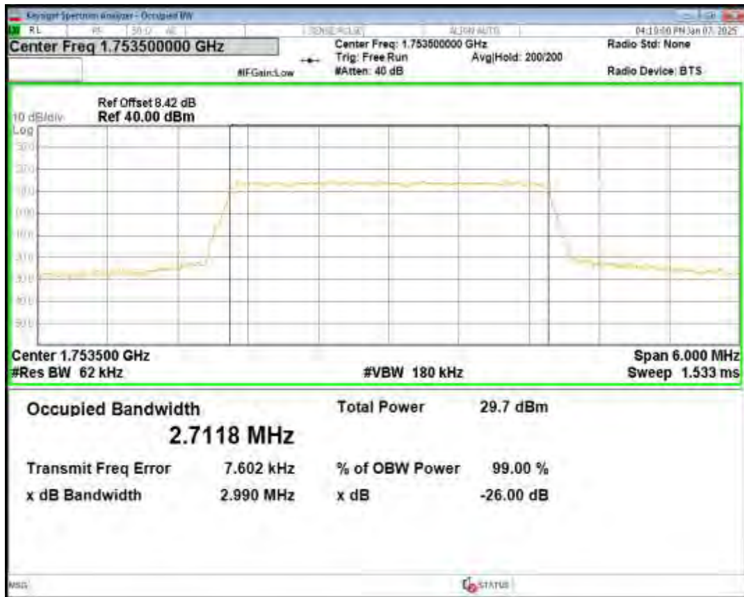
Band4 QPSK BW=5MHz Channel=19975 RB Size=25 Position=#0
