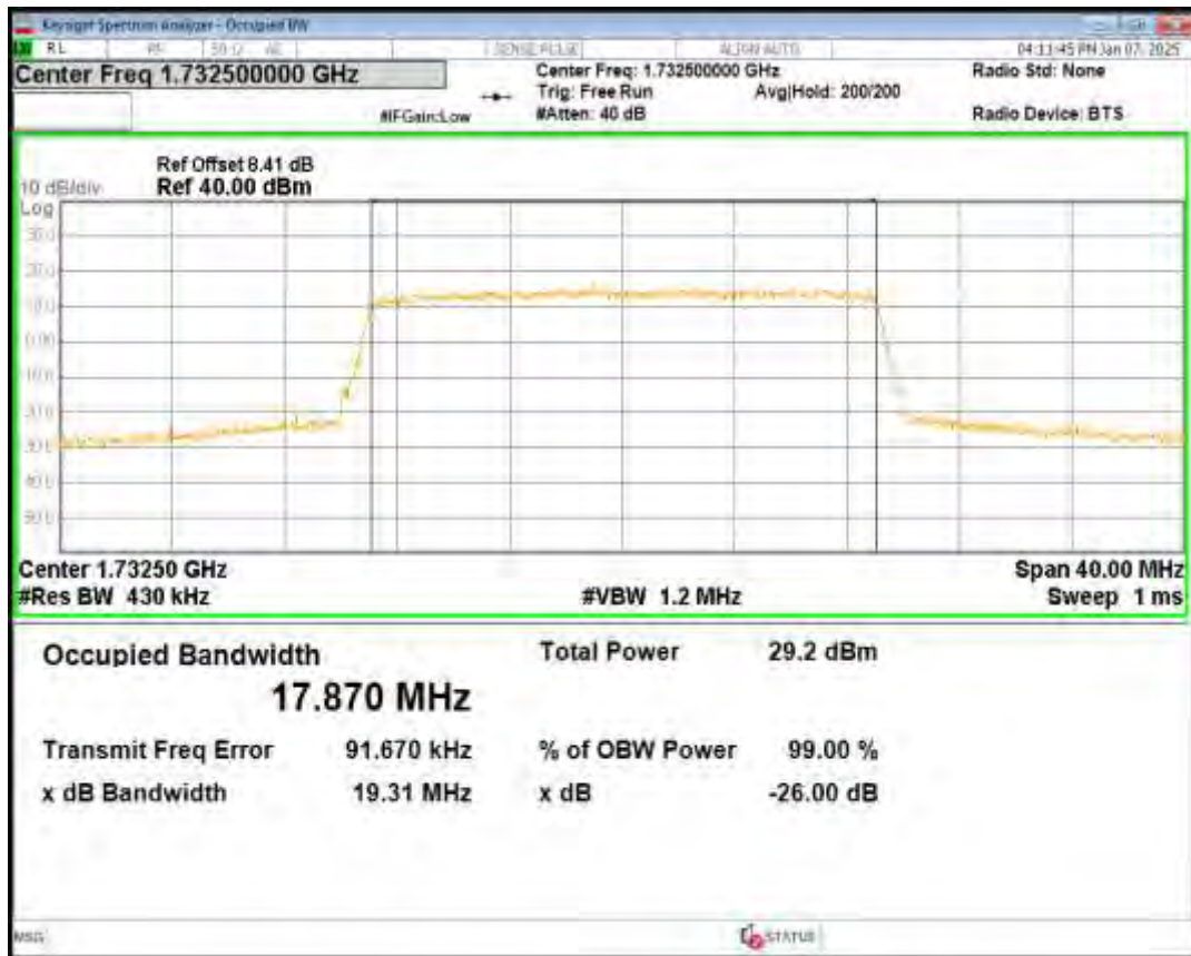
Band4 QPSK BW=20MHz Channel=20300 RB Size=100 Position=#0
