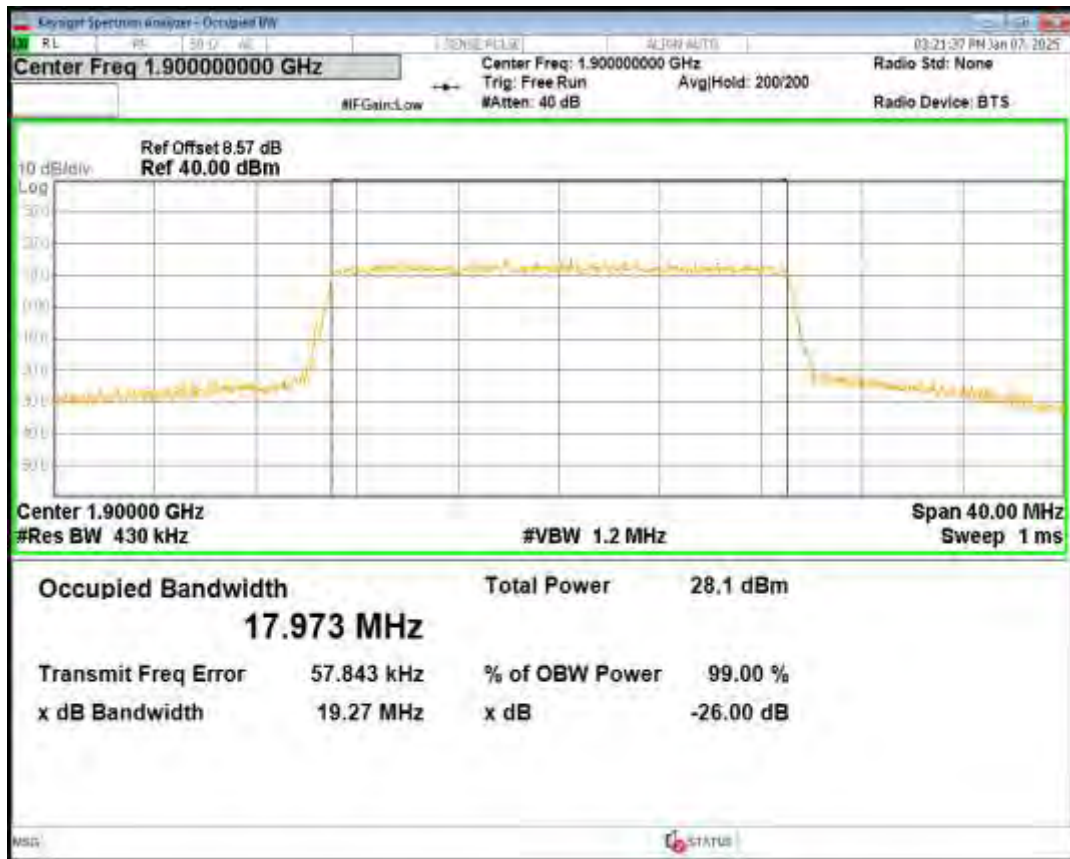
Band2 16QAM BW=3MHz Channel=18900 RB Size=15 Position=#0
