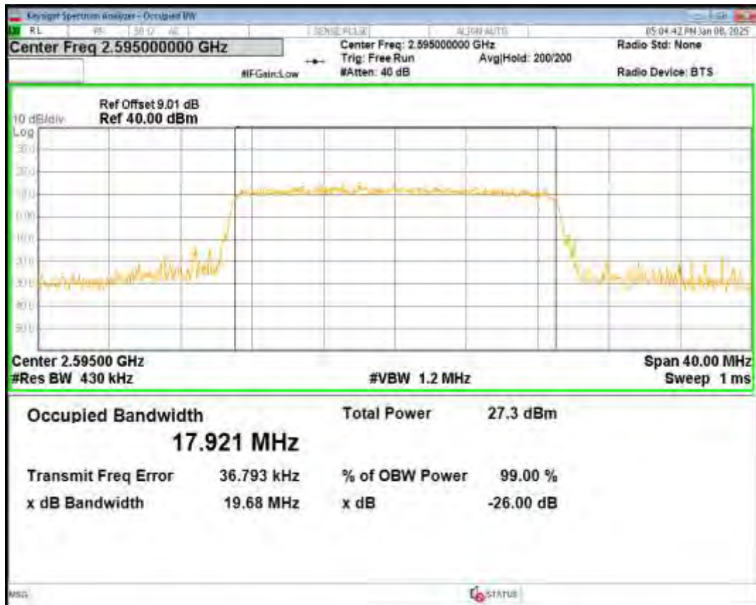
Band38 QPSK BW=10MHz Channel=38000 RB Size=50 Position=#0
