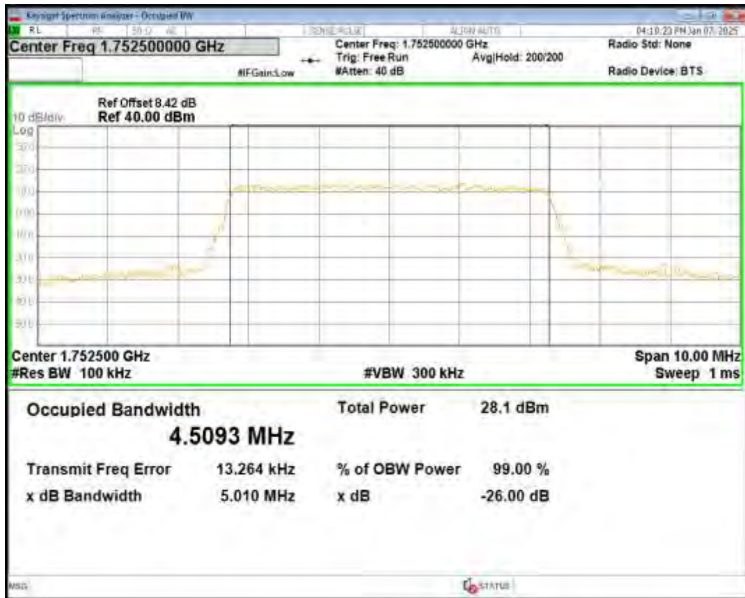
Band4 16QAM BW=5MHz Channel=20175 RB Size=25 Position=#0
