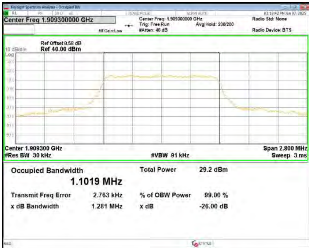
Band2 QPSK BW=1.4MHz Channel=18900 RB Size=6 Position=#0
