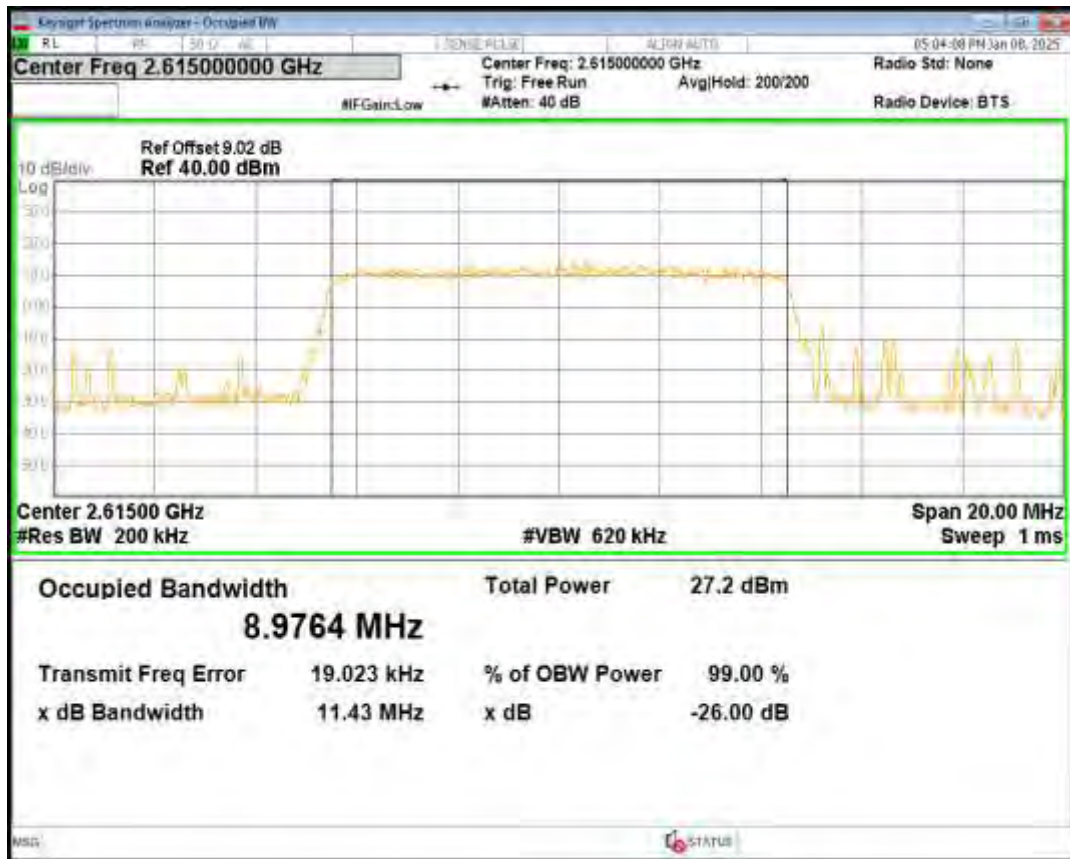
Band38 16QAM BW=15MHz Channel=37825 RB Size=75 Position=#0
