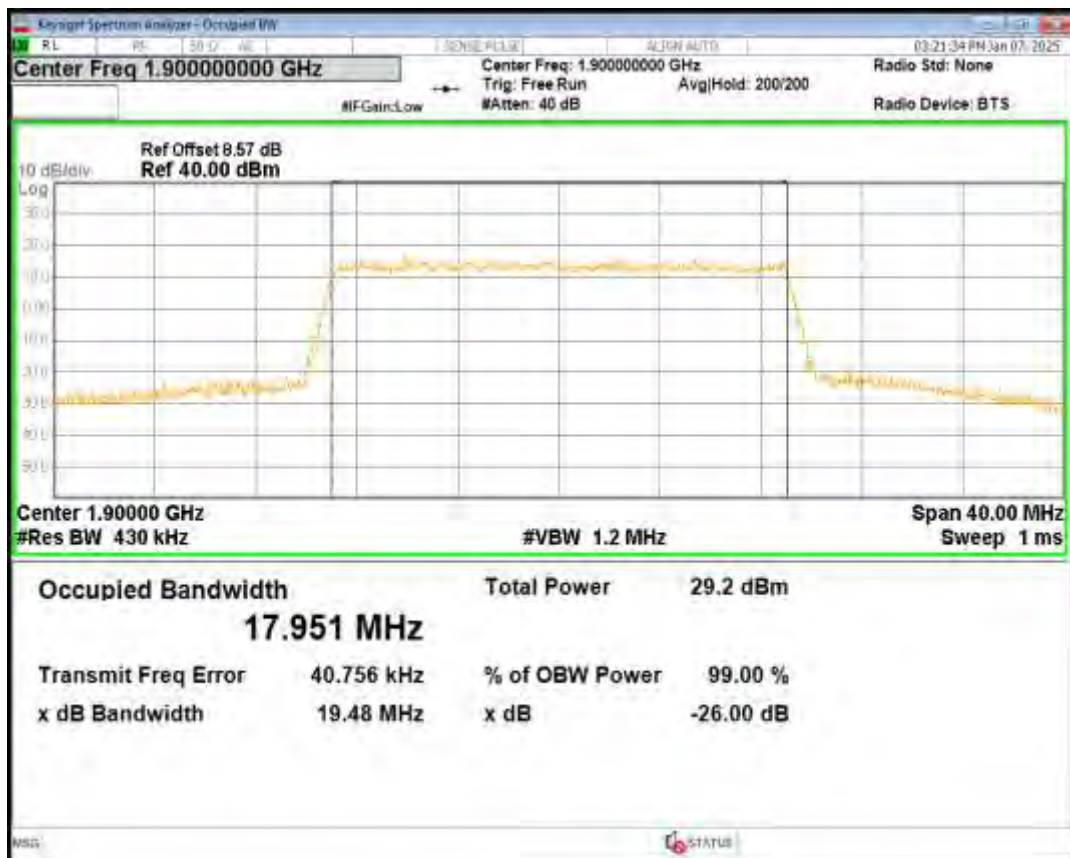
Band2 QPSK BW=3MHz Channel=18615 RB Size=15 Position=#0
