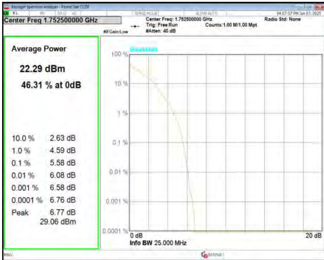
Band40(2305-2315) 16QAM BW=10MHz Channel=38750 RB Size=1 Position=#0
