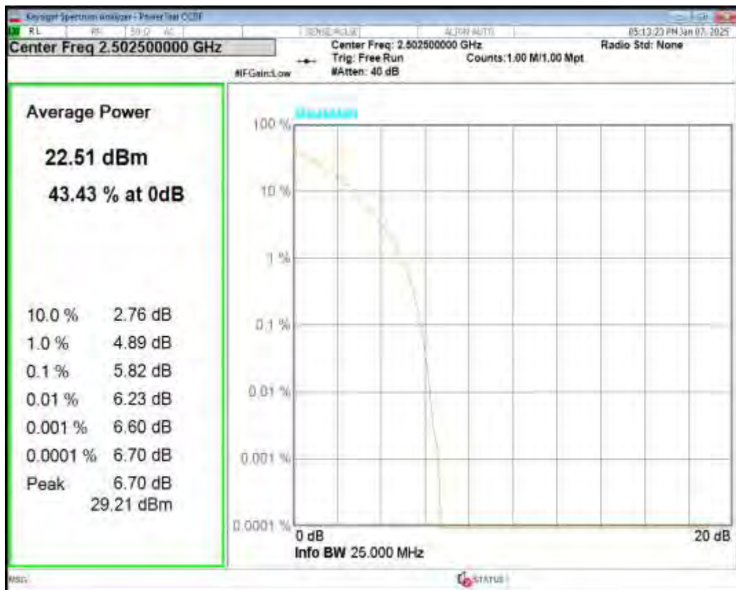
Band7 QPSK BW=5MHz Channel=21425 RB Size=1 Position=#0
