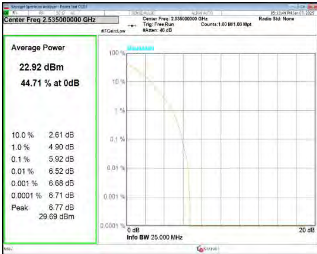
Band7 QPSK BW=10MHz Channel=21400 RB Size=1 Position=#0
