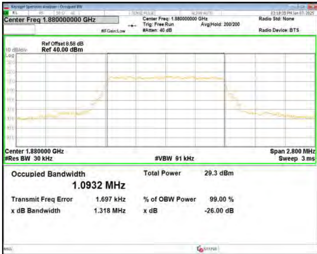
Band2 QPSK BW=10MHz Channel=18650 RB Size=50 Position=#0
