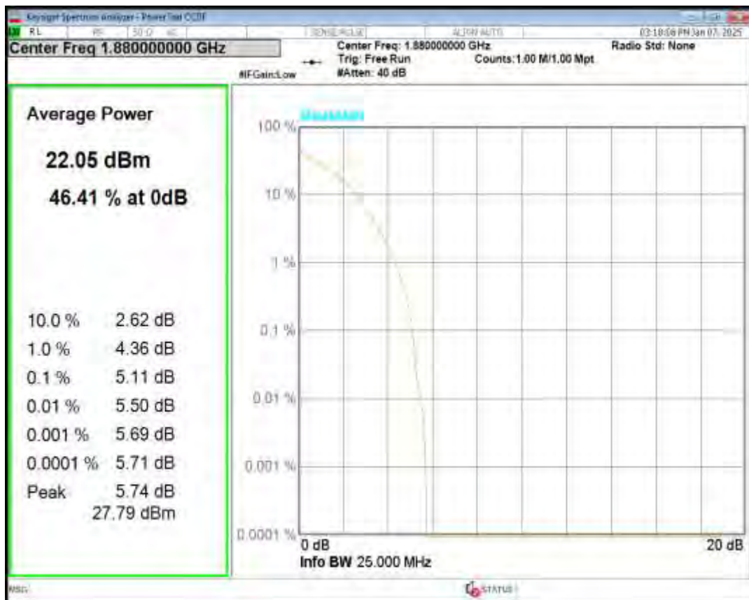
Band2 QPSK BW=20MHz Channel=19100 RB Size=1 Position=#0
