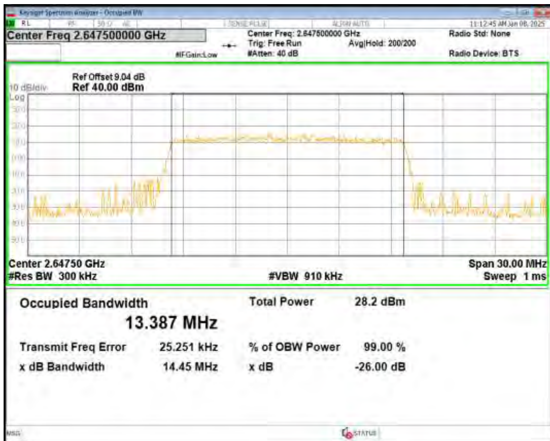
Band41(2555-2655) QPSK BW=20MHz Channel=40340 RB Size=100 Position=#0
