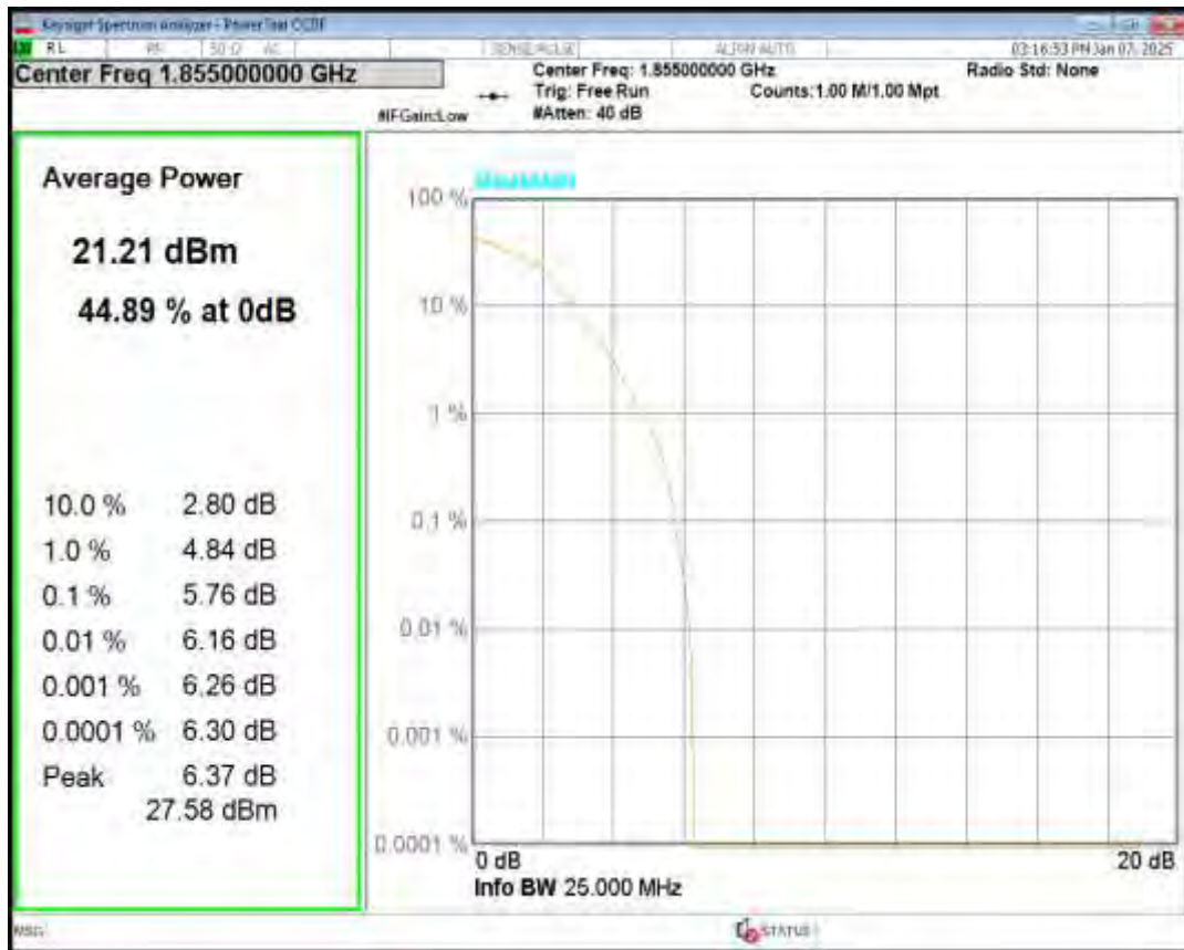
Band2 16QAM BW=10MHz Channel=18900 RB Size=1 Position=#0
