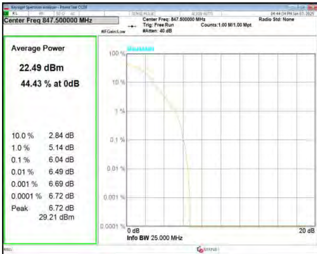
Band5 16QAM BW=5MHz Channel=20625 RB Size=1 Position=#0
