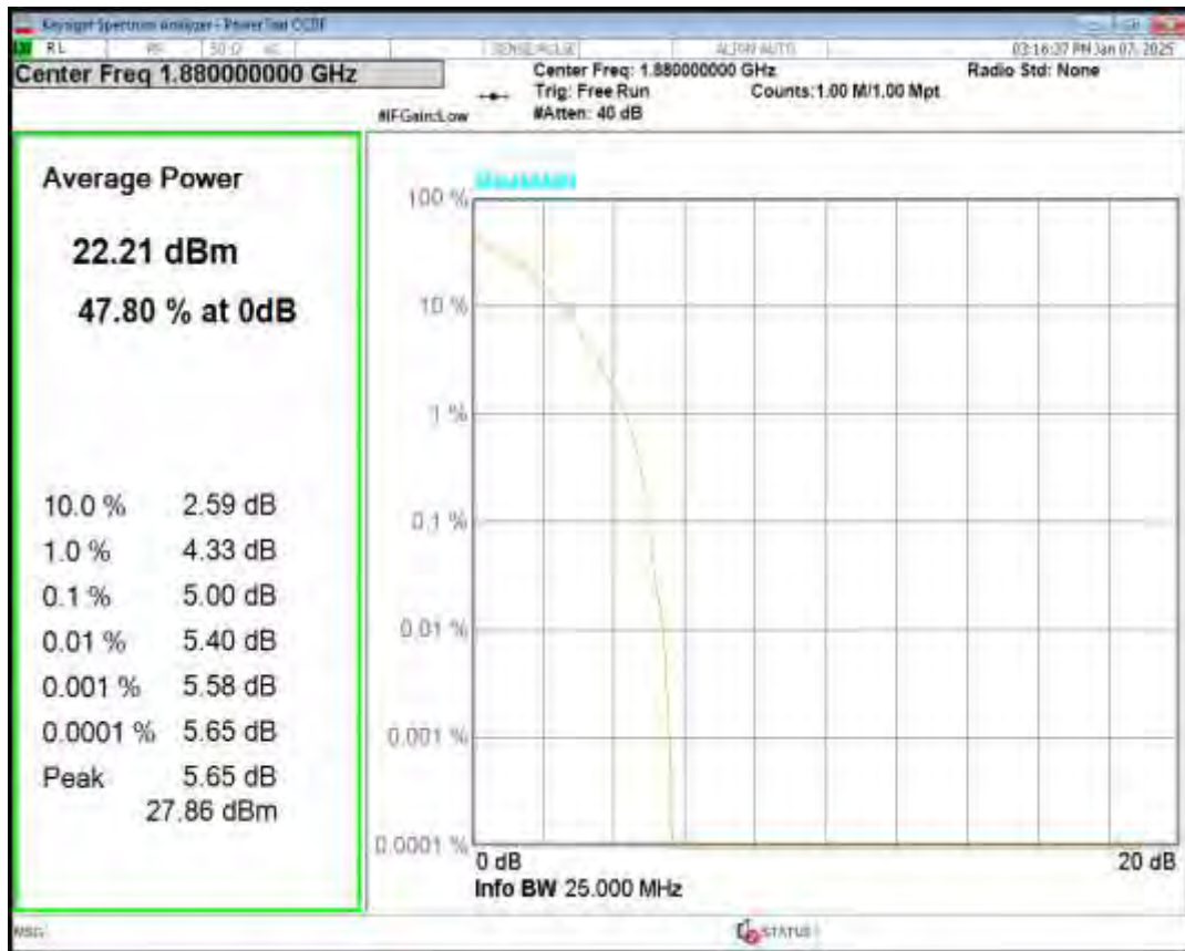
Band2 QPSK BW=5MHz Channel=18625 RB Size=1 Position=#0
