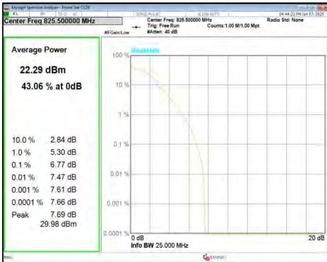
Band5 16QAM BW=10MHz Channel=20600 RB Size=1 Position=#0
