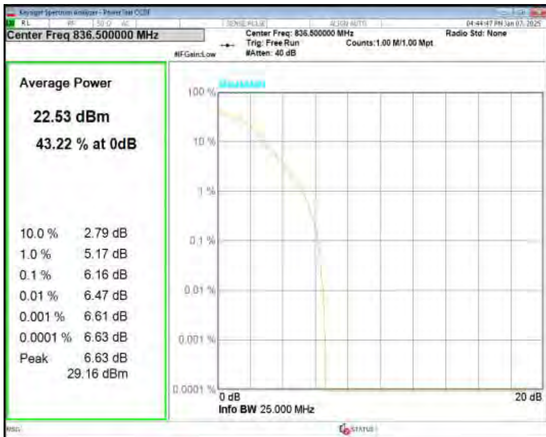
Band5 16QAM BW=5MHz Channel=20425 RB Size=1 Position=#0
