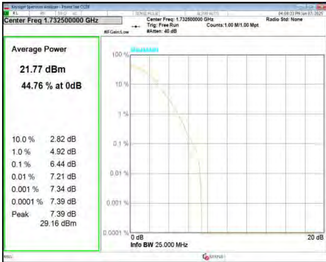
Band4 16QAM BW=15MHz Channel=20325 RB Size=1 Position=#0
