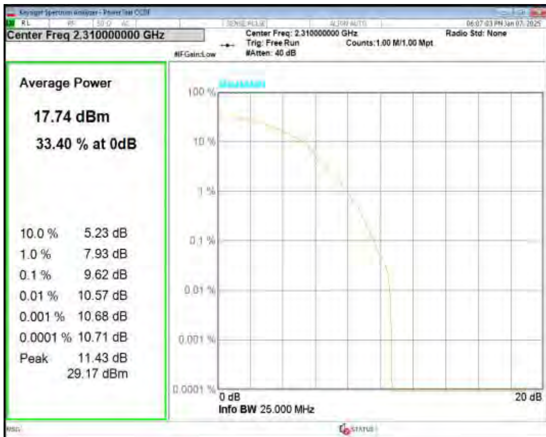
Band40(2305-2315) 16QAM BW=5MHz Channel=38725 RB Size=1 Position=#0
