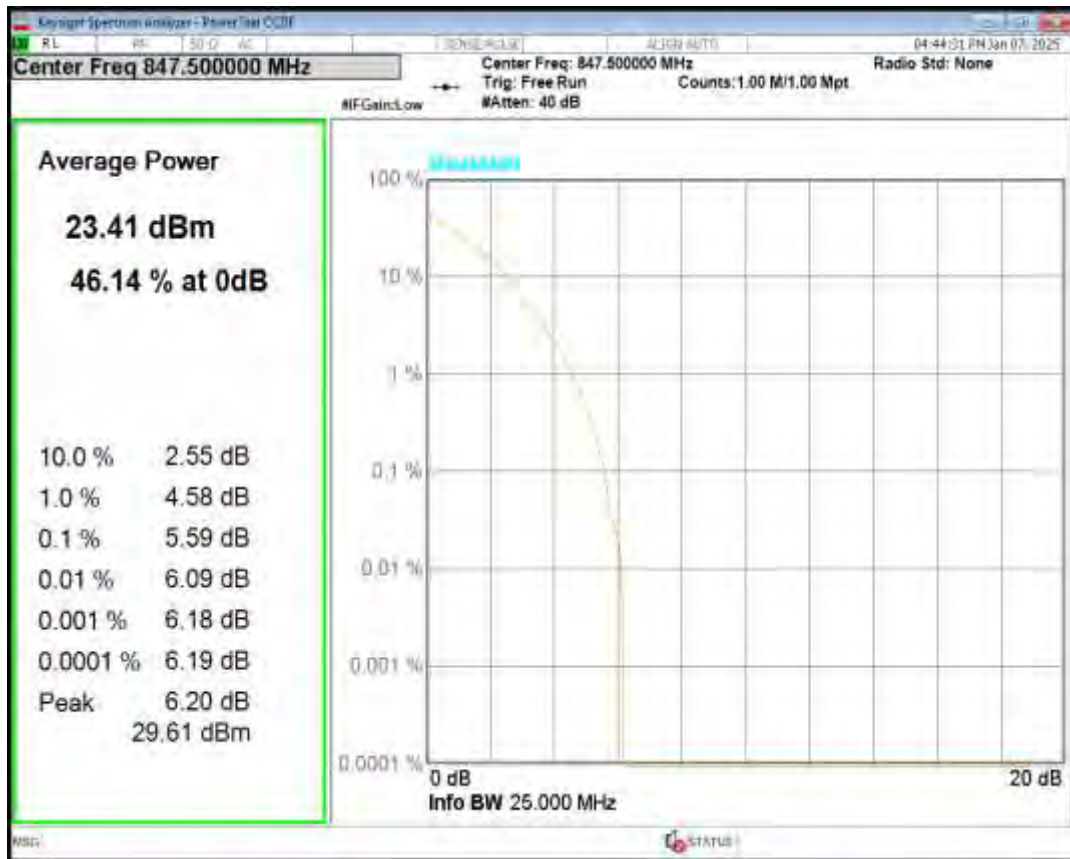
Band5 QPSK BW=5MHz Channel=20425 RB Size=1 Position=#0
