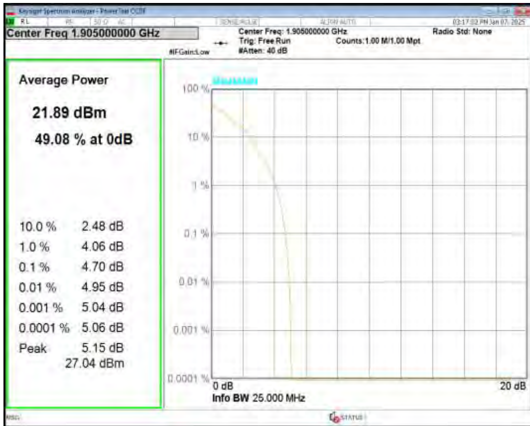
Band2 QPSK BW=15MHz Channel=18675 RB Size=1 Position=#0
