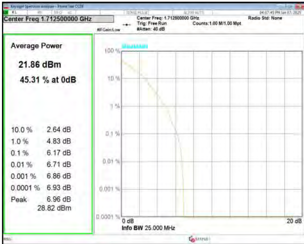
Band4 QPSK BW=5MHz Channel=20175 RB Size=1 Position=#0
