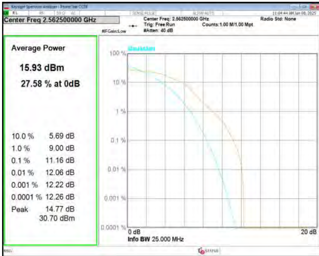
Band41(2555-2655) 16QAM BW=5MHz Channel=40740 RB Size=1 Position=#0
