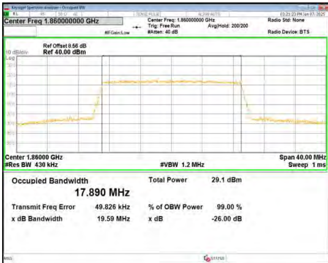
Band2 QPSK BW=20MHz Channel=18900 RB Size=100 Position=#0
