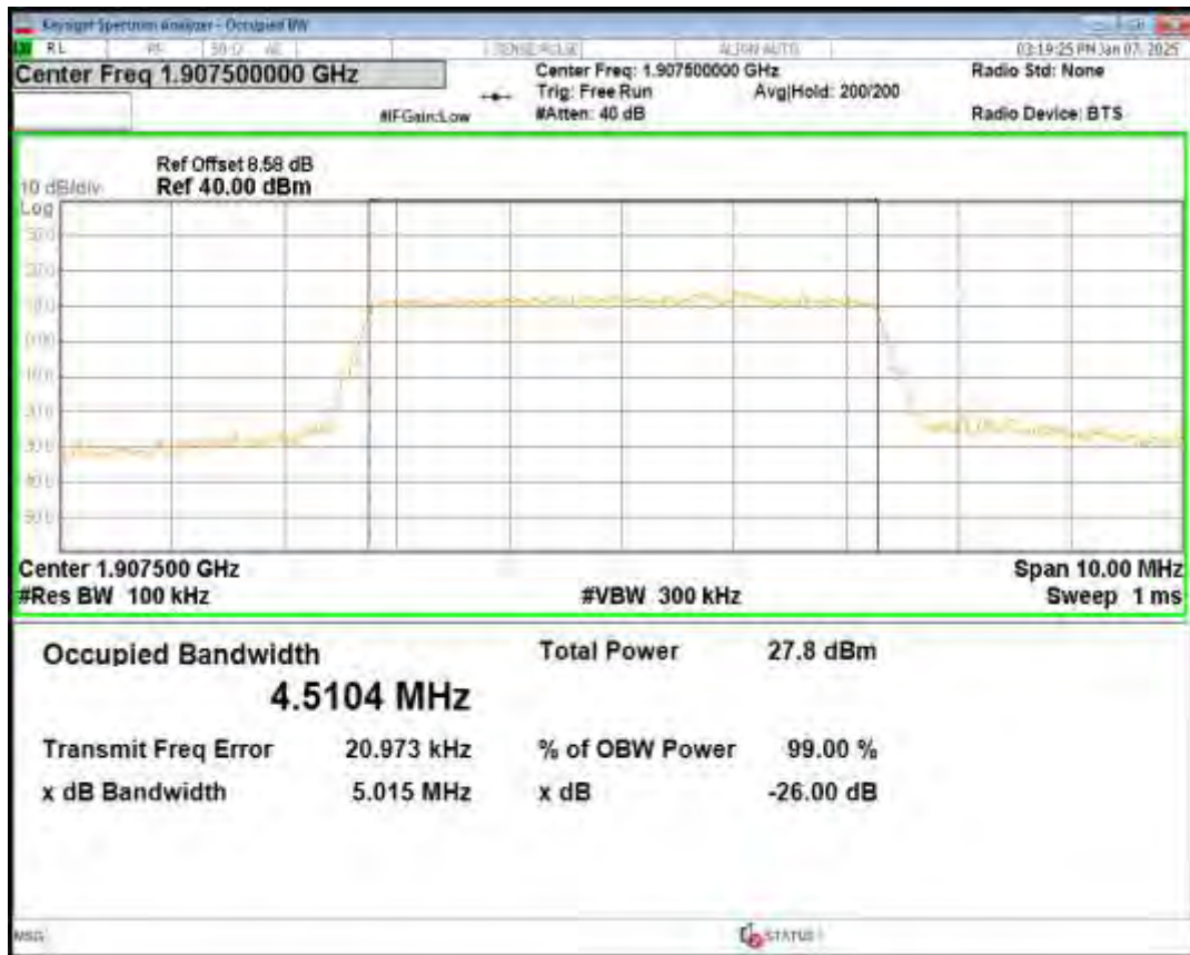
Band2 16QAM BW=3MHz Channel=18615 RB Size=15 Position=#0
