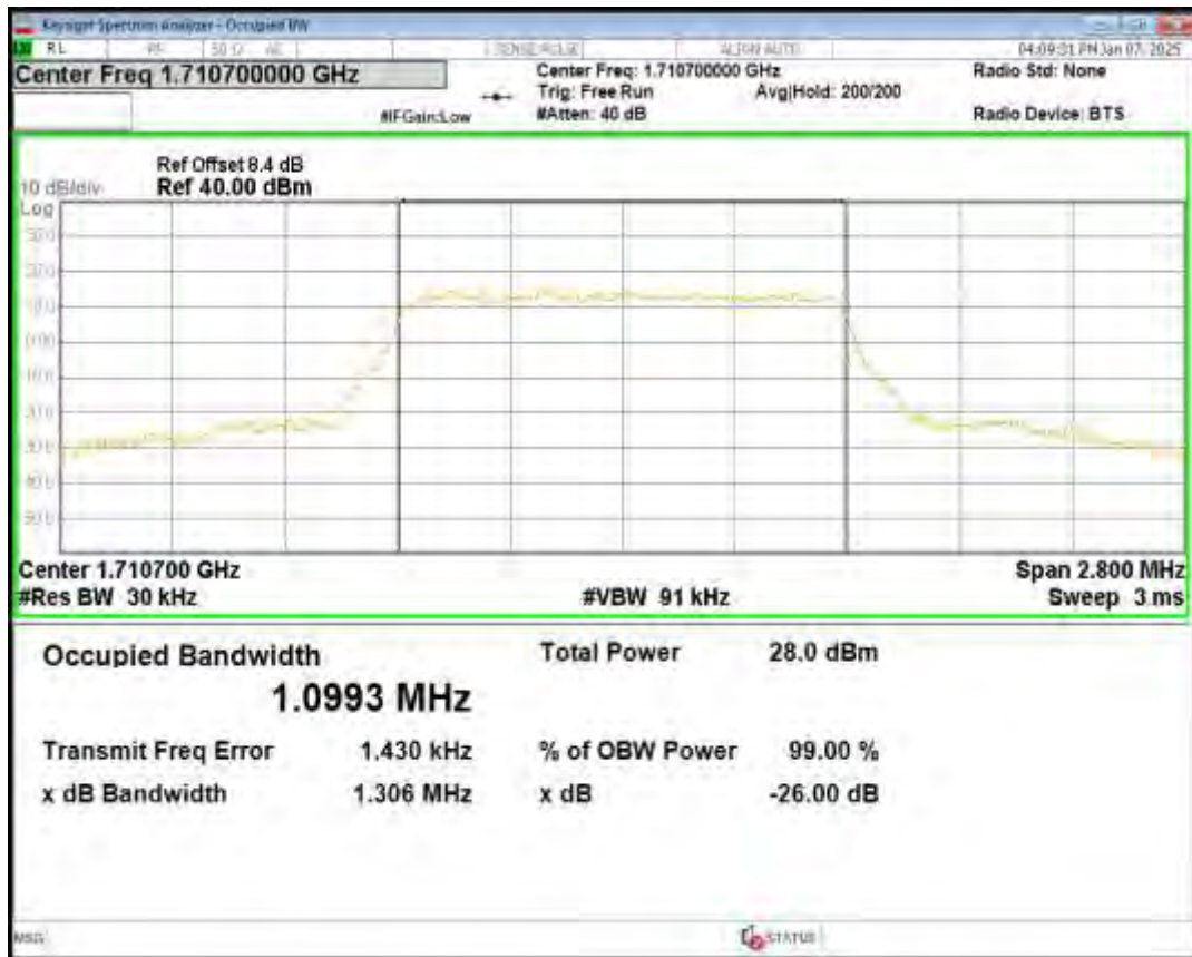
Band4 16QAM BW=1.4MHz Channel=20175 RB Size=6 Position=#0
