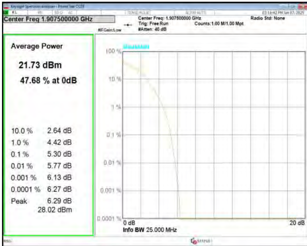
Band38 16QAM BW=10MHz Channel=37800 RB Size=1 Position=#0
