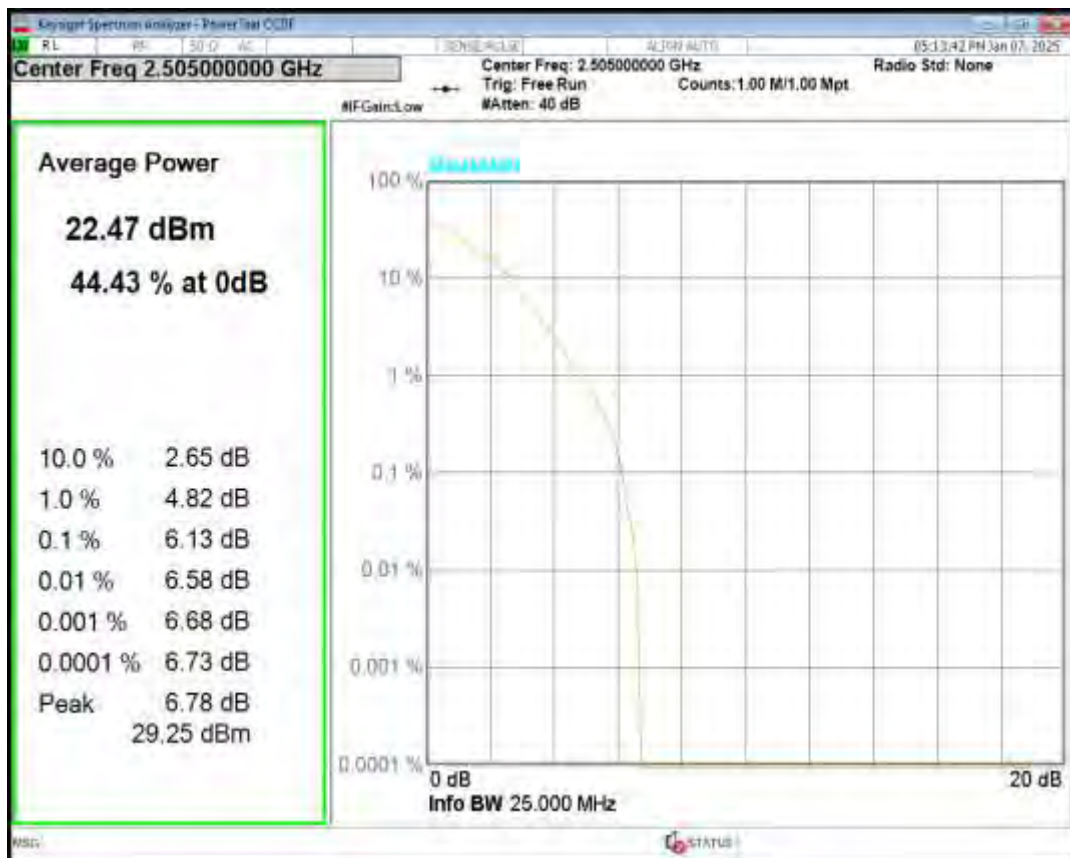
Band7 QPSK BW=10MHz Channel=21100 RB Size=1 Position=#0
