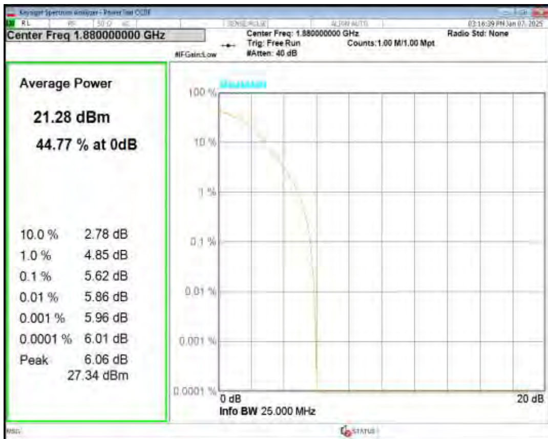
Band2 16QAM BW=5MHz Channel=18625 RB Size=1 Position=#0
