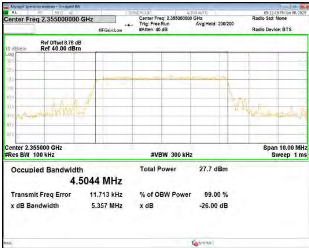
Band40(2350-2360) 16QAM BW=5MHz Channel=39225 RB Size=25 Position=#0
