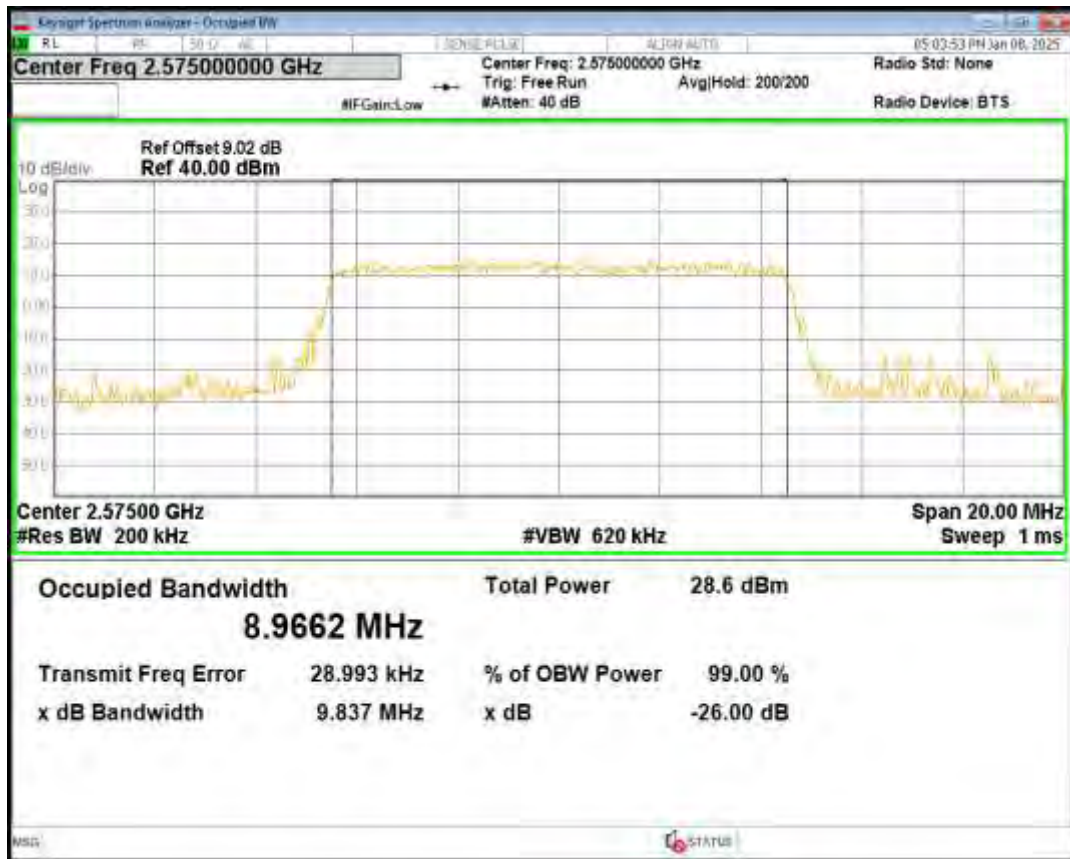
Band38 16QAM BW=5MHz Channel=38000 RB Size=25 Position=#0
