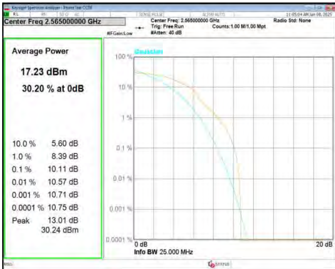
Band41(2555-2655) 16QAM BW=15MHz Channel=41165 RB Size=1 Position=#0
