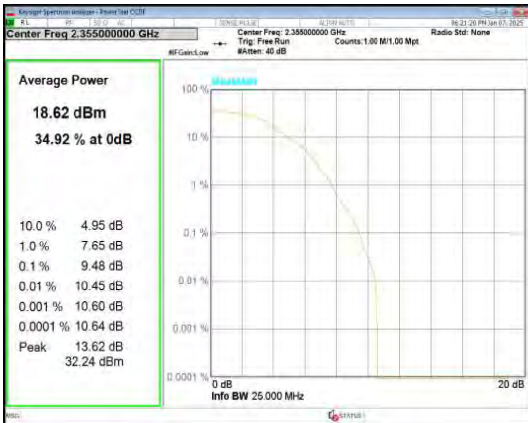
Band40(2350-2360) QPSK BW=5MHz Channel=39175 RB Size=1 Position=#0
