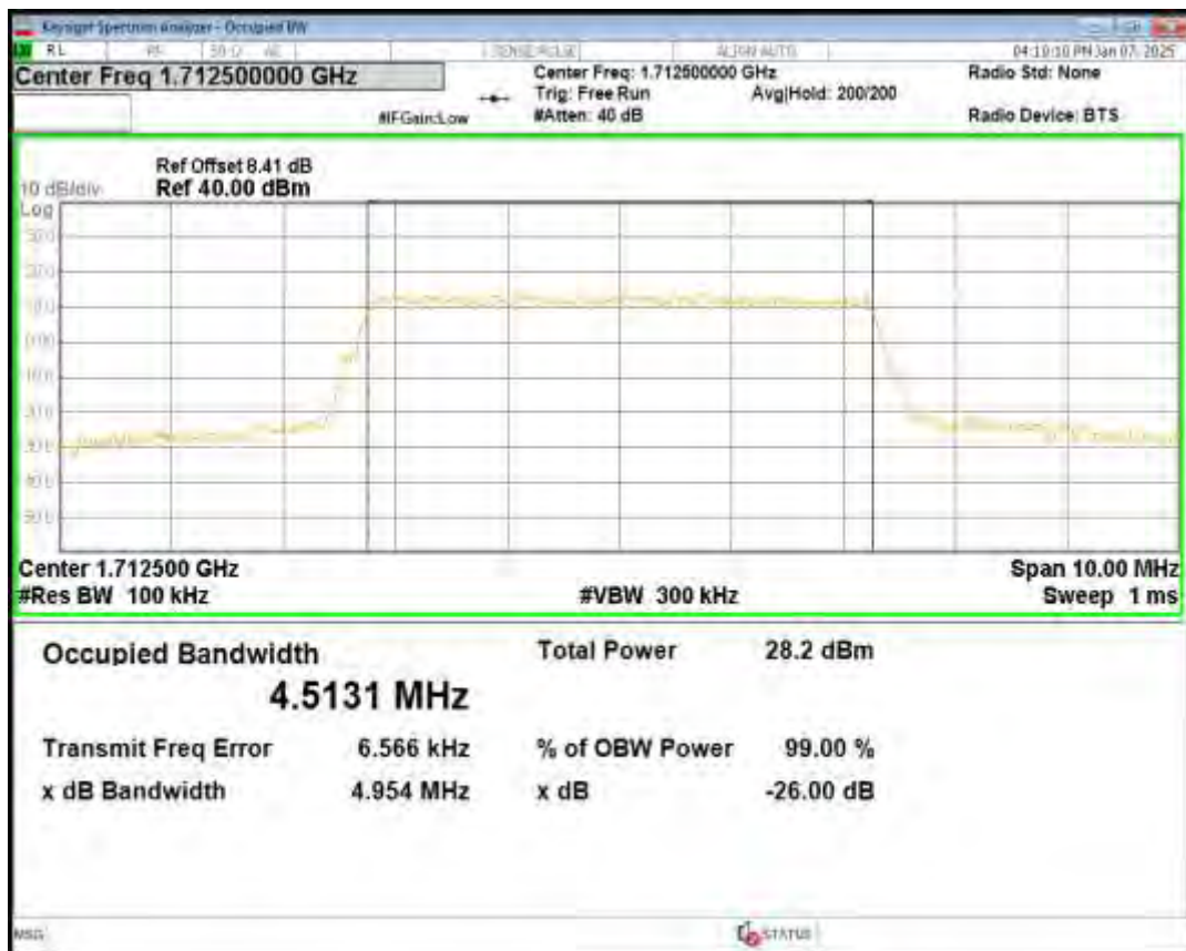
Band4 16QAM BW=5MHz Channel=20375 RB Size=25 Position=#0
