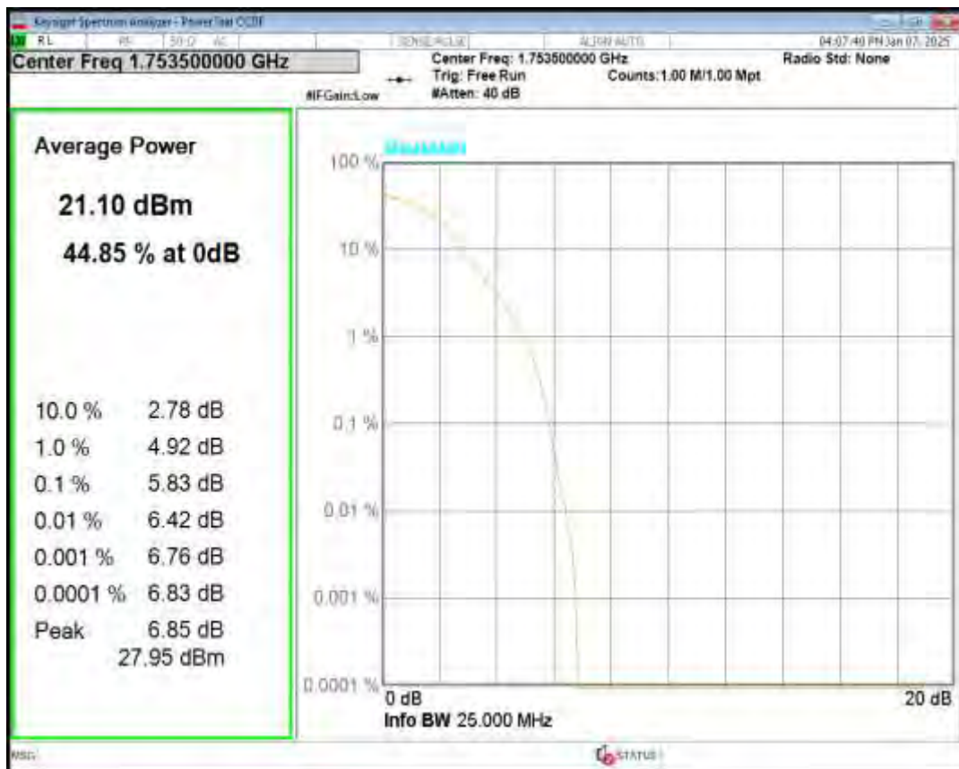
Band4 16QAM BW=5MHz Channel=19975 RB Size=1 Position=#0
