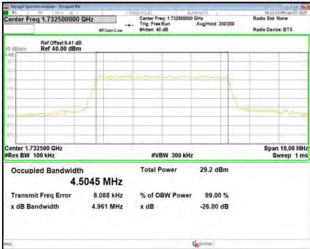
Band4 QPSK BW=5MHz Channel=20375 RB Size=25 Position=#0
