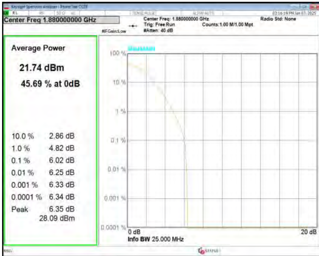
Band2 16QAM BW=3MHz Channel=18615 RB Size=1 Position=#0
