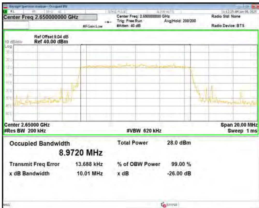
Band41(2555-2655) QPSK BW=15MHz Channel=40315 RB Size=75 Position=#0
