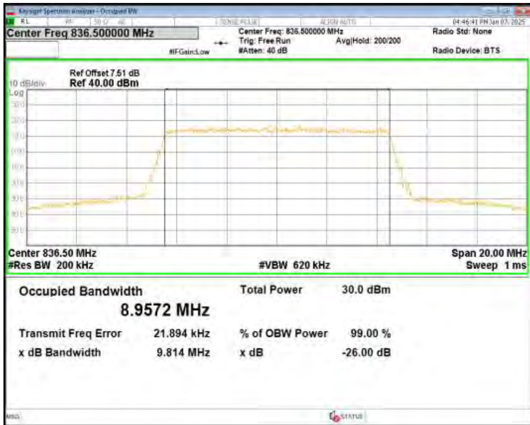
Band5 QPSK BW=10MHz Channel=20450 RB Size=50 Position=#0
