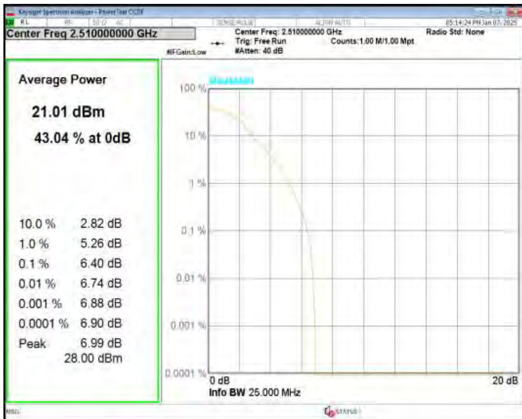
Band7 16QAM BW=15MHz Channel=21375 RB Size=1 Position=#0
