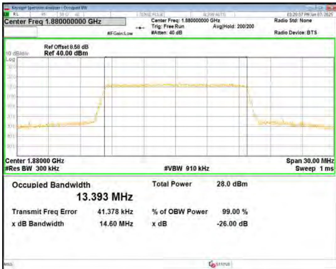
Band2 16QAM BW=15MHz Channel=19125 RB Size=75 Position=#0
