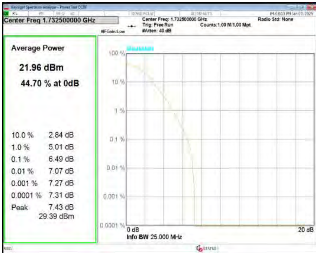
Band4 16QAM BW=10MHz Channel=20350 RB Size=1 Position=#0
