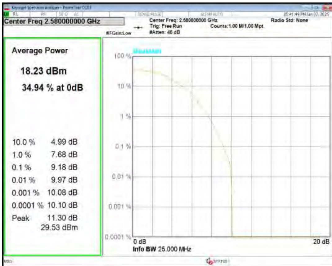
Band38 QPSK BW=20MHz Channel=38000 RB Size=1 Position=#0
