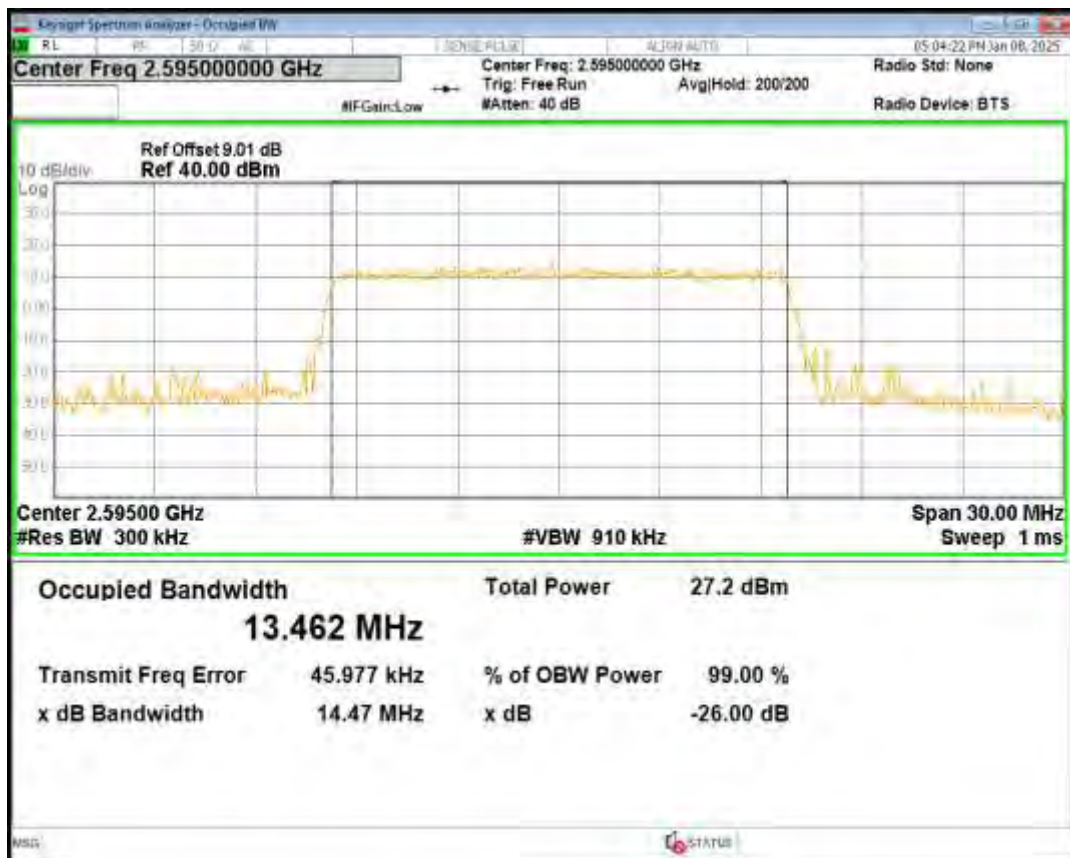
Band38 16QAM BW=20MHz Channel=38000 RB Size=100 Position=#0
