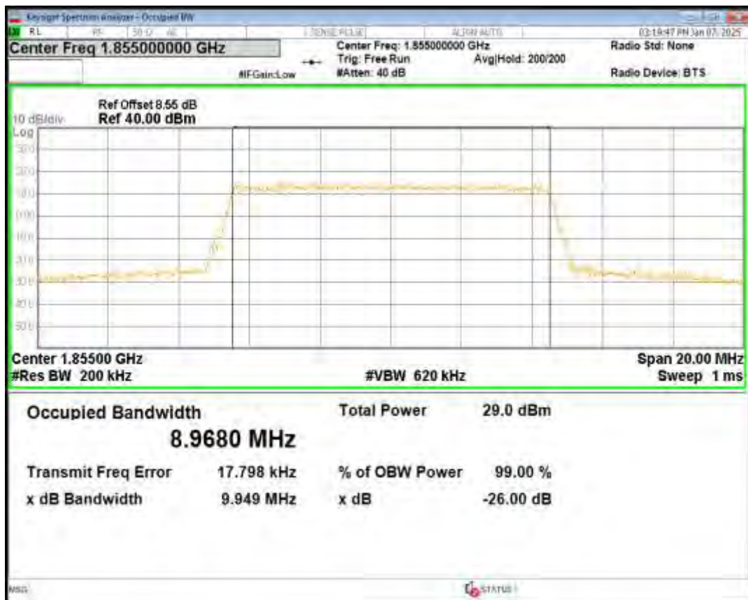
Band2 QPSK BW=15MHz Channel=19125 RB Size=75 Position=#0
