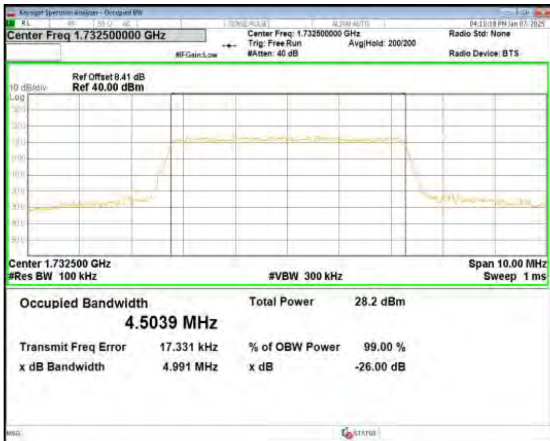
Band4 QPSK BW=1.4MHz Channel=19957 RB Size=6 Position=#0
