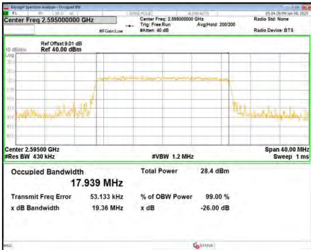
Band38 QPSK BW=20MHz Channel=38150 RB Size=100 Position=#0
