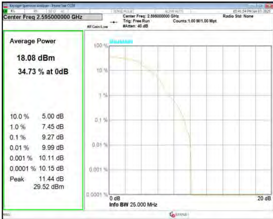
Band38 QPSK BW=20MHz Channel=38150 RB Size=1 Position=#0
