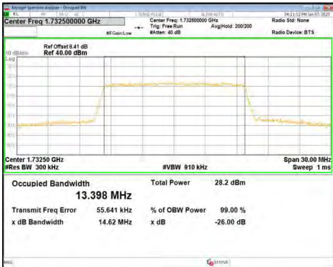
Band4 16QAM BW=15MHz Channel=20325 RB Size=75 Position=#0
