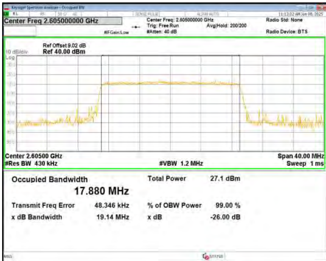
Band41(2555-2655) 16QAM BW=20MHz Channel=41140 RB Size=100 Position=#0
