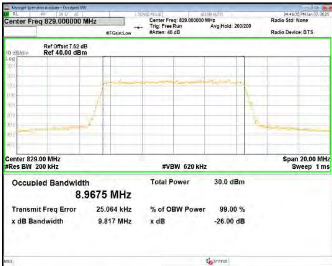
Band5 16QAM BW=5MHz Channel=20625 RB Size=25 Position=#0
