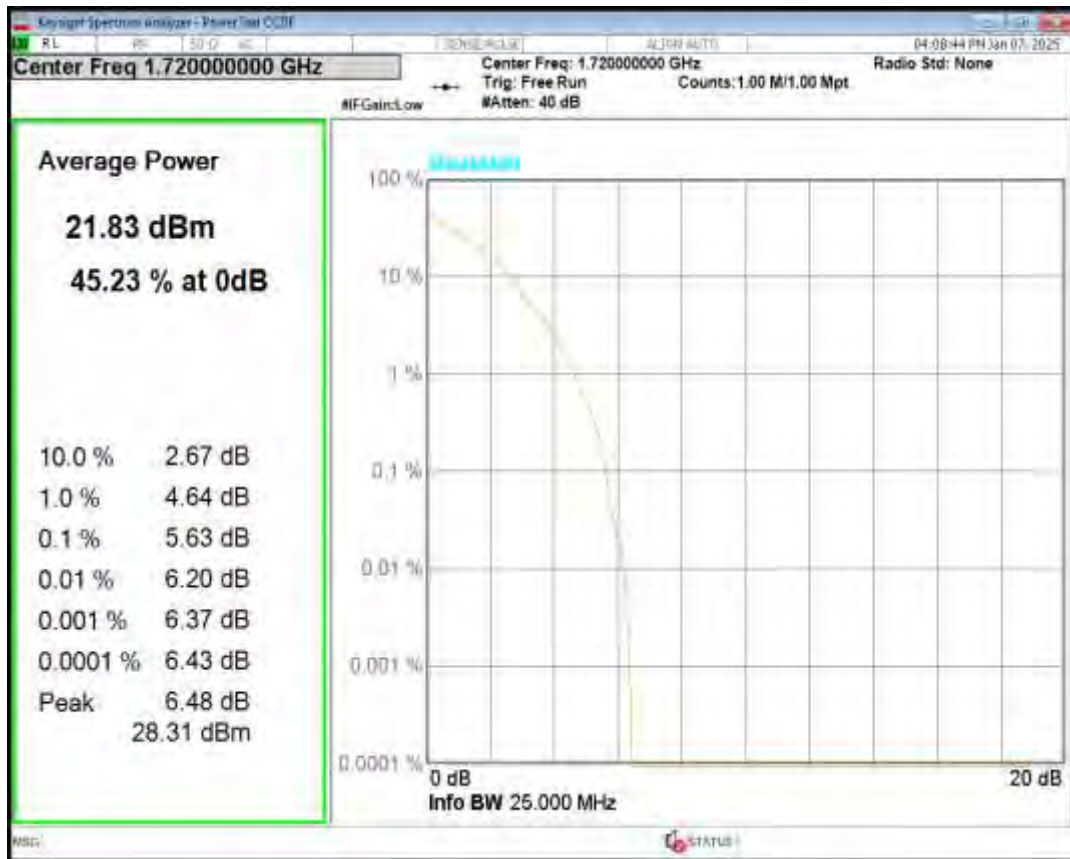
Band4 QPSK BW=3MHz Channel=20385 RB Size=1 Position=#0
