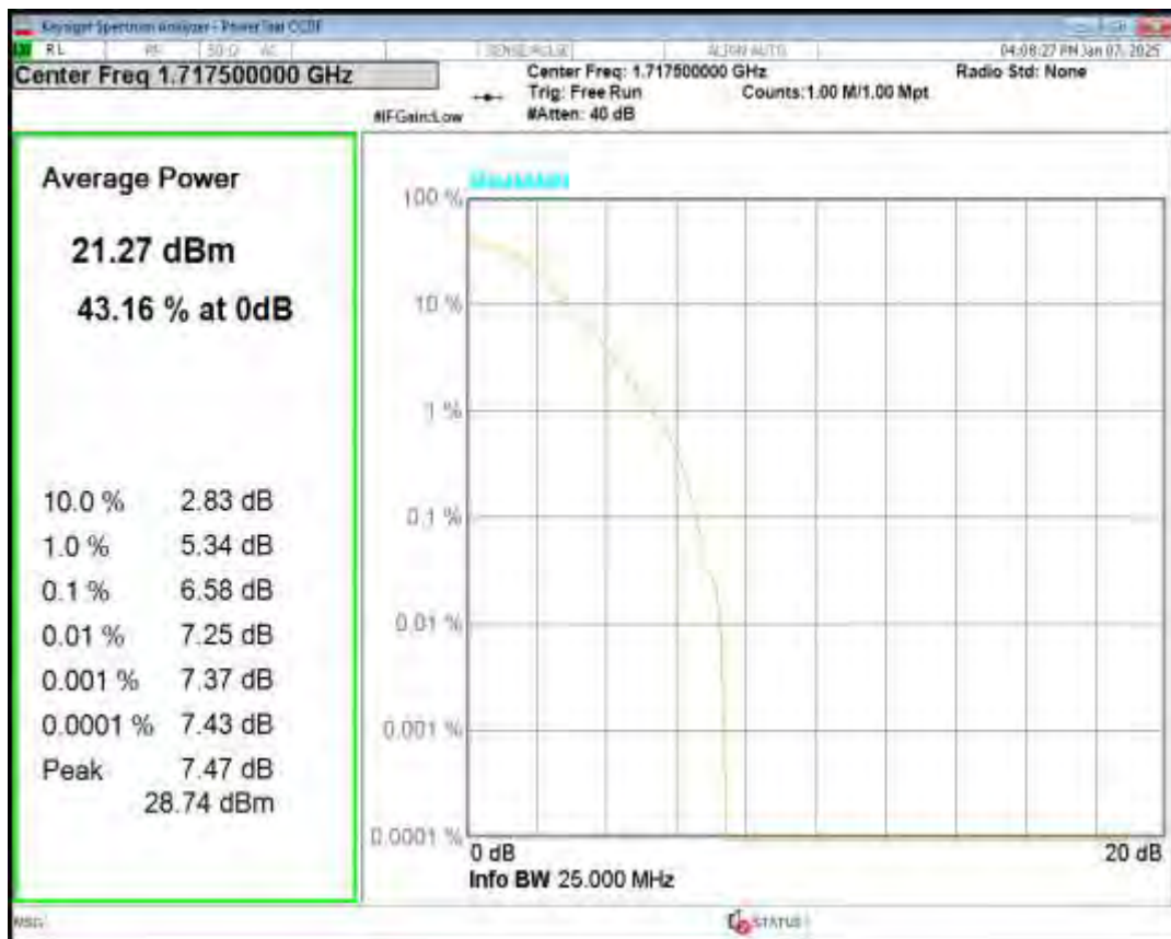
Band4 16QAM BW=15MHz Channel=20175 RB Size=1 Position=#0
