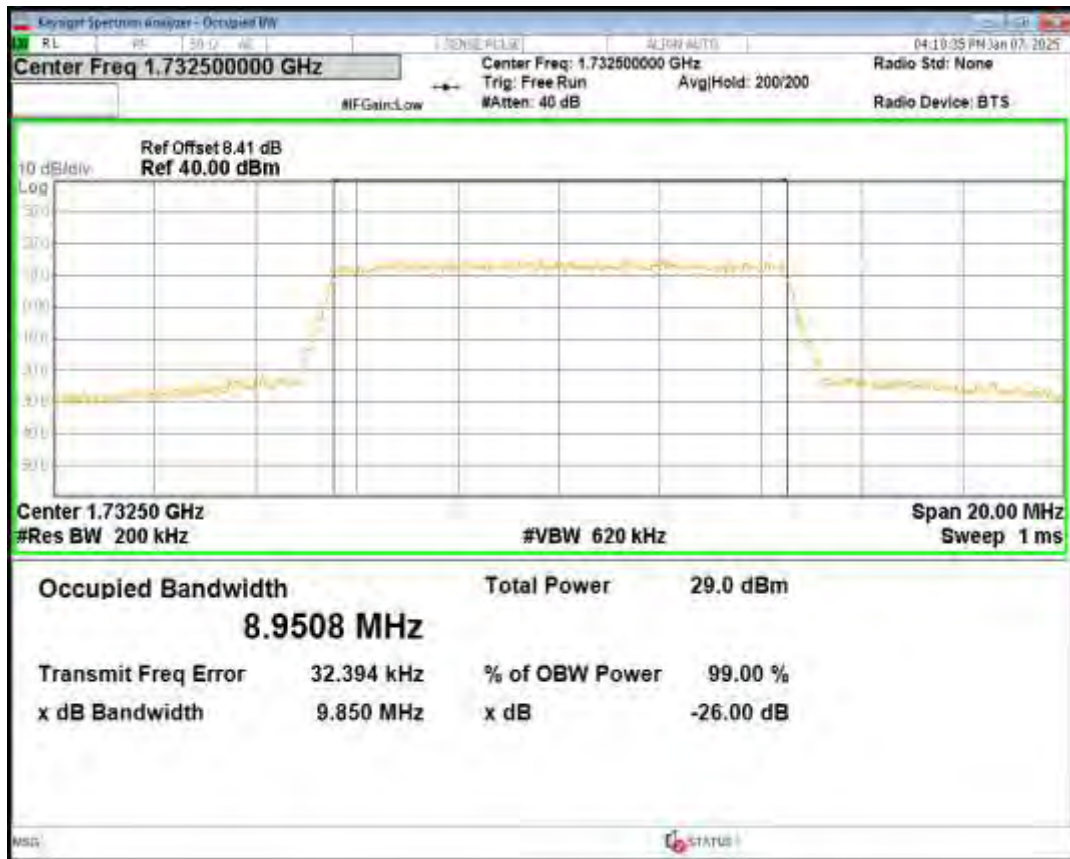
Band4 QPSK BW=10MHz Channel=20350 RB Size=50 Position=#0
