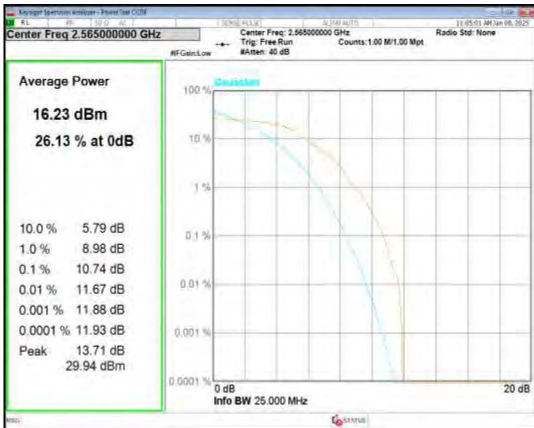
Band41(2555-2655) QPSK BW=20MHz Channel=40740 RB Size=1 Position=#0
