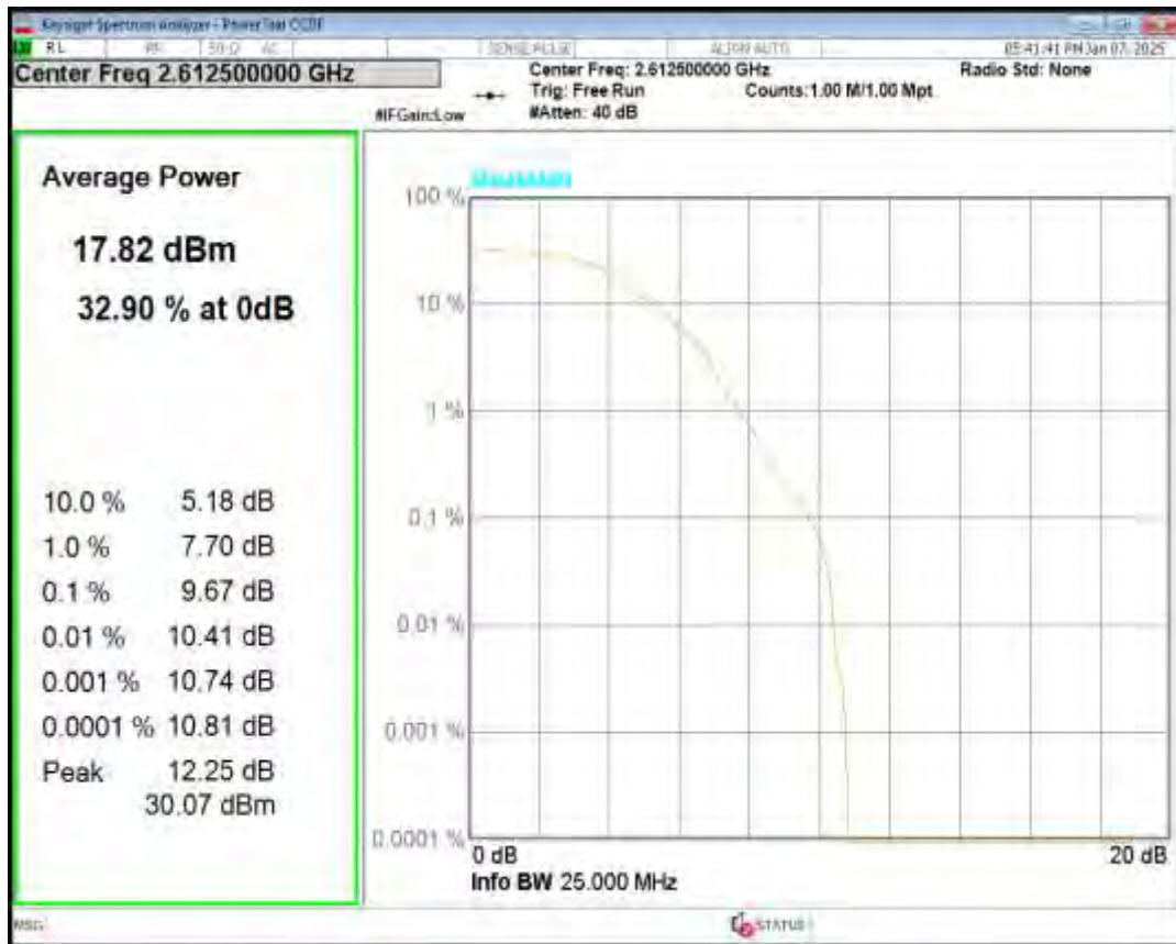
Band38 QPSK BW=20MHz Channel=37850 RB Size=1 Position=#0
