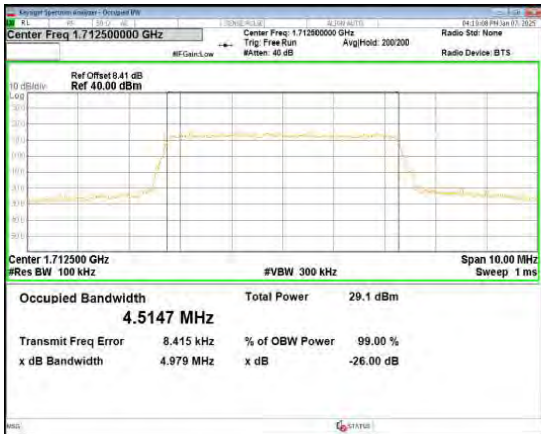
Band4 QPSK BW=5MHz Channel=20175 RB Size=25 Position=#0
