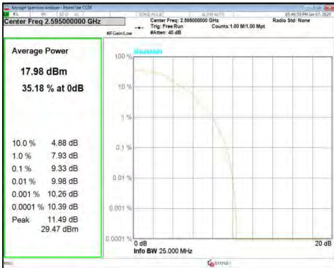
Band38 QPSK BW=5MHz Channel=38225 RB Size=1 Position=#0
