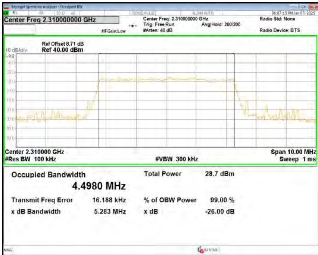
Band40(2305-2315) QPSK BW=5MHz Channel=38775 RB Size=25 Position=#0
