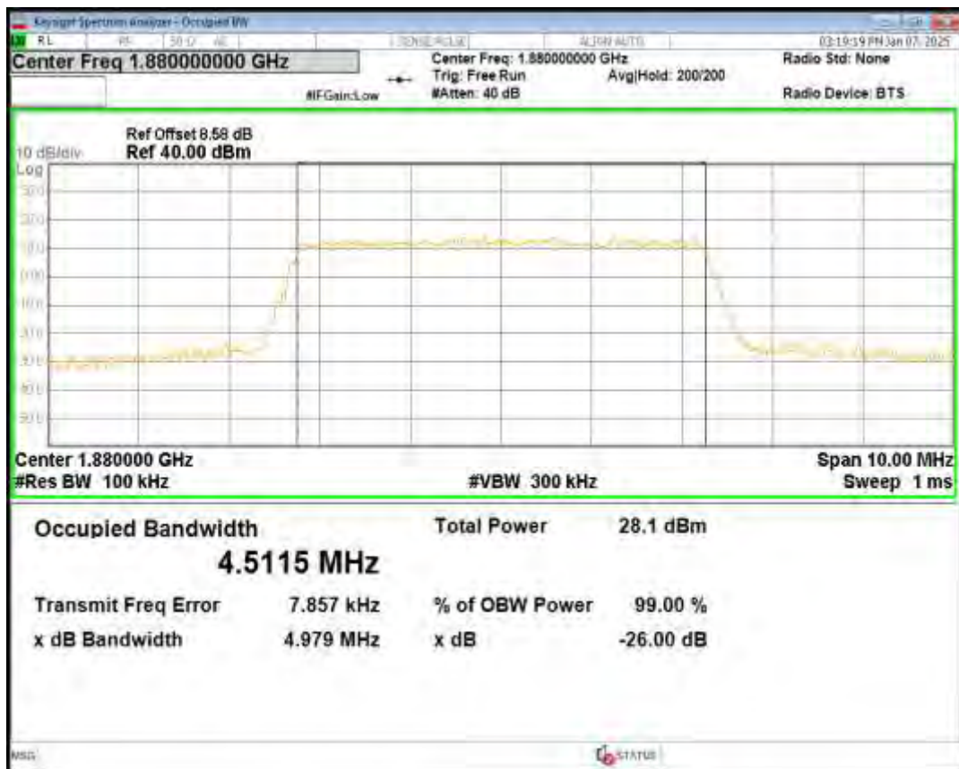
Band2 16QAM BW=5MHz Channel=18625 RB Size=25 Position=#0
