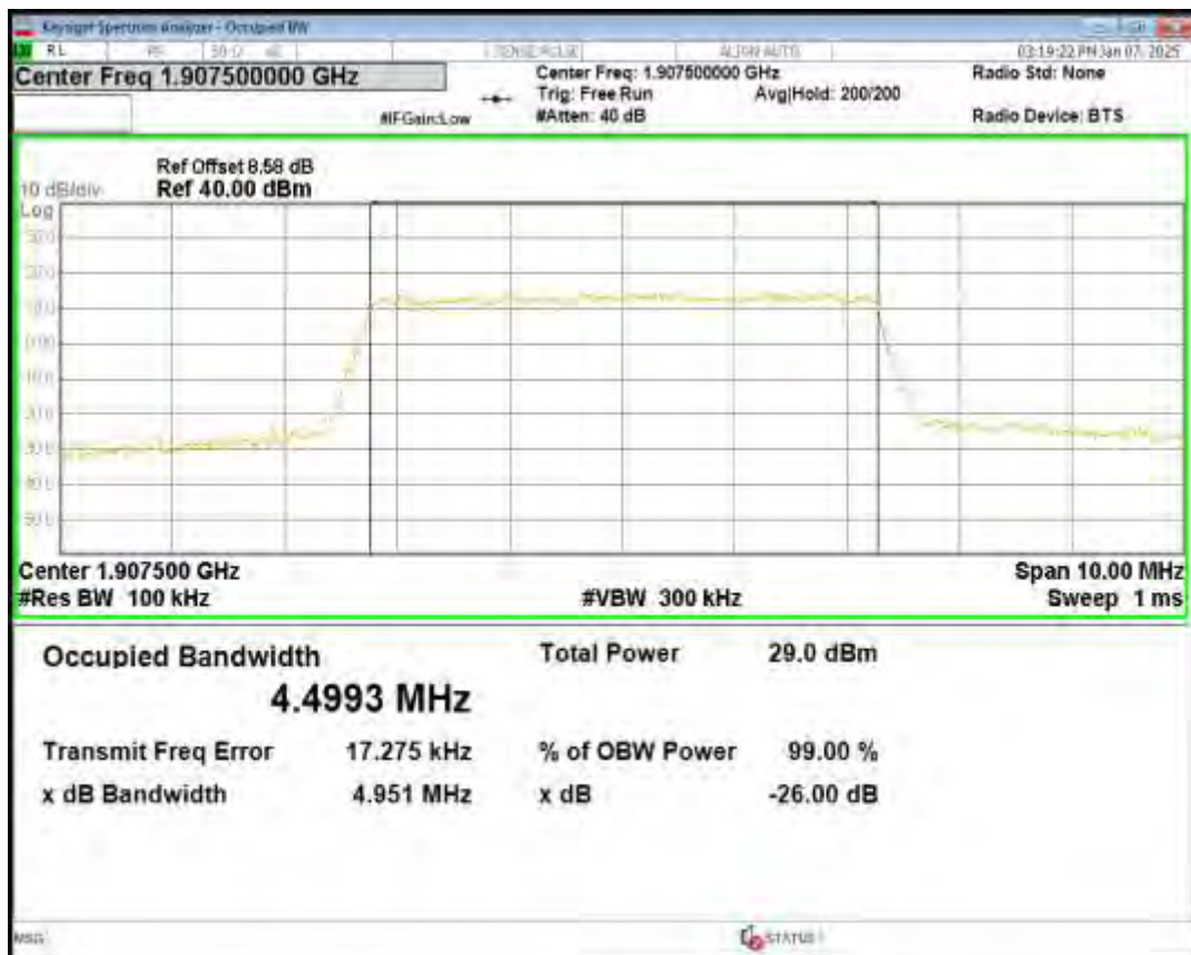
Band38 16QAM BW=10MHz Channel=37800 RB Size=50 Position=#0
