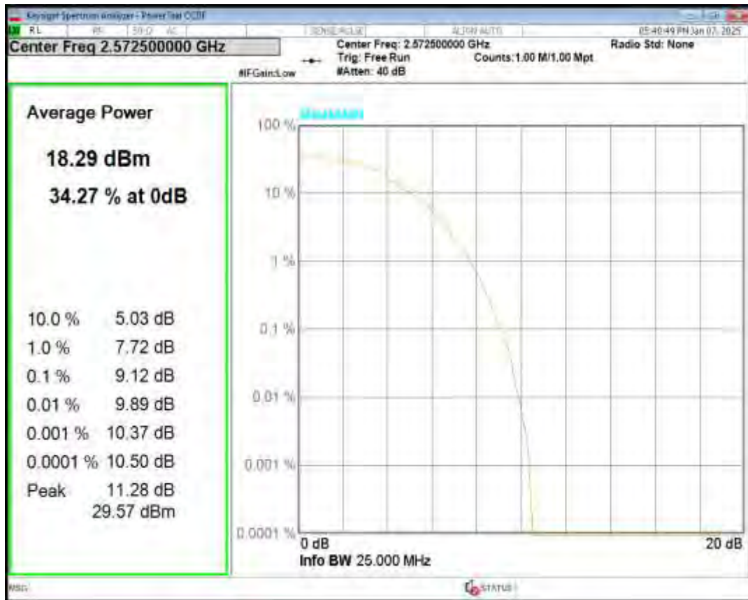
Band38 QPSK BW=5MHz Channel=38000 RB Size=1 Position=#0
