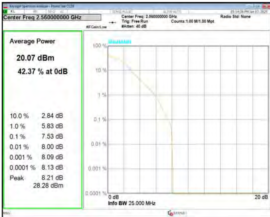
Band7 16QAM BW=5MHz Channel=21425 RB Size=1 Position=#0
