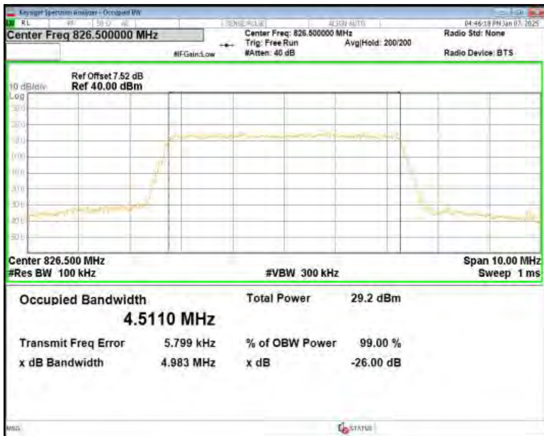
Band5 QPSK BW=3MHz Channel=20415 RB Size=15 Position=#0
