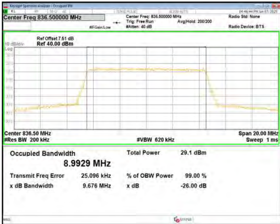
Band5 16QAM BW=10MHz Channel=20600 RB Size=50 Position=#0
