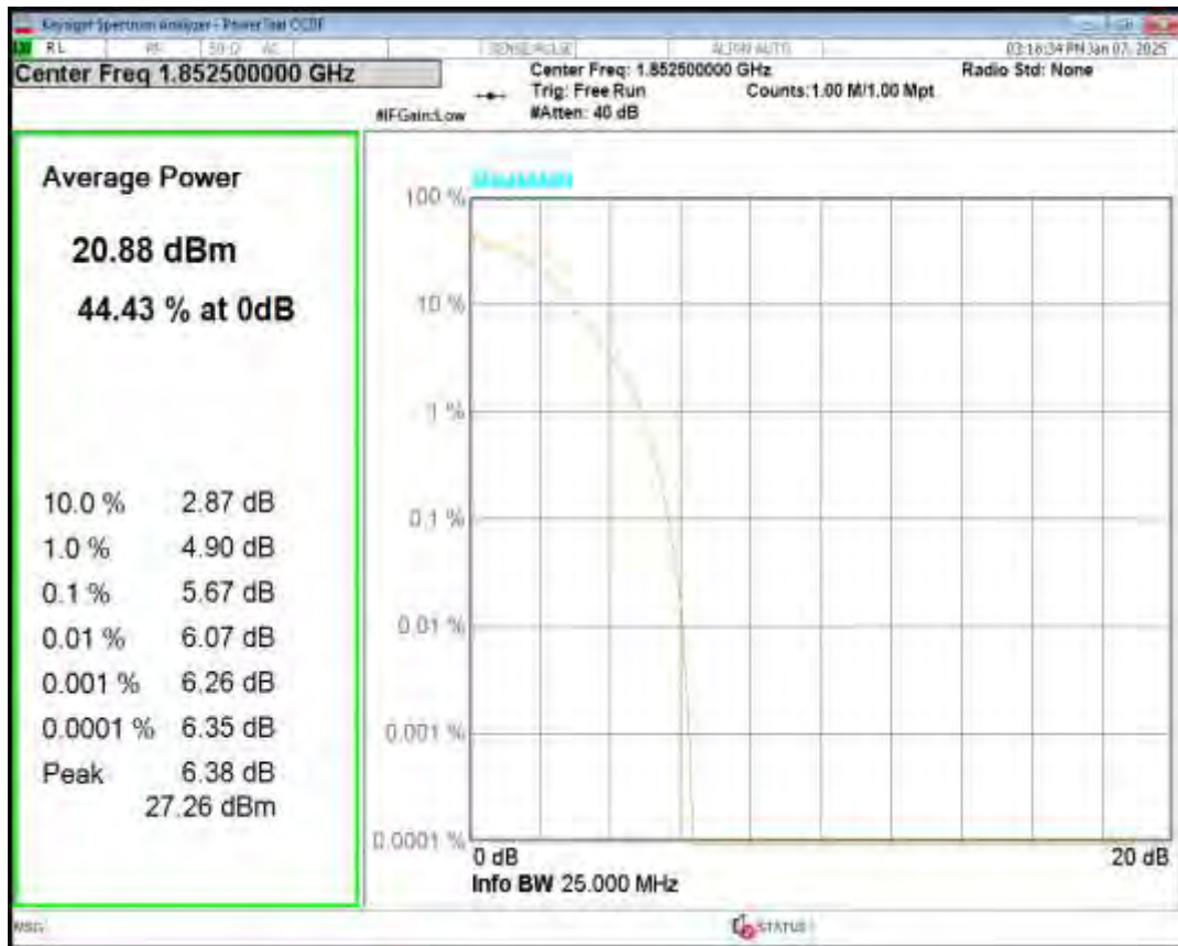
Band2 QPSK BW=1.4MHz Channel=18607 RB Size=1 Position=#0
