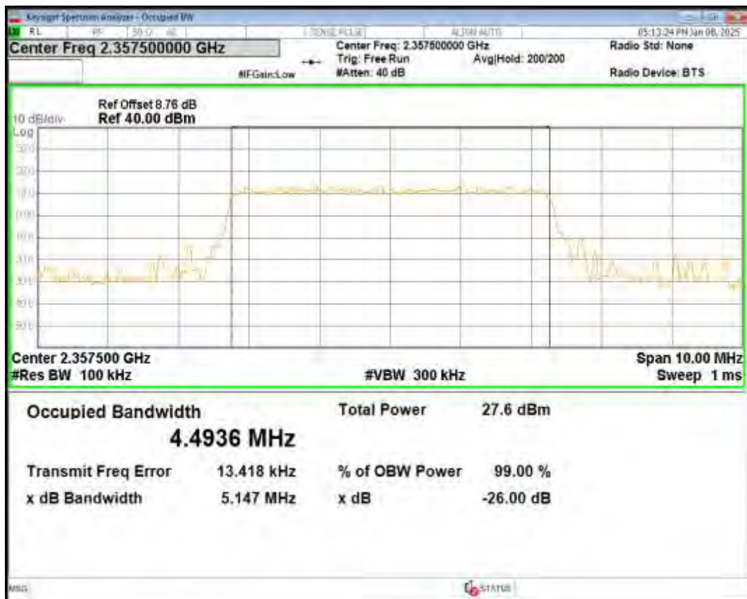
Band40(2350-2360) QPSK BW=10MHz Channel=39200 RB Size=50 Position=#0
