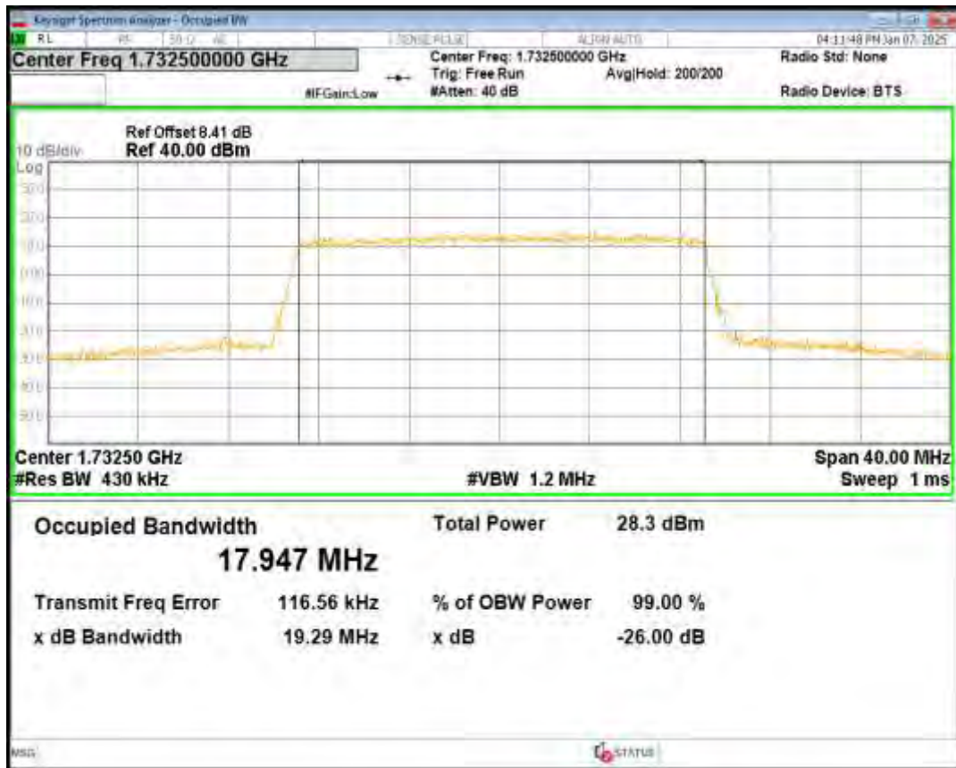
Band4 16QAM BW=20MHz Channel=20300 RB Size=100 Position=#0
