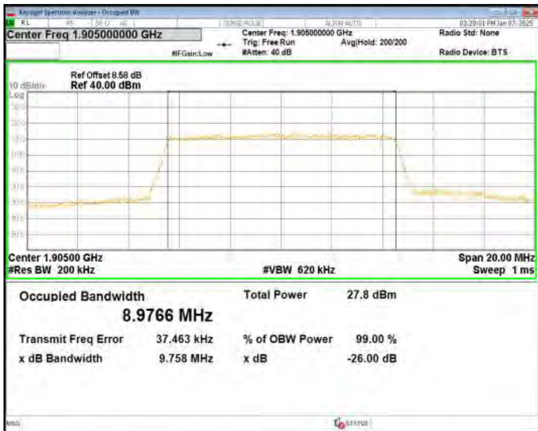
Band2 16QAM BW=15MHz Channel=18675 RB Size=75 Position=#0
