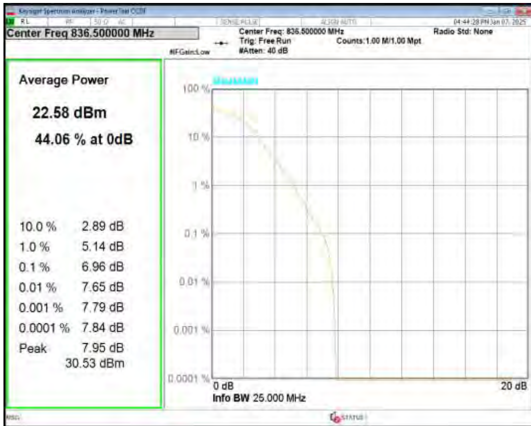
Band5 QPSK BW=1.4MHz Channel=20407 RB Size=1 Position=#0
