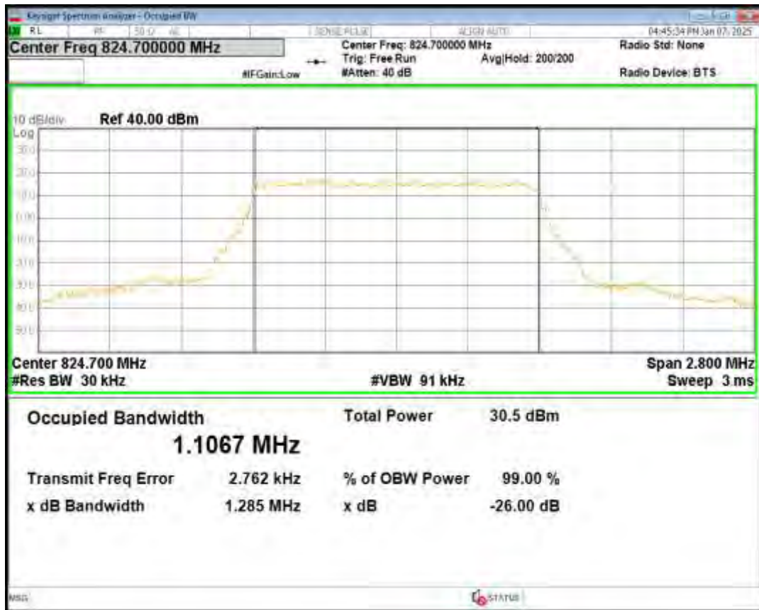
Band5 16QAM BW=5MHz Channel=20525 RB Size=25 Position=#0
