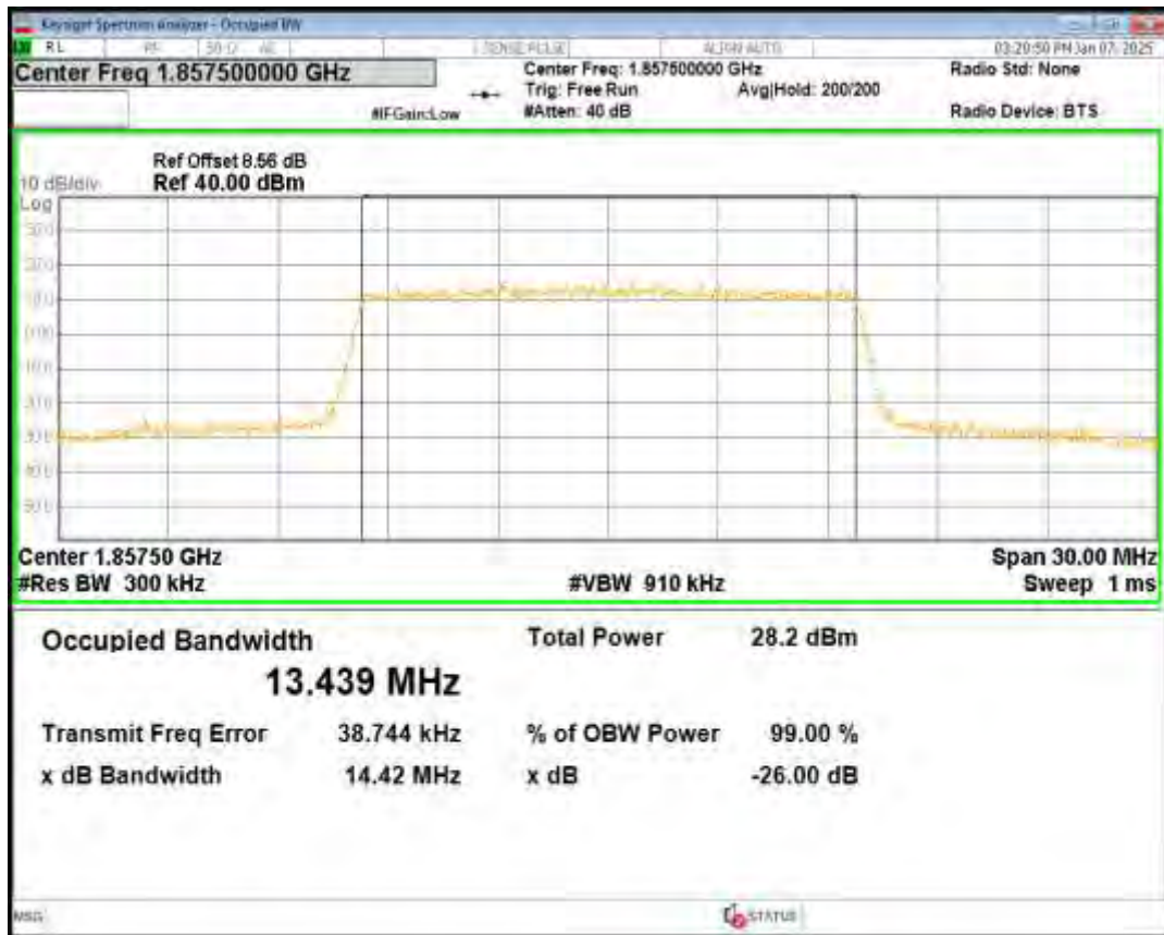
Band2 16QAM BW=15MHz Channel=18900 RB Size=75 Position=#0
