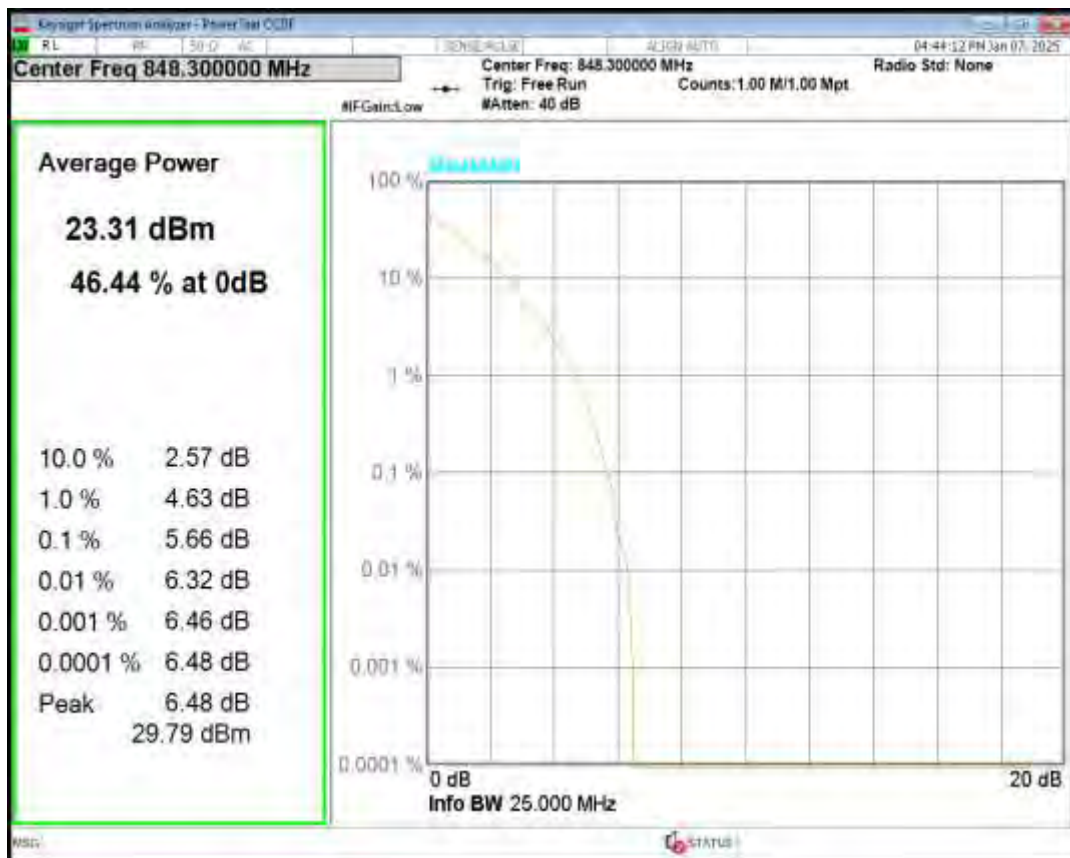
Band5 QPSK BW=10MHz Channel=20450 RB Size=1 Position=#0
