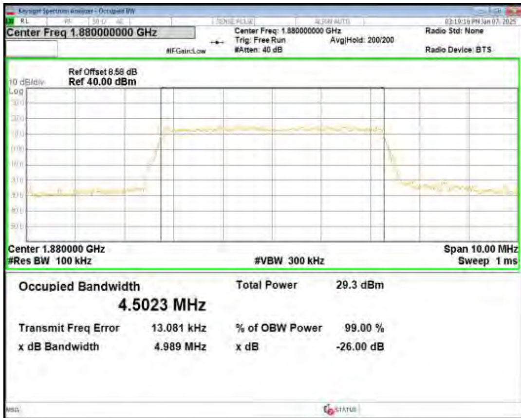
Band2 QPSK BW=5MHz Channel=19175 RB Size=25 Position=#0
