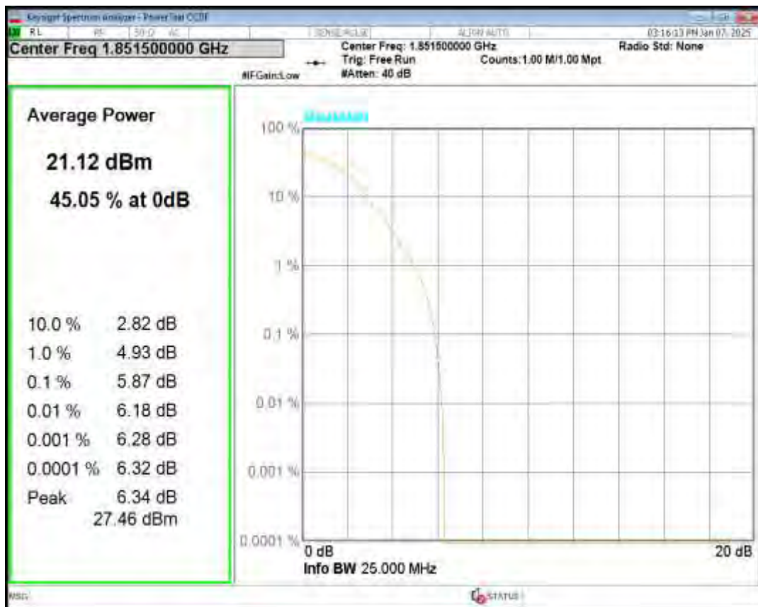
Band2 16QAM BW=20MHz Channel=19100 RB Size=1 Position=#0
