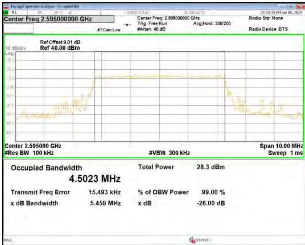
Band38 QPSK BW=5MHz Channel=38225 RB Size=25 Position=#0
