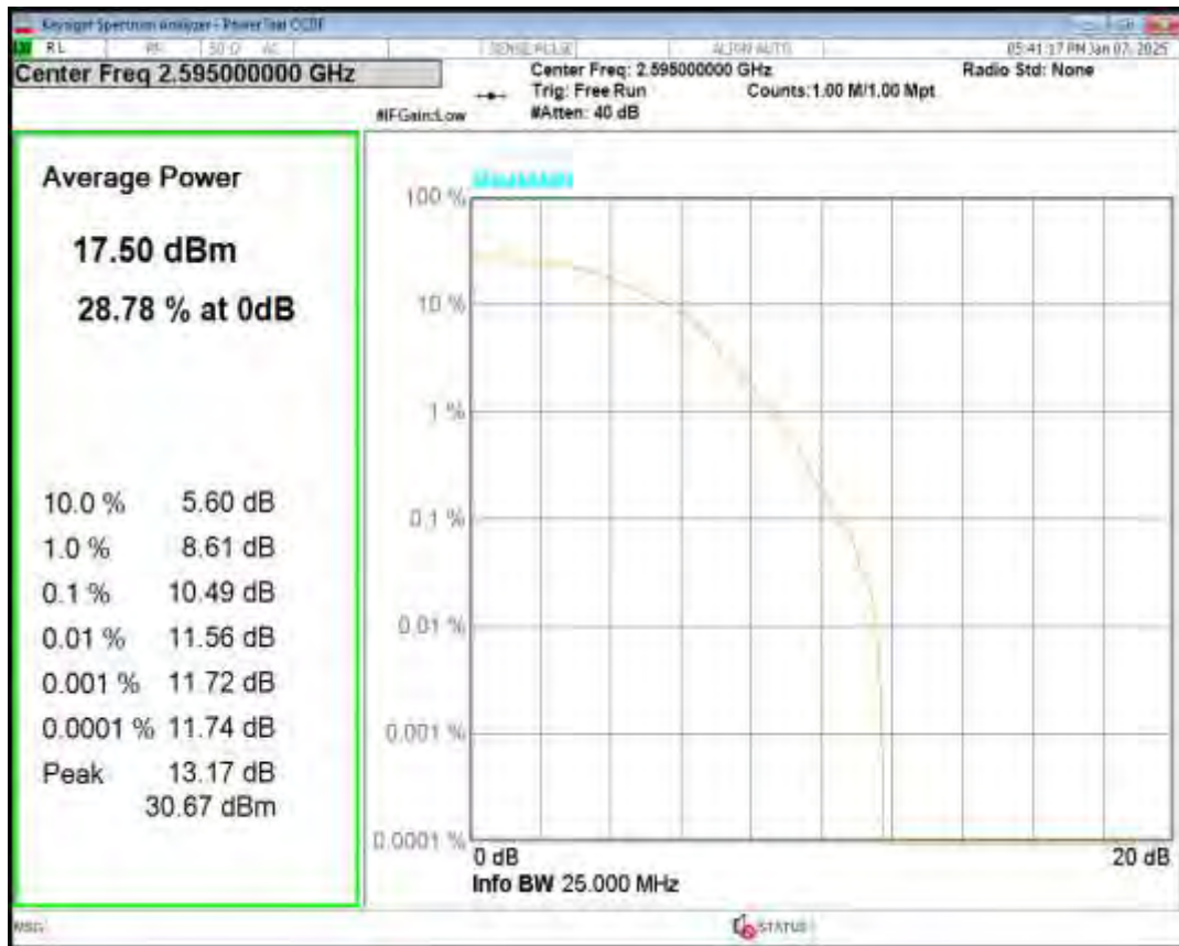
Band38 16QAM BW=10MHz Channel=38200 RB Size=1 Position=#0
