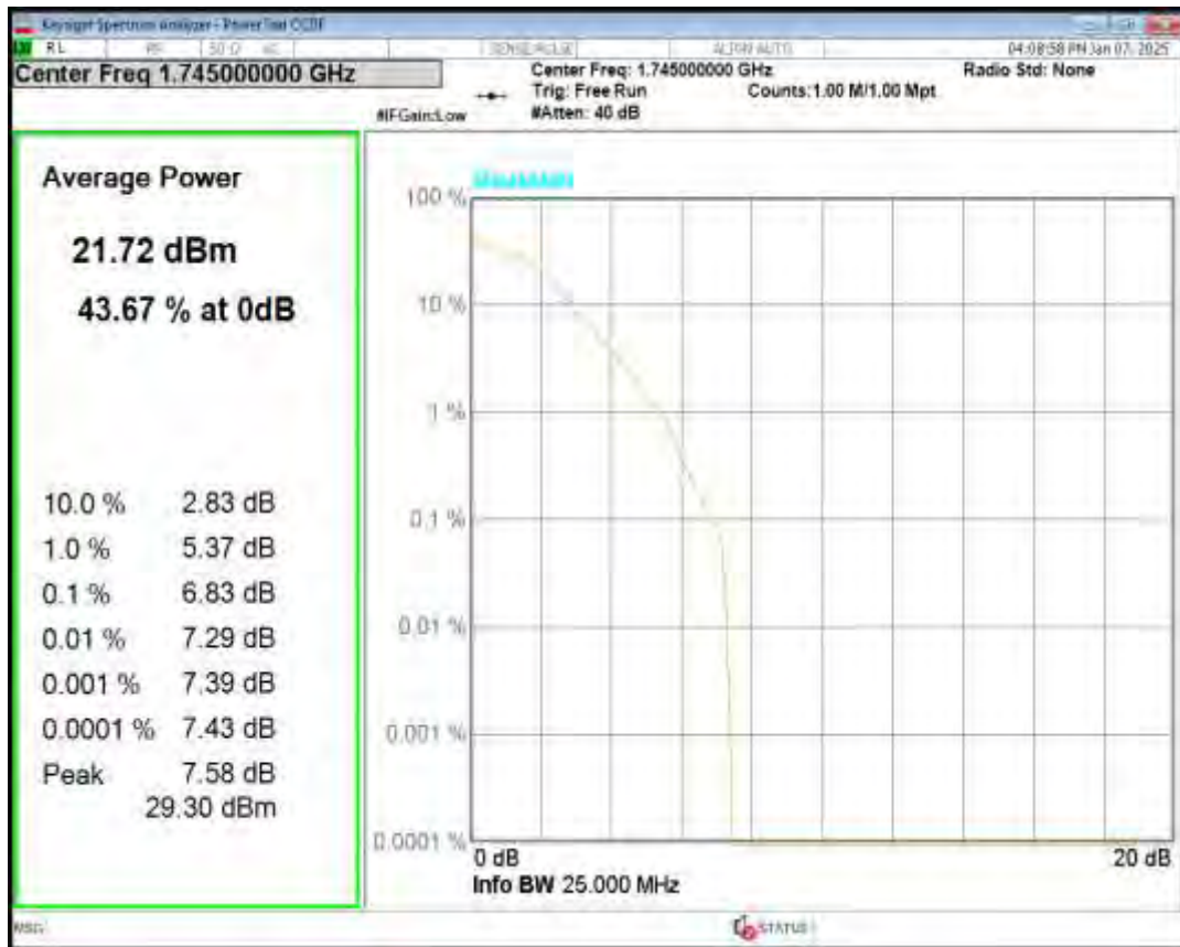
Band4 16QAM BW=3MHz Channel=19965 RB Size=1 Position=#0
