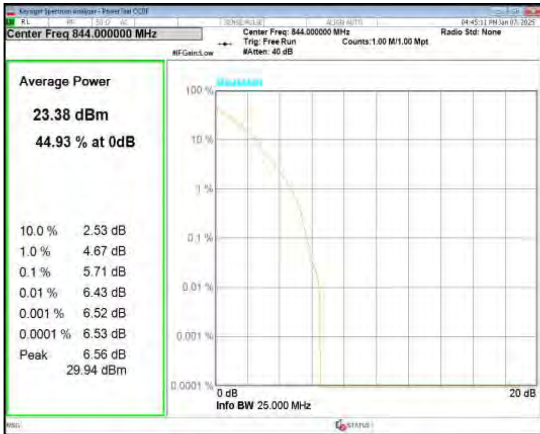
Band5 QPSK BW=3MHz Channel=20415 RB Size=1 Position=#0
