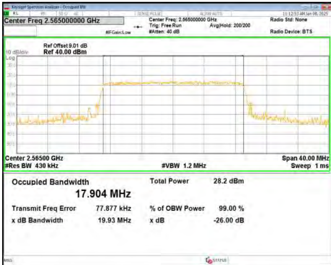
Band41(2555-2655) QPSK BW=20MHz Channel=40740 RB Size=100 Position=#0
