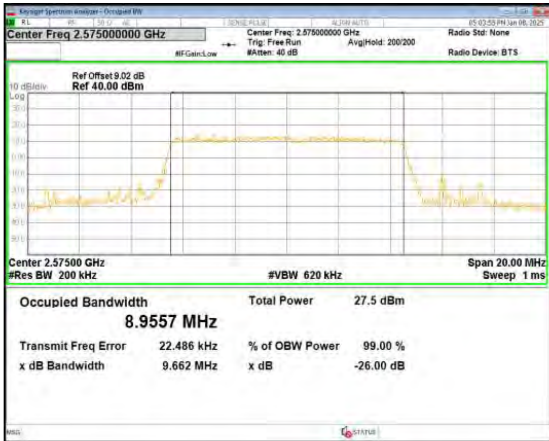
Band38 16QAM BW=10MHz Channel=38000 RB Size=50 Position=#0
