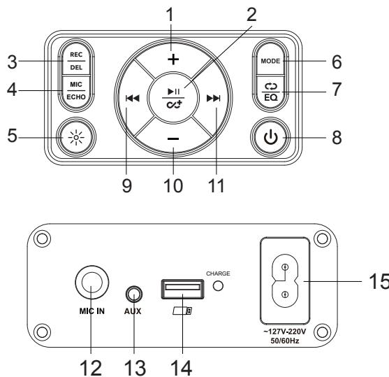
4. MIC/ECHO: Short press this button, the screen will display "N", and you can adjust the volume of the microphone at this time. Short press this button again, and the screen will display "E", at which point you can adjust the reverb volume.
