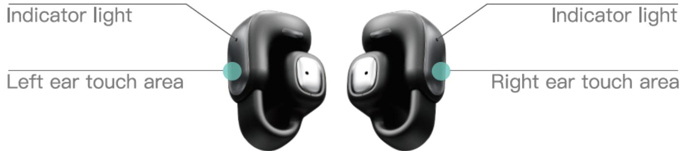
**Introduction to Indicator Lights:** When the left and right earphones are pairing during startup, the white lights on them will flash. When the pairing is successful, the white light on the master earphone will flash while the light on the slave earphone will go out. When the mobile phone's Bluetooth connection is successful, the lights on both the left and right earphones will go out simultaneously.
