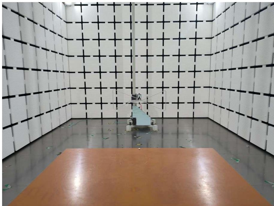
**Radiated Emission Test View Above 1GHz (left ear)**
