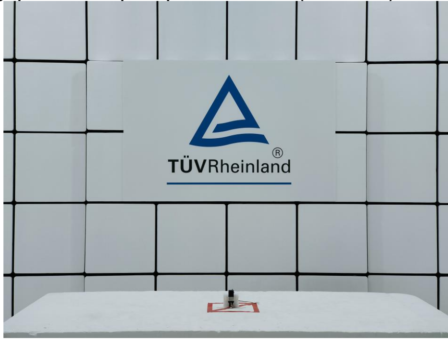
Photograph 2: Test Setup for Spurious Emissions (Front View 2)
