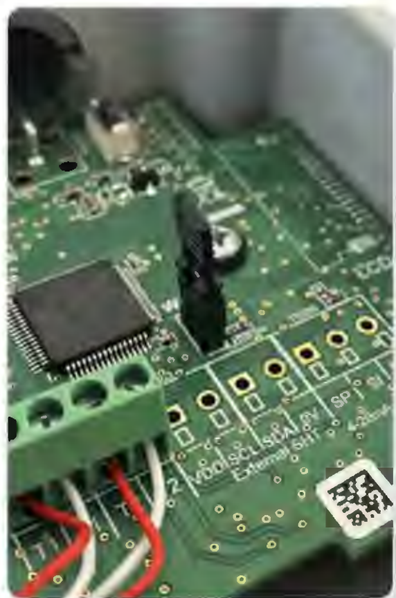
Proprietary LoRa mode Jumper positioned on both pins
