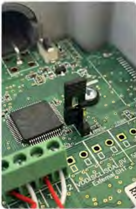
LoRaWAN Mode Jumper positioned on a single pin
