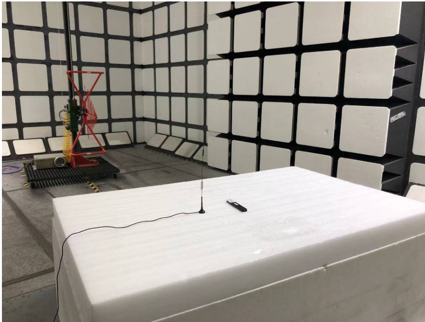
Radiated Emissions View (Below 1 GHz)
