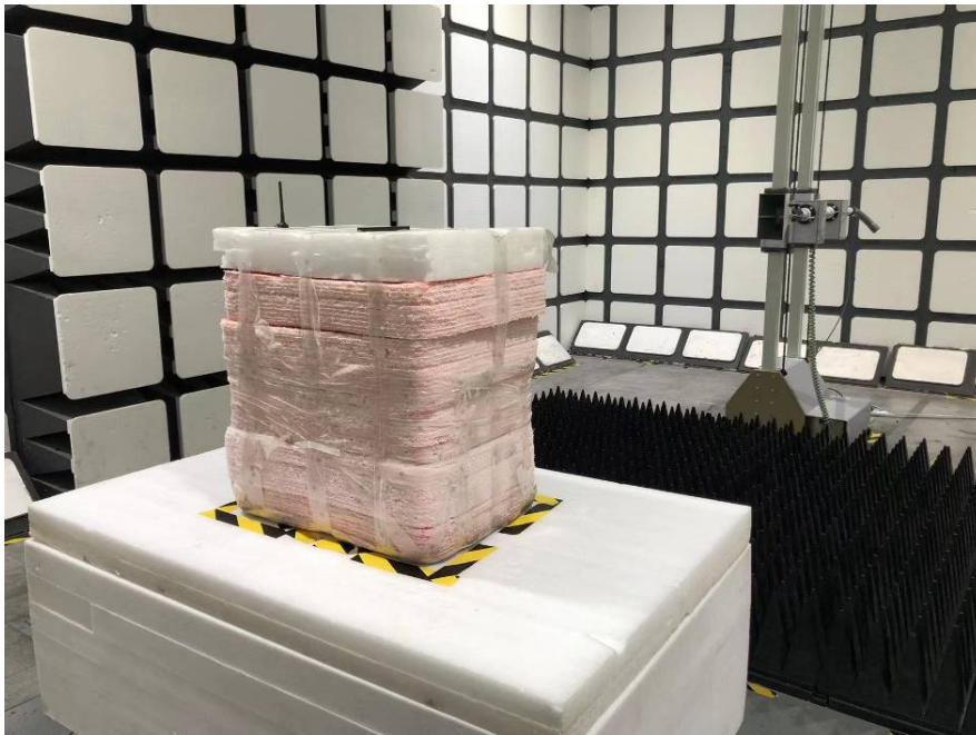
Radiated Emissions View (Above 1 GHz)
