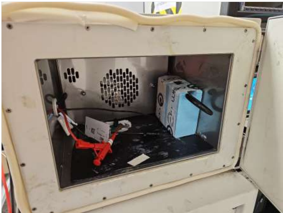
Photograph 5: EUT test setup in climatic chamber (EUT view)
