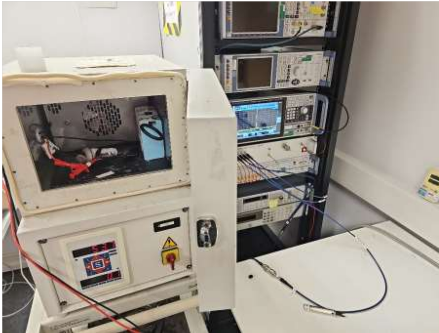
Photograph 4: EUT test setup in climatic chamber (overview)
