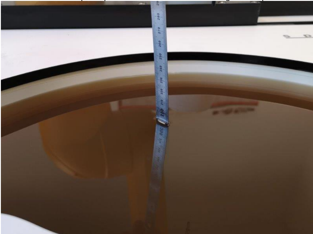
Photo 2: Liquid depth HBBL600-10000MHz Simulating Head Liquid
