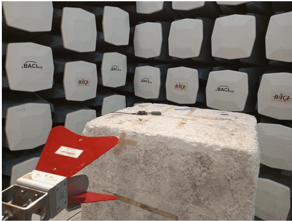
**1.6 Radiated Spurious Emissions measured at 1 meter, 1 GHz to 18 GHz, Rear View**
