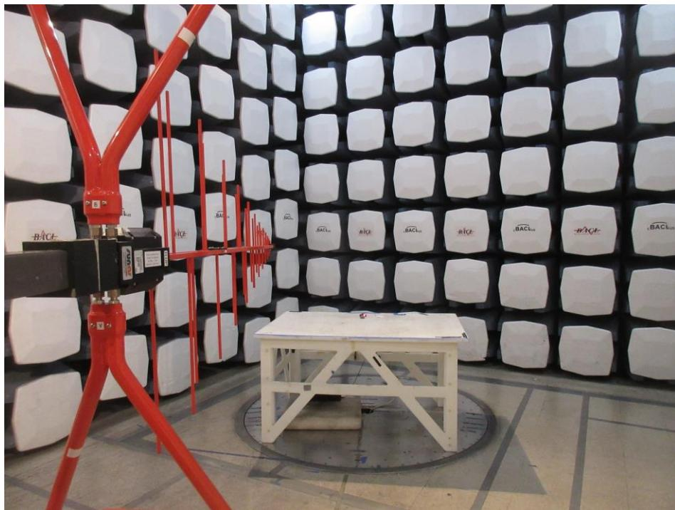
**1.4 Radiated Spurious Emissions measured at 3 meters, 30 MHz to 1000 MHz, Rear View**
