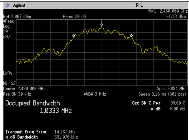
BLE_High Ch_2480MHz_1MBit_Occupied Bandwidth_99 percent
