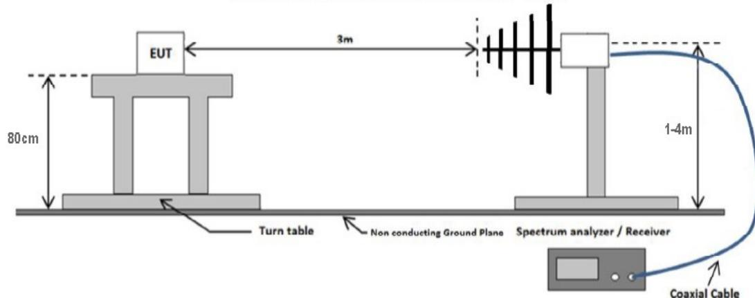
Radiated emissions test setup above 1 GHz
