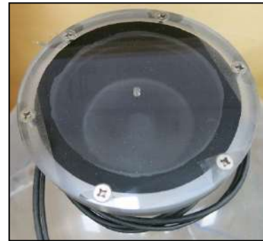
Figure 28.1 Examples of the fluid level of the stabilized platform and vertical accelerometer sensor: (a) fluid level sufficient, (b) fluid level too low
