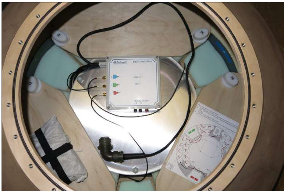
Figure 8.2 DWR4/ACM 0.9m - ACM electronics inside the hull control unit and coaxial cables of the three acoustic transducers.
