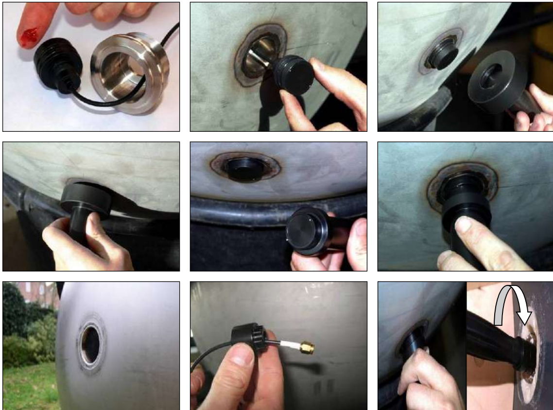
Figure 28.4 Procedure for installing an acoustic transducer. Pictures are labelled (a)-(i) first left to right, then top to bottom.
