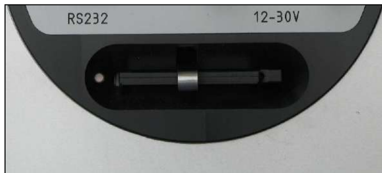
Figure 17.1 Logger flash card slot in the central block of the hatchcover electronics unit, with drive activity LED, metal clip and release button.
