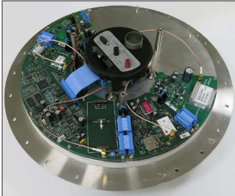
Figure 19.5 Overview of an electronics unit configuration with GSM and Iridium SBD
