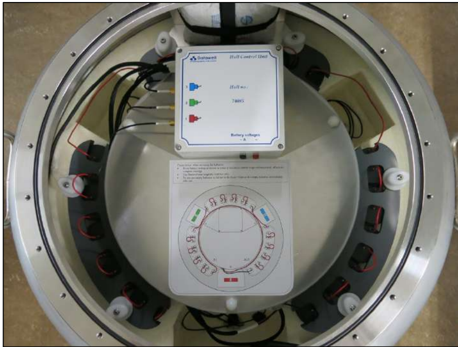
Figure 8.3 DWR4/ACM 0.7m - ACM electronics inside the hull control unit and coaxial cables of the three acoustic transducers.
