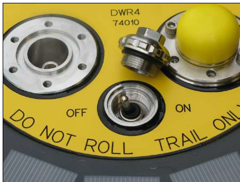
Figure 22.1 External power switch on the hatchcover, underneath the nut with sealing ring and ON and OFF labels on the sides.
