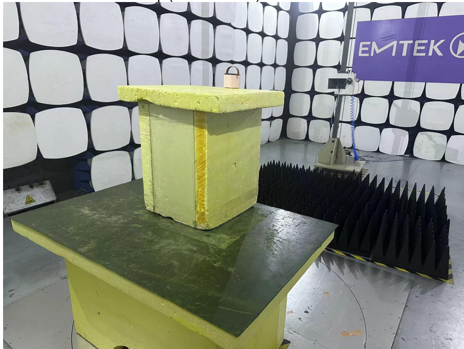
Spurious Emission Test Setup (30MHz-1GHz)
