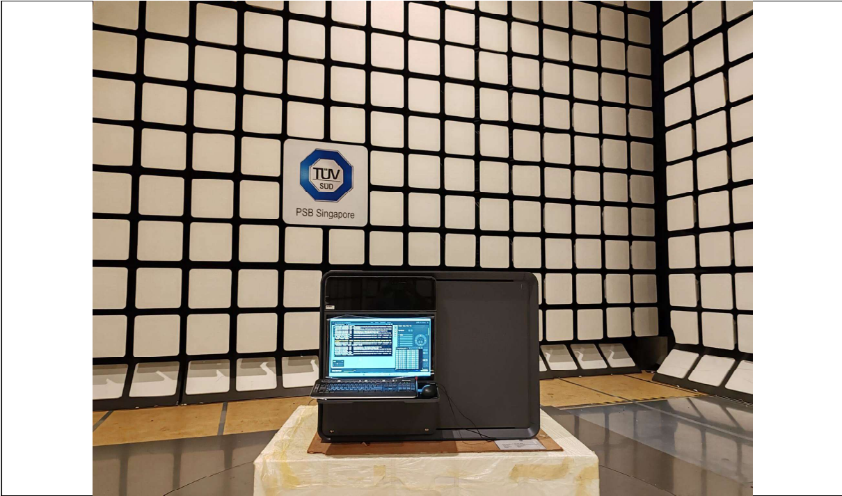
Radiated Emissions (Fundamental) Test Setup (Front View)
