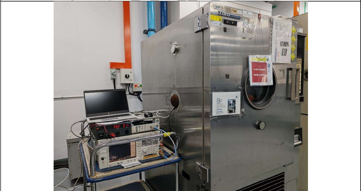
Frequency Stability Versus Input Voltage Test Setup
