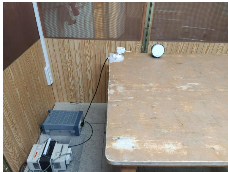
Photograph 7.6.1 Setup for conducted emission measurements
