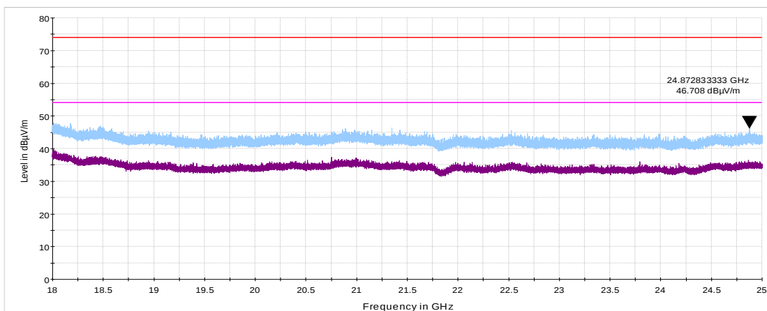
Plot 7.3.19 Radiated emission measurements from 18 to 25 GHz at the mid carrier frequency
