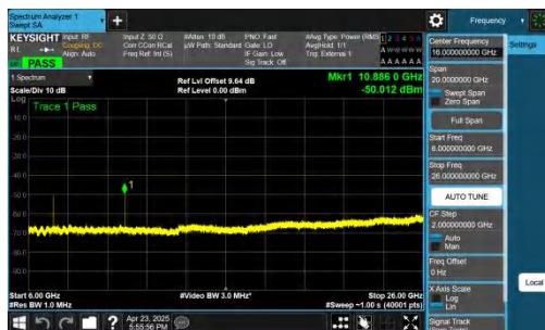
NTNV-n48-PC3-30-10-M-CP-QPSK-Inner_1RB_Right-6000-2600 0-PASS
