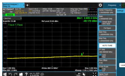
NTNV-DC_2A-n78A(3700-3800)-PC2-30-5+50-M+L-QPSK-IDLE-D FT-QPSK-Inner 1RB Left-1000-3000-PASS
