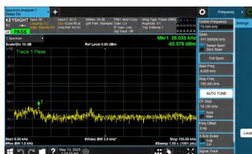
NTNV-DC_2A-n78A(3450-3550)-PC2-30-5+80-M+H-QPSK-IDLE-D FT-QPSK-Inner 1RB Right-0.009-0.15-PASS
