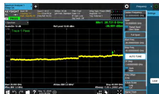
NTNV-DC_2A-n77A(3700-3980)-PC2-30-5+40-M+M-QPSK-IDLE-D FT-QPSK-Inner 1RB Right-26000-40000-PASS
