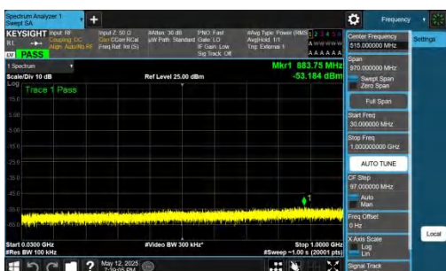
NTNV-DC_2A-n77A(3700-3980)-PC2-30-5+20-M+L-QPSK-IDLE-D FT-BPSK-Inner 1RB Left-30-1000-PASS
