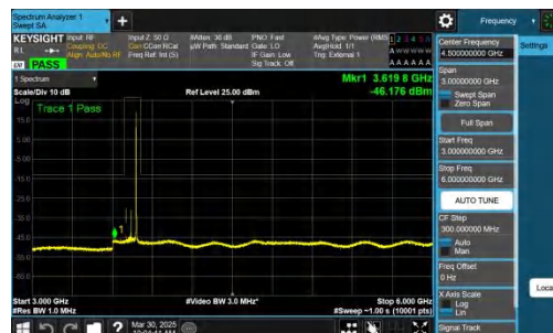
NTNV-n78(3700-3800)-PC2-30-80-L-CP-QPSK-Inner_1RB_Right-3000-6000-PASS
