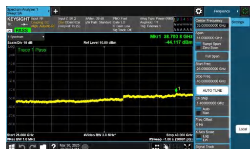
NTNV-n78(3700-3800)-PC2-30-80-H-CP-QPSK-Inner_1RB_Right- 26000-40000-PASS
