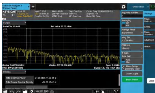
NTNV-n41-PC2-30-90-H-DFT-QPSK-Edge 1RB Right-PASS
