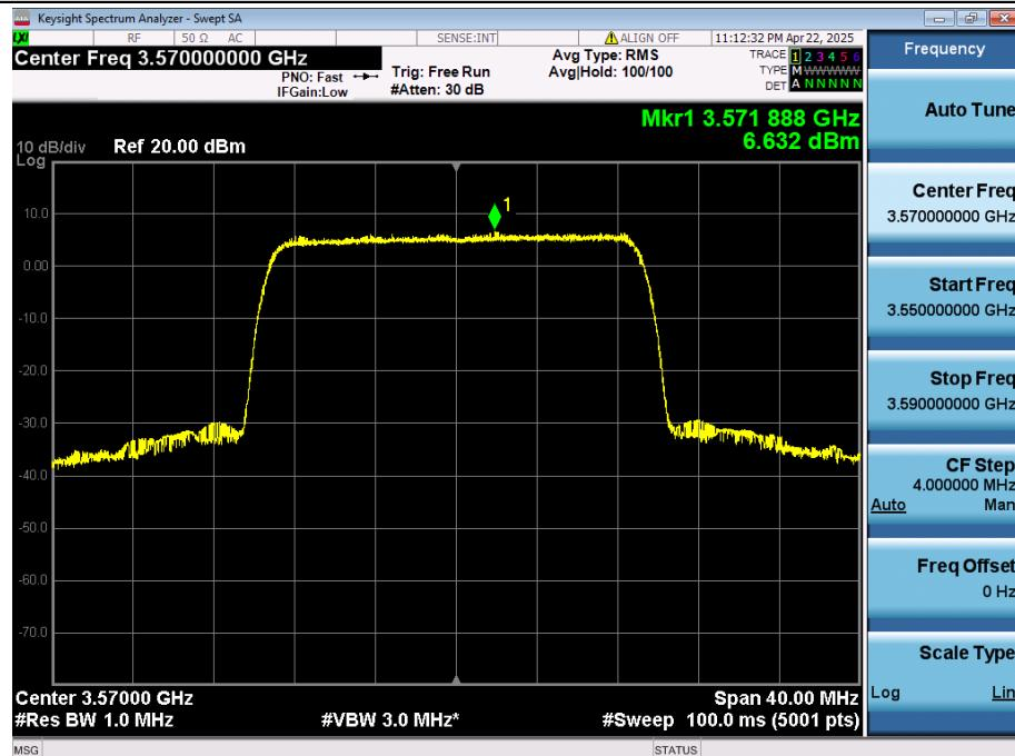
EIRP PSD=6.632-1.36+4.5=9.772dBm/MHz, Antenna gain is -1.36dBi, the path loss is 4.5dB
