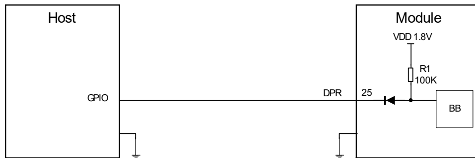
Figure 19: DPR Signal Reference Circuit Design
