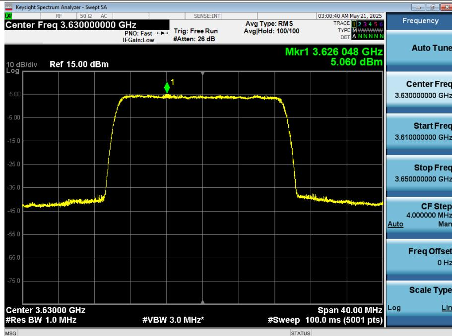
EIRP PSD=5.060-4.29+4.5+3=8.27dBm/MHz, Antenna gain is -4.29dBi, the path loss is 4.5dB, the MIMO Factor is 3dB
