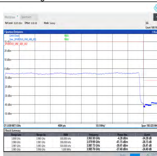
1-N77-3700-3980-30-90-H-3-DFT-PI2BPSK-Outer _Full-240@0-Ant0-1--PASS-see graph
