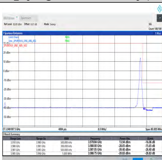
1-N77-3700-3980-30-70-H-5-CP-QPSK-Edge_1RB_Ri ght-1@188-Ant0-1--PASS-see graph
