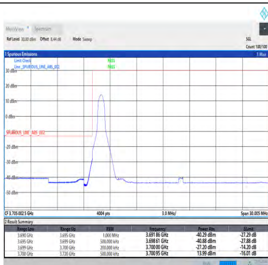
1-N77-3700-3980-30-20-L-1-DFT-PI2BPSK-Edge_1RB _Left-1@0-Ant0-1--PASS-see graph
