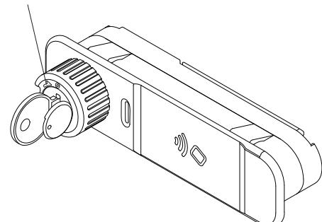
After opening, remember to turn it back to the locked position and pull it out (indicator window will be red)
