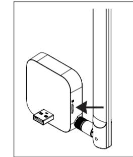
2. When the gateway is powered off, insert the 4G assistant into the USB card holder marked with 4G on the gateway. Make sure to insert it effectively.
