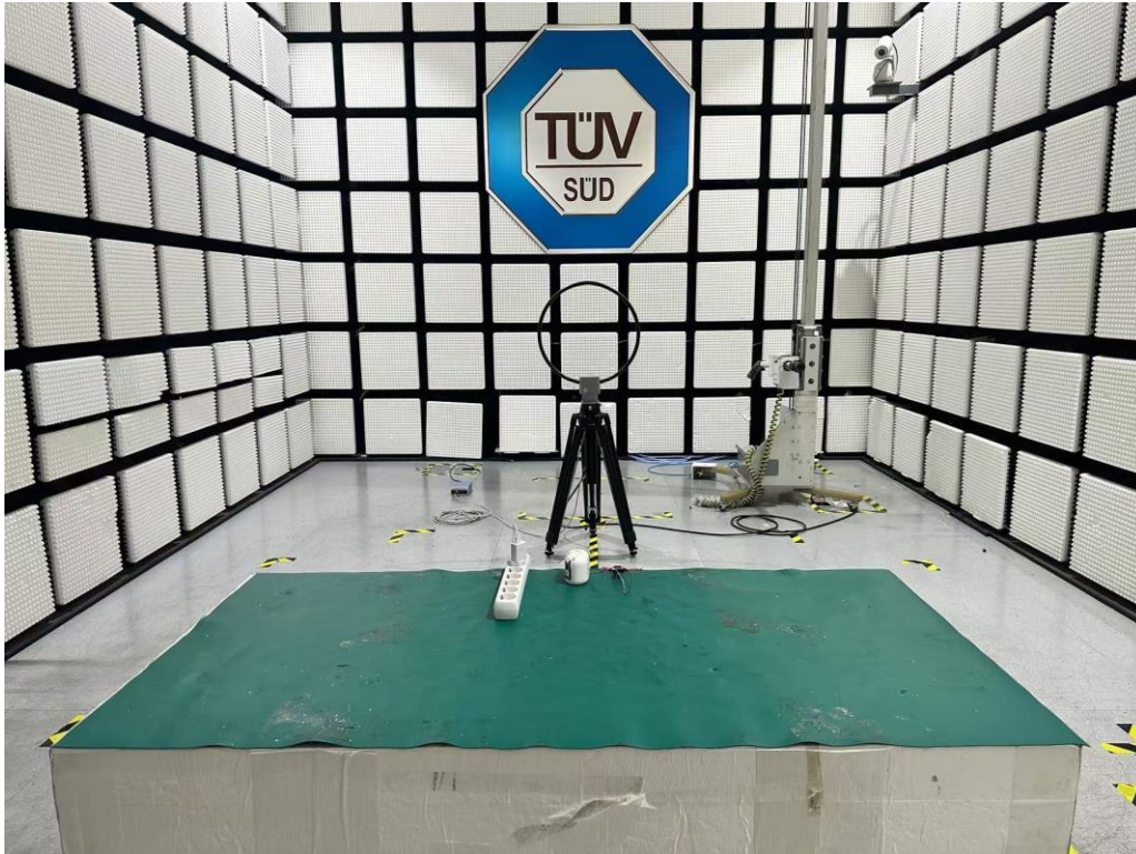
Radiated Emission Setup 9KHz-30MHz
