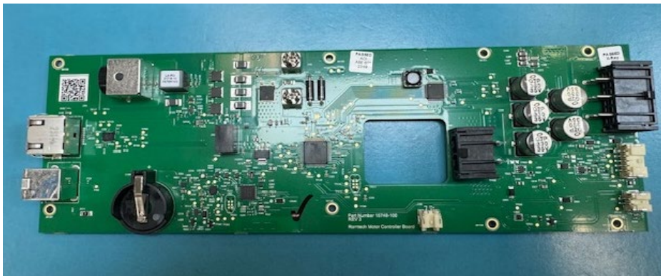
Figure 10; Topside Motor controller Board 15749-200 Rev 7
