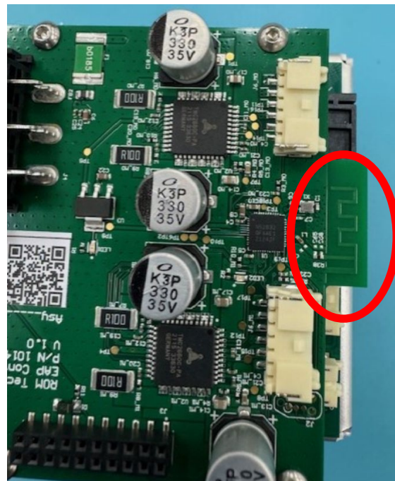
Figure 18; Trace antennae 10145-200 Rev 2 for Bluetooth
