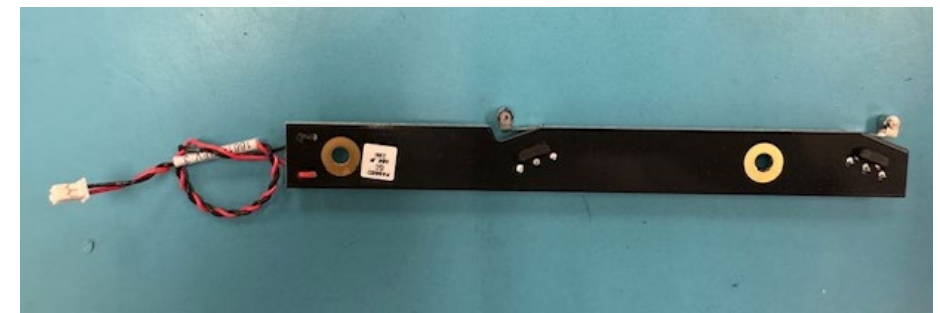
Figure 17; Bottom Side Accuradius Zippy PCA ,16614-200 Rev 4
