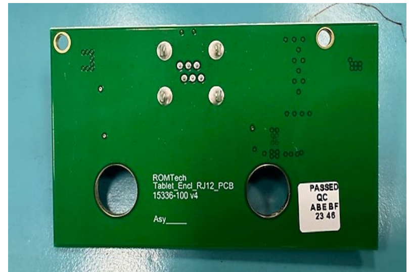
Figure 15; Bottom side Tablet Enclosure RJ12 PCA, 15336-200 Rev 4
