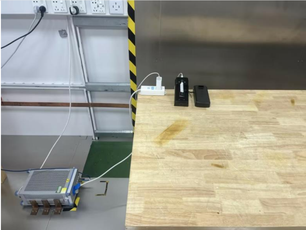
AC Power Line Conducted Emission
